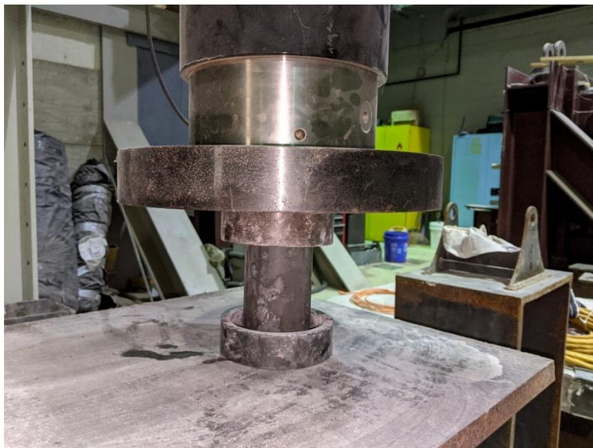
**Figure 4-1:** UHPC compression test setup.
