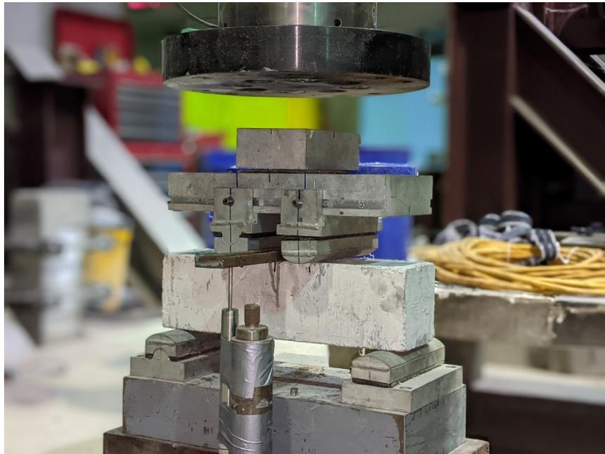
**Figure 4-3:** Flexural test setup of a UHPC beam.
