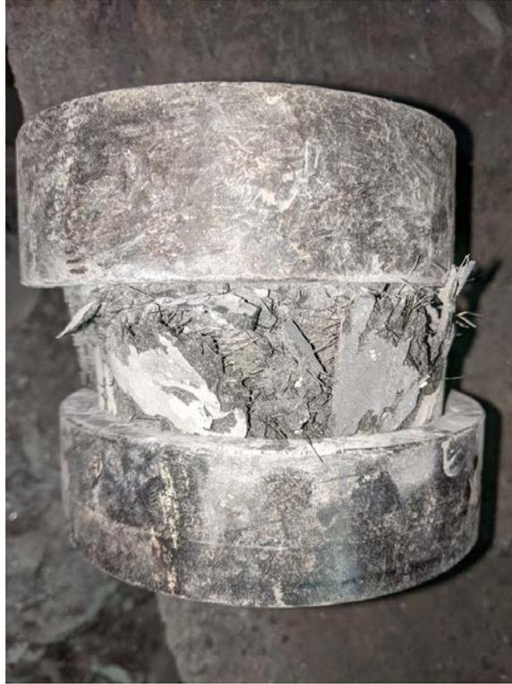
**Figure 4-2:** UHPC cylinder sample after testing.
