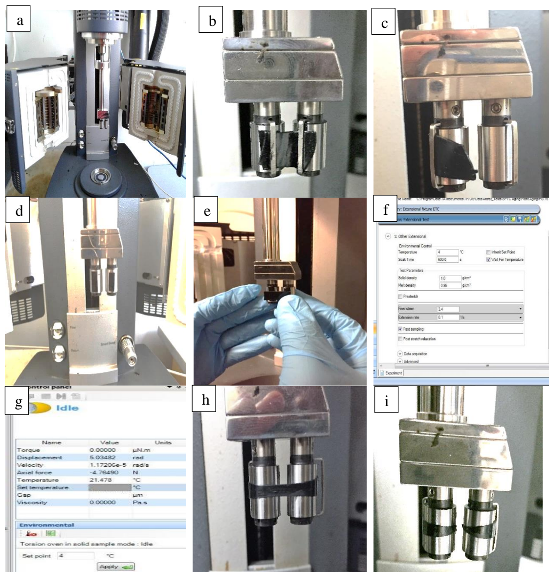
Figure 2-3: (a) The SER fixture before loading the specimen, (b) SER fixture after loading the specimen, (c) Clamps kicked out due to the high stresses, (d) Double-sided adhesion tape fixed to the drums, (e) Loading the sample post to the double-side adhesion tape, (f) Software screenshot shows the test Parameter, (g) Software screenshot shows the DSR control panel, (h) Sample during the extensional deformation test, (i) Sample after the end of the test.
