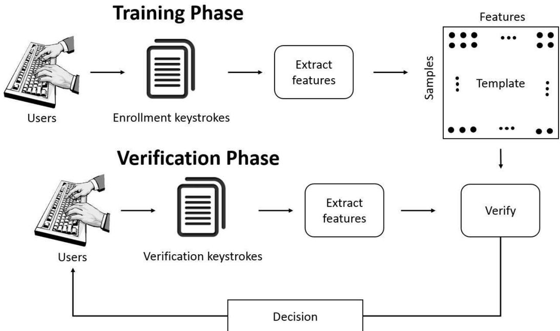
Figure 1.2: Overview of keystroke verification system on fixed text. In the training phase, keystroke features are extracted and a template (which is a matrix of order  $ab$ ) is created for each user from  $a$  features collected during  $b$  typing attempts. In the verification phase, features extracted from a keystroke sample is compared with the template to produce a verification decision.
