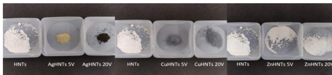
**Figure 5-2:** The natural white color of the HNTs was altered to darker colors depending on the type of metal used and quantity adsorbed.
