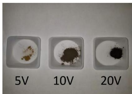
**Figure 4-3:** mHNTs produced at 5, 10, 20 V respectively, increasing applied voltage led to darker colored mHNTs, which can be attributed to the quantity of metal oxide adsorbed on HNTs.
