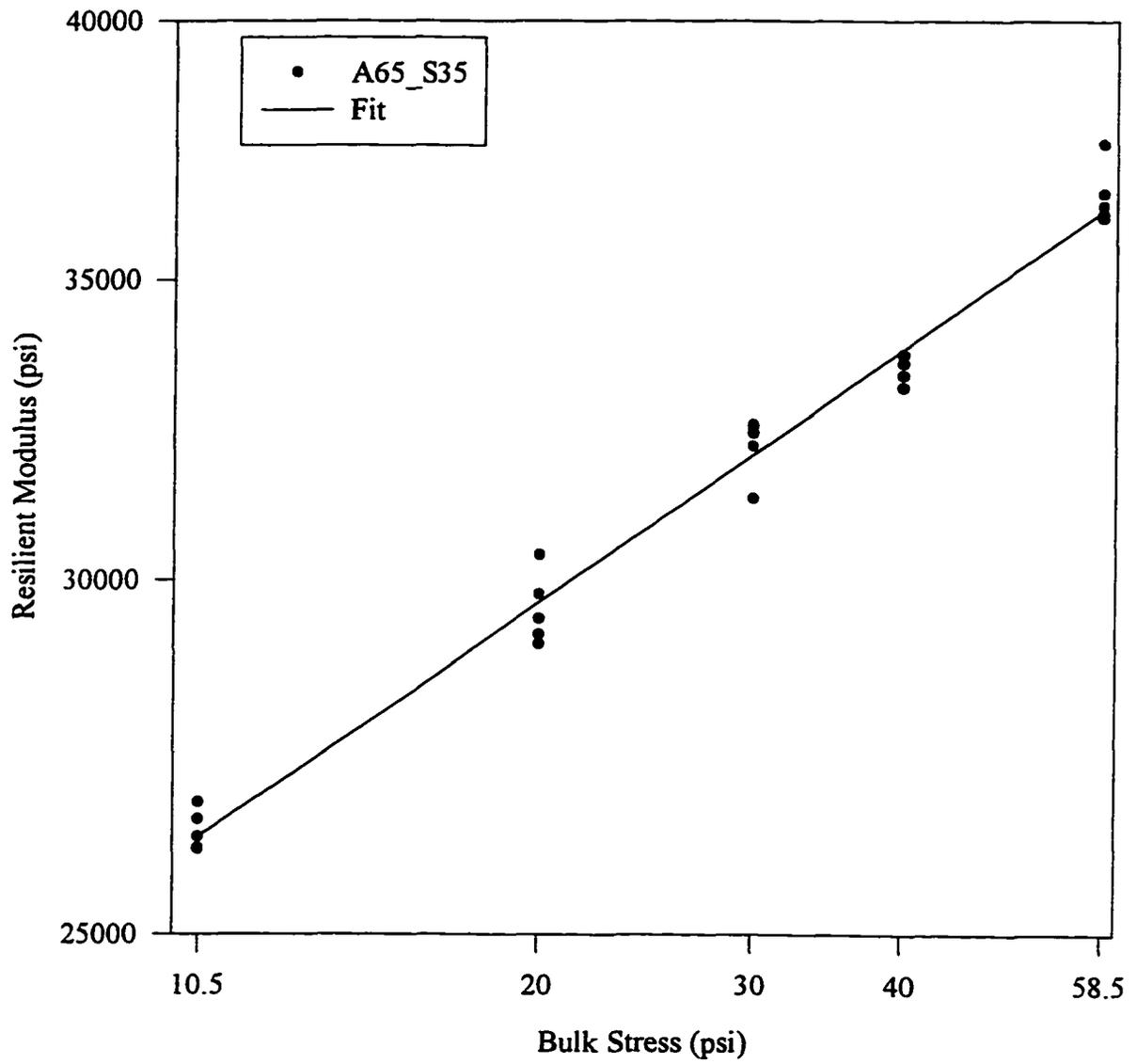
**Figure 5.5 Resilient Modulus vs. Bulk Stress: A65\_S35**
