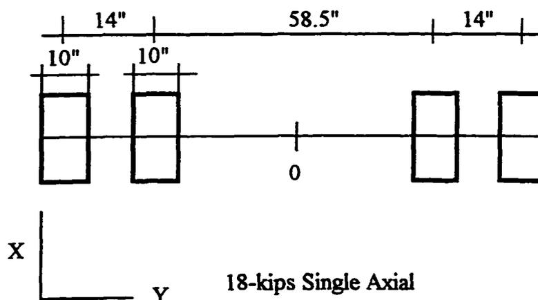
Figure 3.3 Load Configuration Used in Analysis
