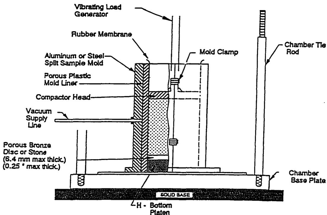
**Figure 4.6 Apparatus for Vibratory Compaction of Unbound Materials [39]**
