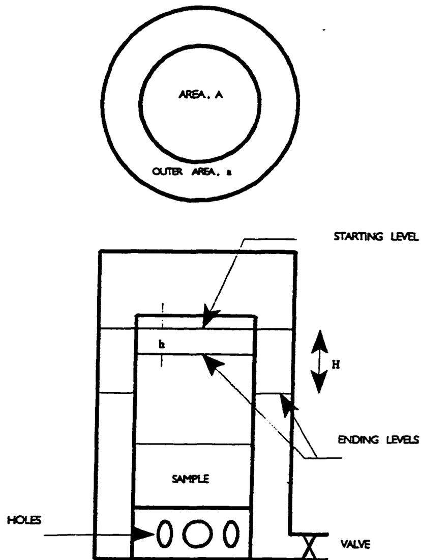
**Figure 4.1 Sketch of a Barber and Sawyer Permeameter**
