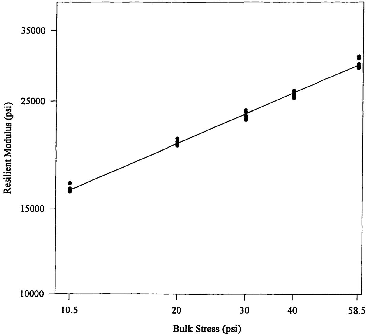
**Figure 5.3 Resilient Modulus vs. Bulk Stress: A85\_S15**
