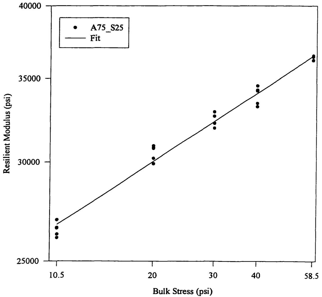
**Figure 5.4 Resilient Modulus vs. Bulk Stress: A75\_S25**
