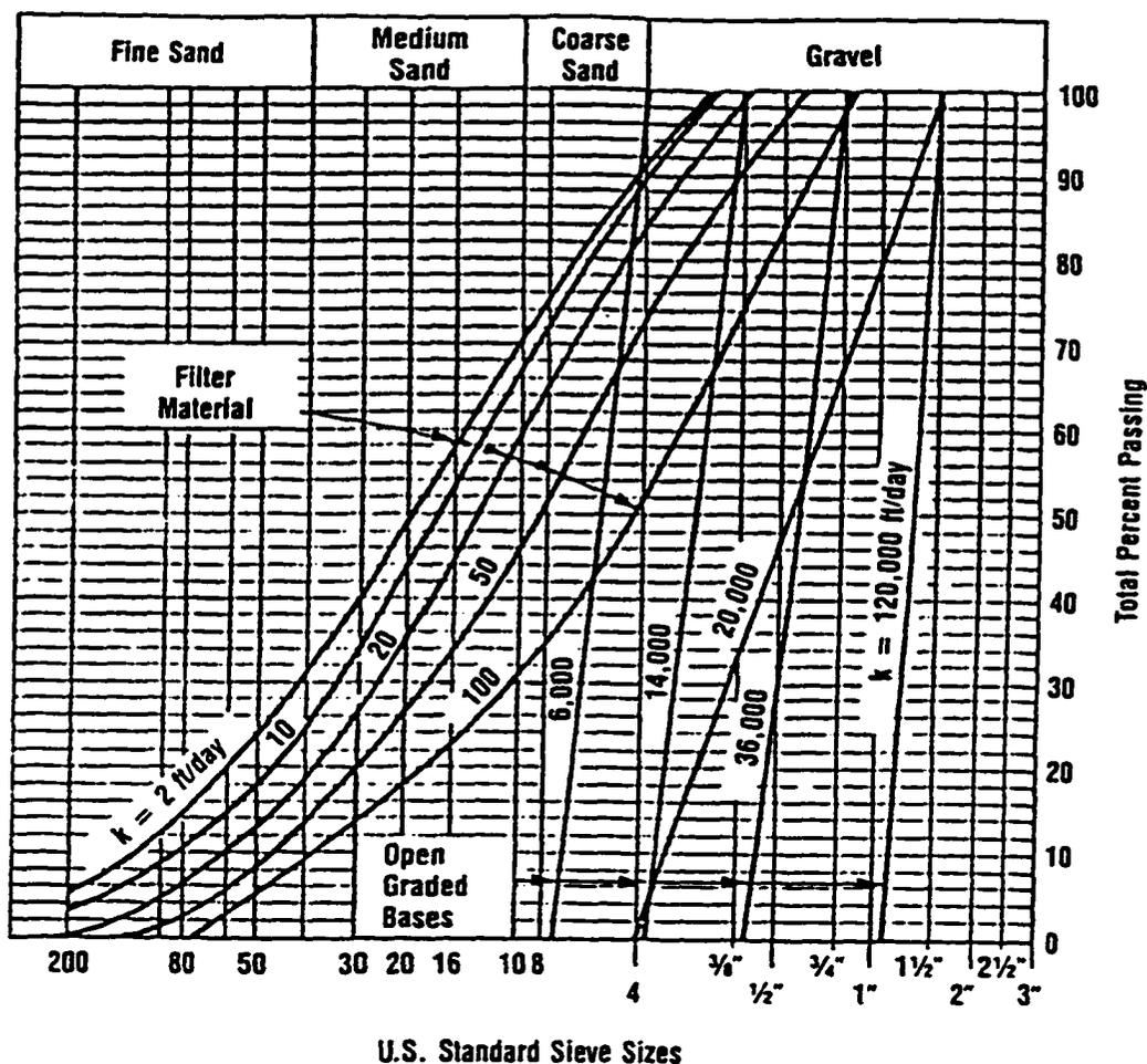
**Figure 2.4 Typical Gradation and Coefficients of Permeability of Open-Graded Bases and Filter Materials [33]**
