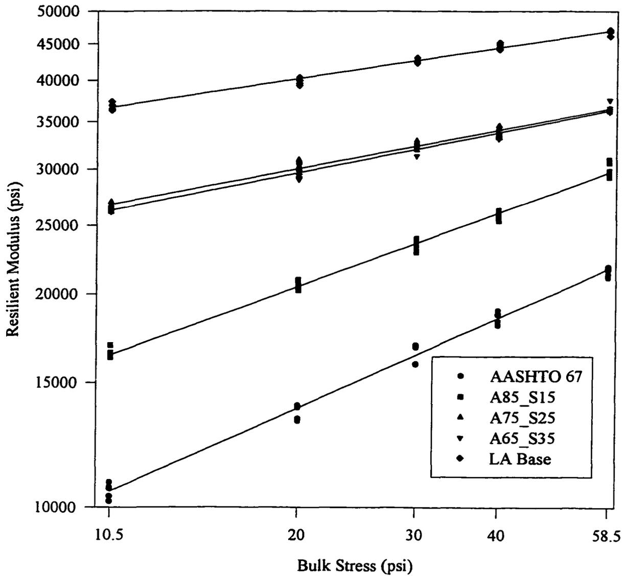
**Figure 5.7 Resilient Modulus vs. Bulk Stress: All Gradations**
