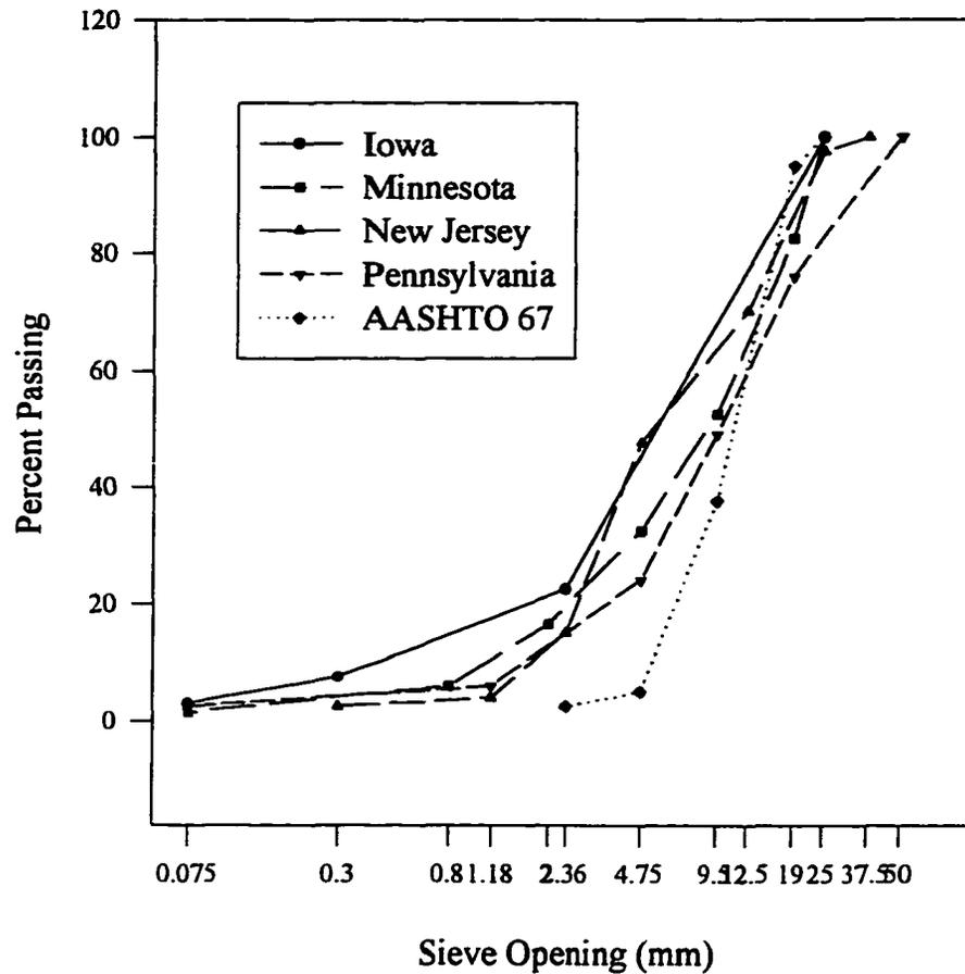
**Figure 2.2 Some SHAs Open-Graded Permeable Bases [11]**
