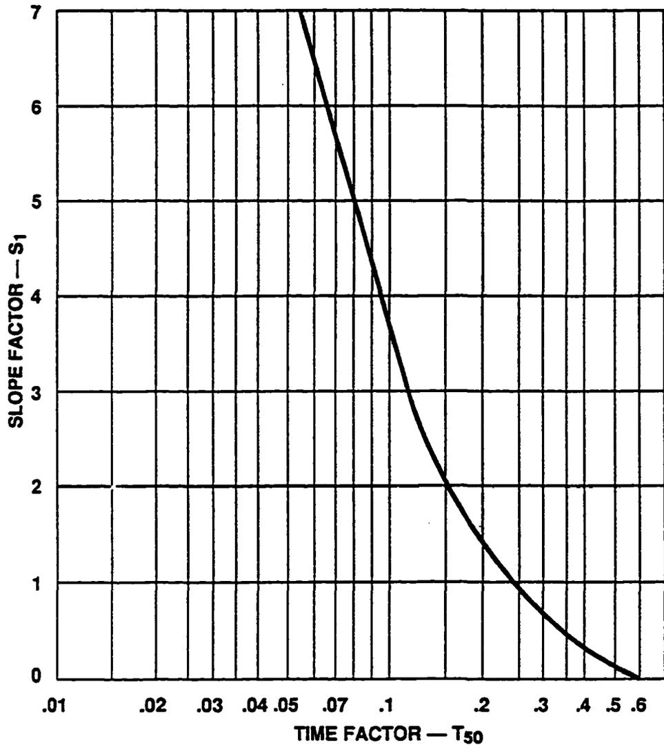
**Figure 6.4 Time Factor for 50 Percent Drainage [11]**
