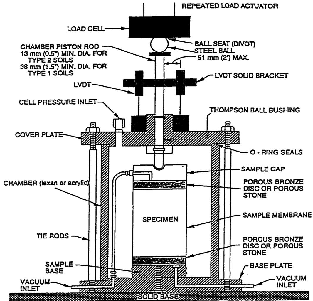
**Figure 4.5 Triaxial Chamber with External Mounted LVDTs and Load Cell [39]**
