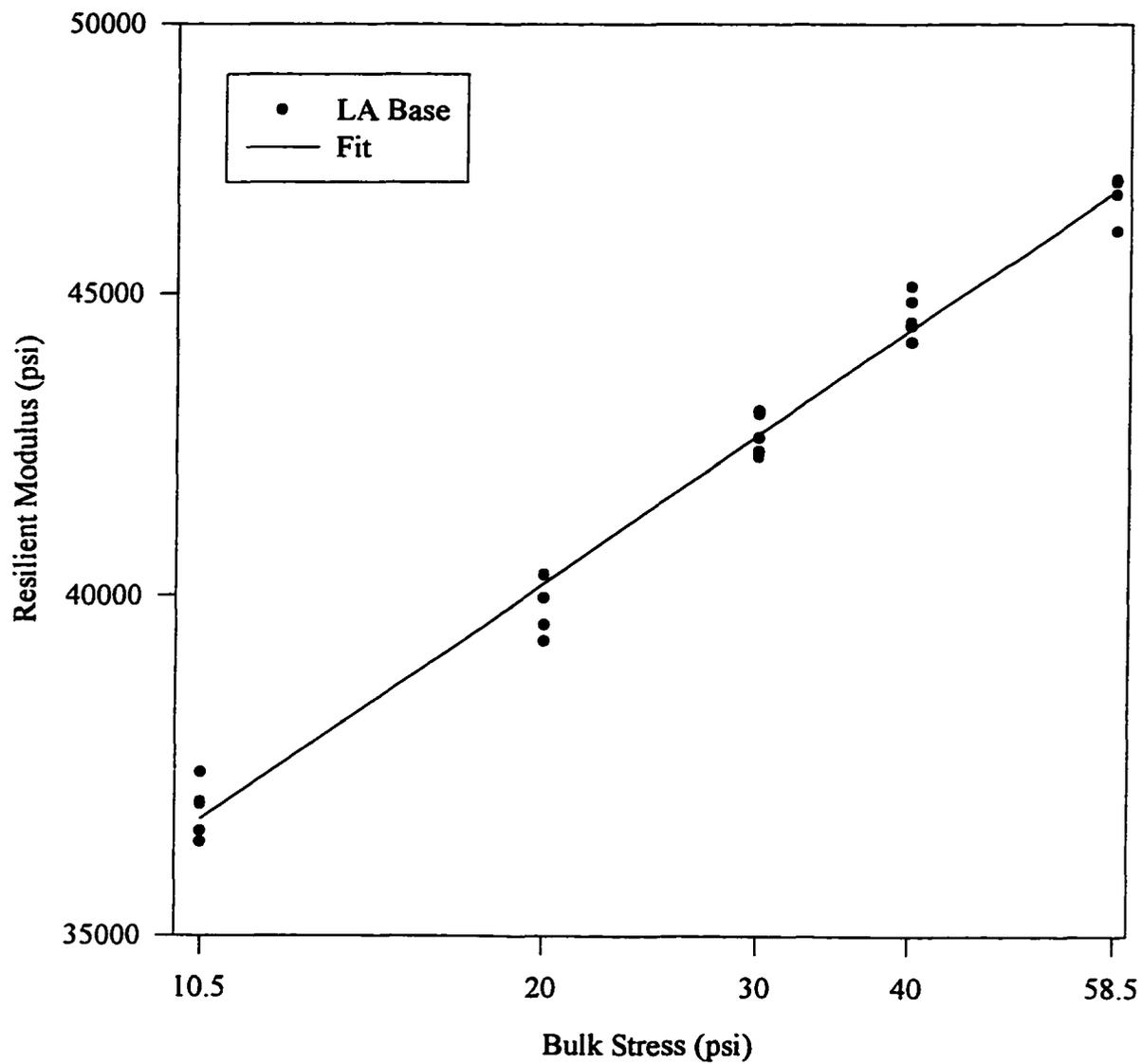
**Figure 5.6 Resilient Modulus vs. Bulk Stress: LA Typical Base**
