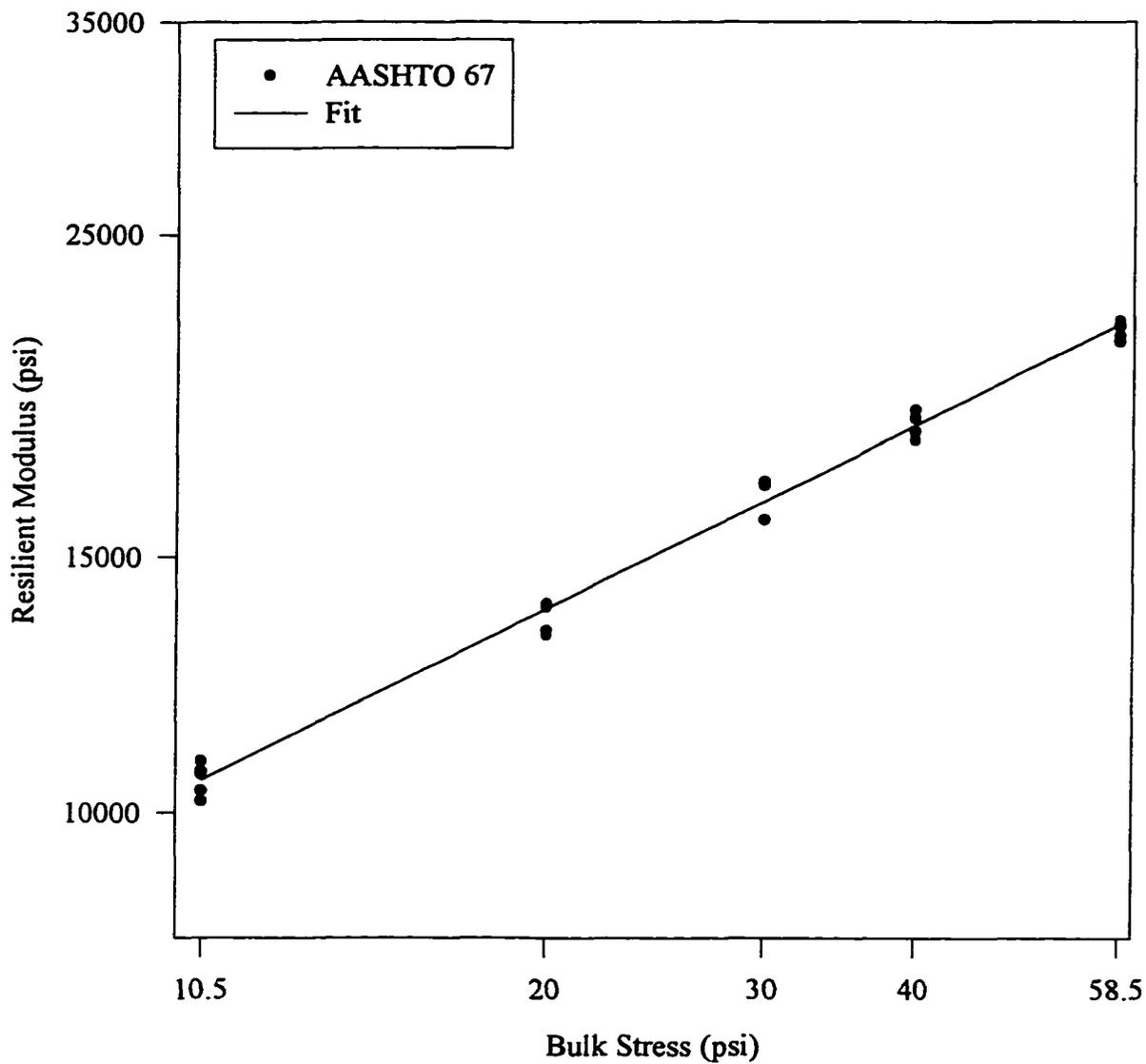
**Figure 5.2 Resilient Modulus vs. Bulk Stress: AASHTO 67**
