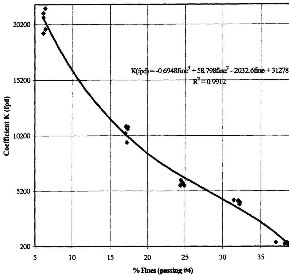
**Figure 5.1 Coefficient of Permeability vs. % Passing #4**
