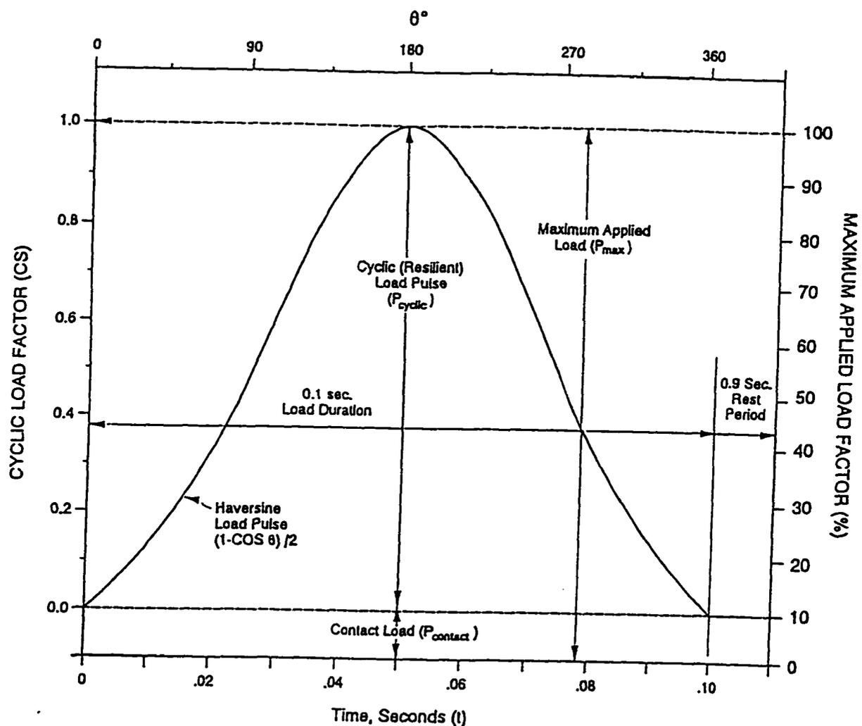
**Figure 4.4 Haversine Load Pulse [39]**
