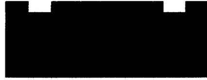
**d. Expose and develop to make vias pattern on the photoresist.**
