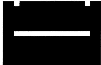
**j. Expose and develop to make backside via on photoresist.**
