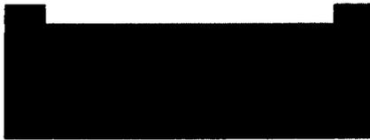
**e. Expose and develop to make channel pattern on the photoresist.**
