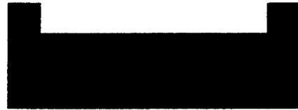
**f. ICP etching to transfer pattern from photoresist to silicon wafer.**
