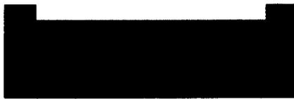
**g. Remove photoresist and clean the wafer.**
