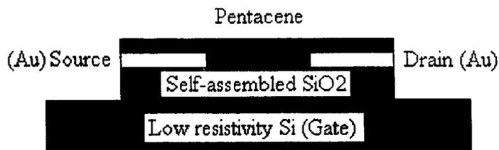
Figure 5-17 Schematic structure of Pentacene FET with SA- $\text{SiO}_2$  as gate dielectric
