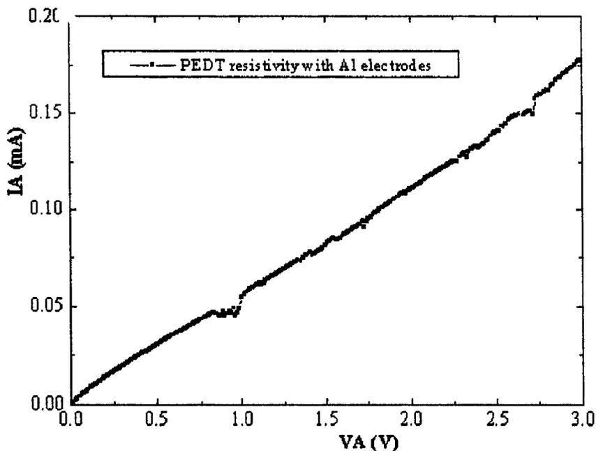
Figure 2-5 I-V Curve of PEDT thin-film with Al electrodes
