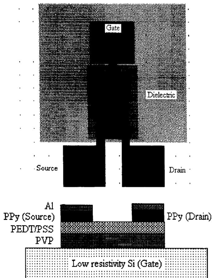
Figure 4-11 Mask (Top) and schematic structure (Bottom) of PEDT/PSS FETs
