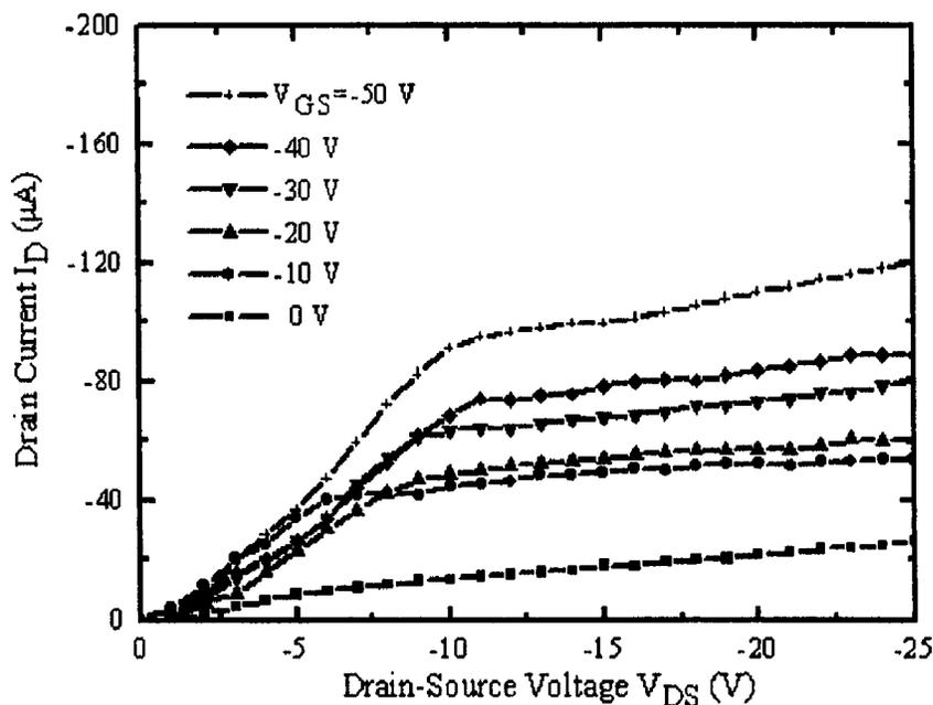
Figure 4-13 Drain characteristics of PEDT/PSS OFET with  $n^+$  Si as gate
