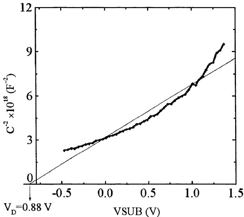
Figure 2-10 Reverse bias  $C^{-2} \sim V$  plot of Al/(PEDT/PSS) Schottky diode
