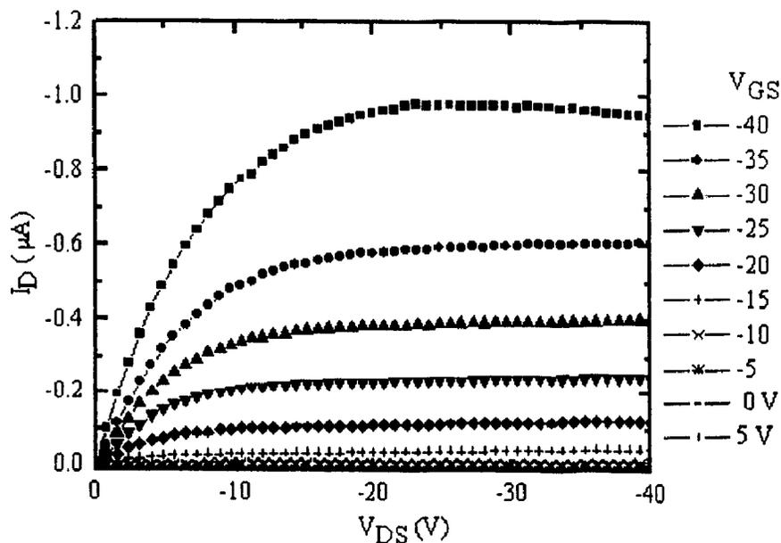
Figure 5-11 Drain characteristics of pentacene FET with thermal oxide as insulator
