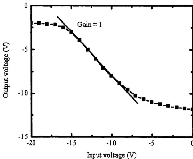
Figure 5-34 Transfer characteristics of pentacene inverter
