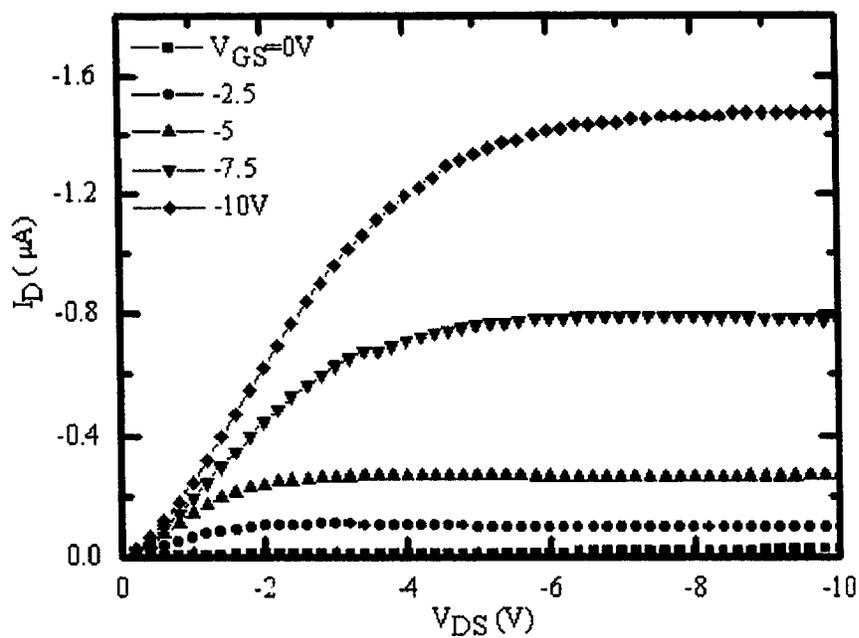
Figure 5-26 Drain characteristics of dual-gate pentacene FET
