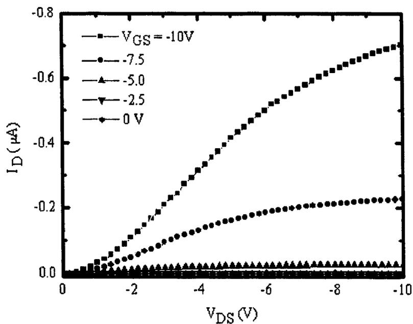
Figure 5-28 Drain characteristics of bottom part of dual-gate pentacene FET
