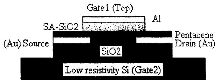
Figure 5-25 Schematic cross-section view of dual-gate pentacene OFETs
