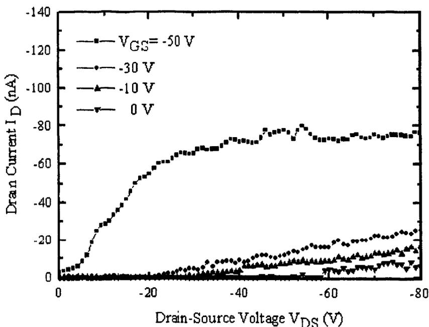
Figure 4-17  $I_D \sim V_{DS}$  curve of all-organic PEDT/PSS FET
