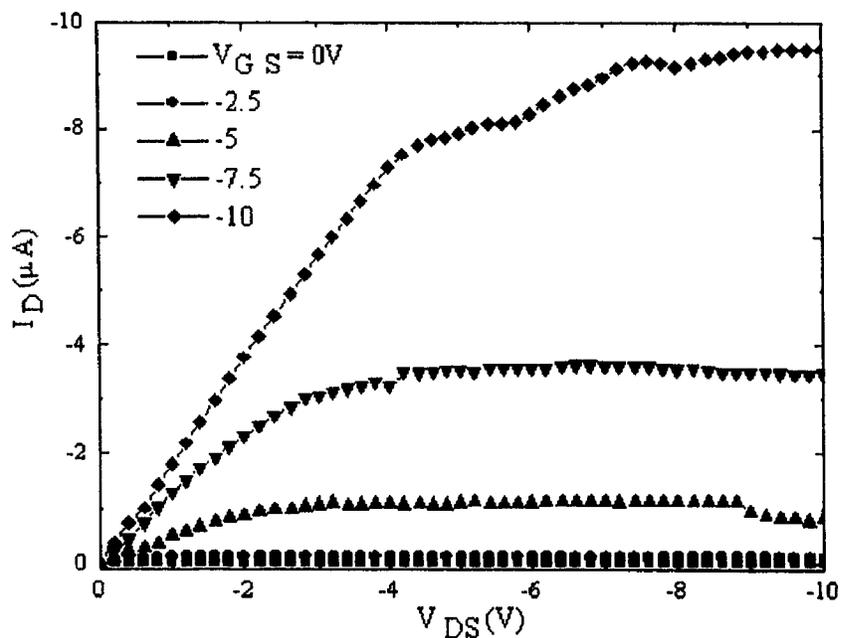
Figure 5-5 Drain characteristics of pentacene FET after one day
