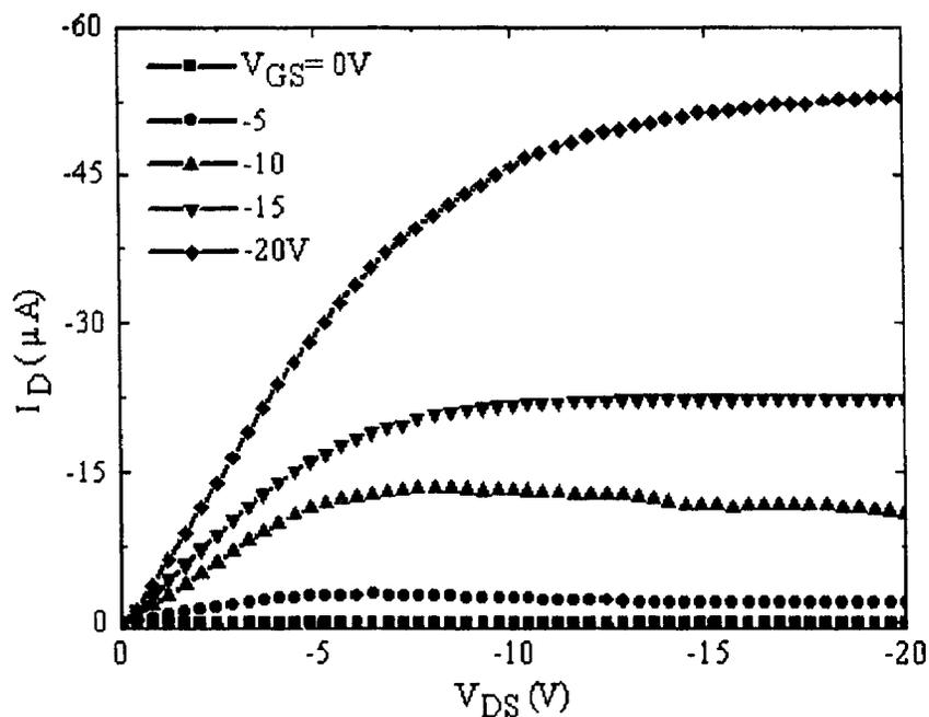
Figure 5-3 Drain characteristics of pentacene FET with thermal oxide as insulator
