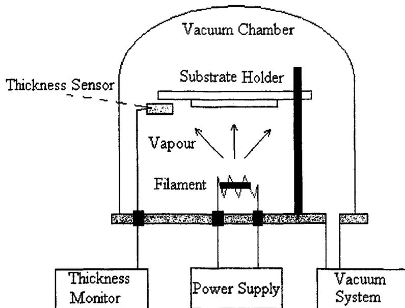
Figure 1-7 A schematic setup of the evaporator
