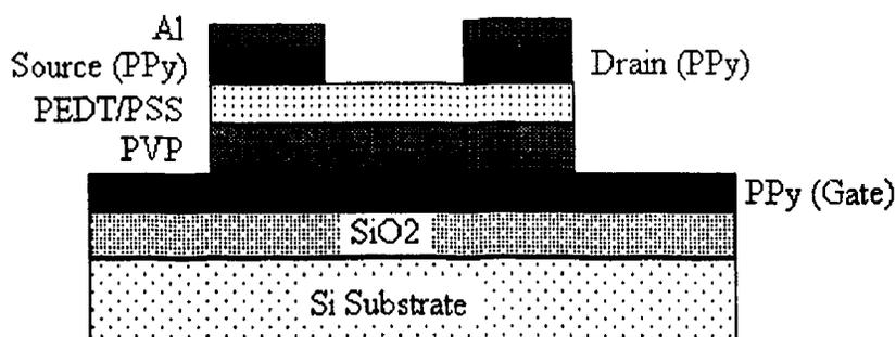
Figure 4-15 Schematic cross-sectional view of all-organic PEDT/PSS FETs
