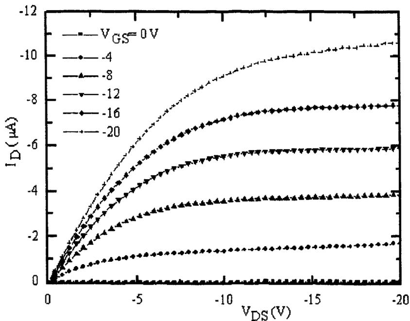
Figure 5-23 Drain characteristics of pentacene FET with oxygen plasma treatment
