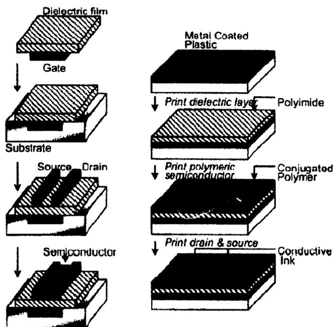
Figure 1-11 Two constructing strategies for all-polymer FETs (Left <sup>[31]</sup>, right <sup>[32]</sup>)
