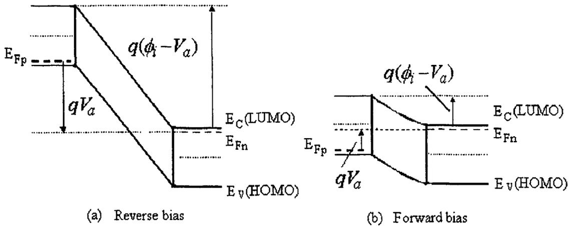
Figure 3-4 Energy band diagram of a p-n diode under forward bias and reverse bias
