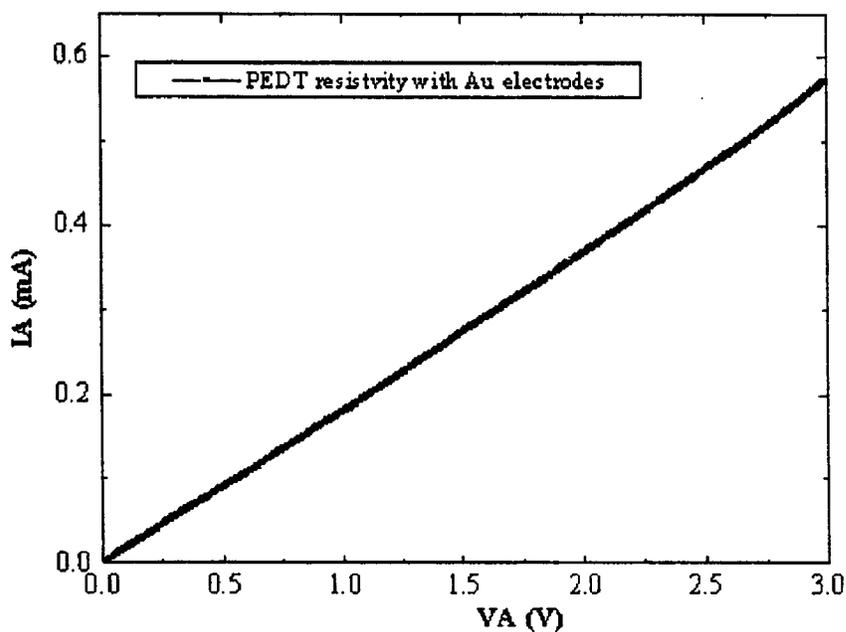
Figure 2-4 I-V Curve of PEDT thin-film with Au electrodes
