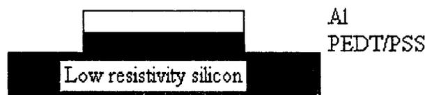
Figure 2-6 Schematic diagram of polymer Schottky diode structure
