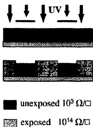
Figure 1-8 Process of photochemical lithography<sup>[7]</sup>
