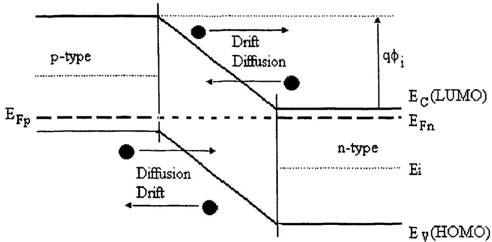
Figure 3-3 Energy band diagram of a p-n junction in thermal equilibrium
