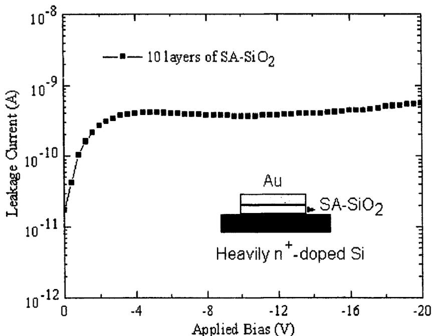
Figure 5-16 Gate leakage characteristic of Au/(SA-SiO<sub>2</sub>)/Heavily-doped Si structure
