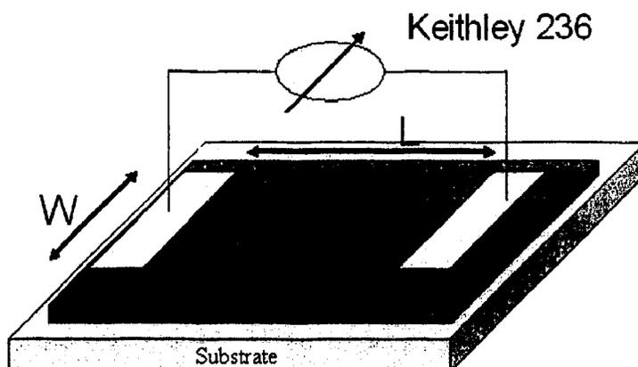
Figure 2-3 Parallel electrodes set-up for PEDT/PSS resistivity measurement
