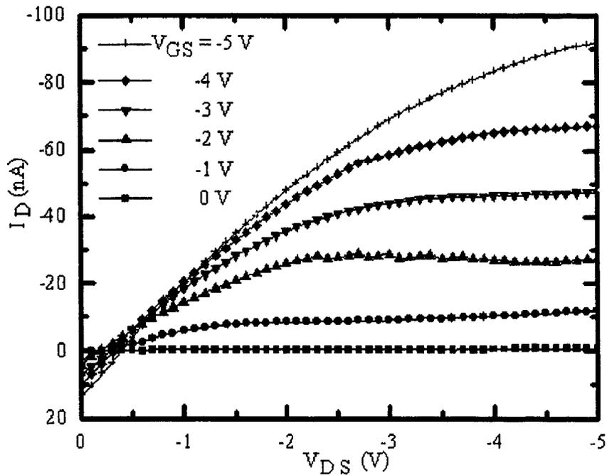
Figure 5-19 Drain characteristics of pentacene FET with SA-SiO<sub>2</sub> as insulator
