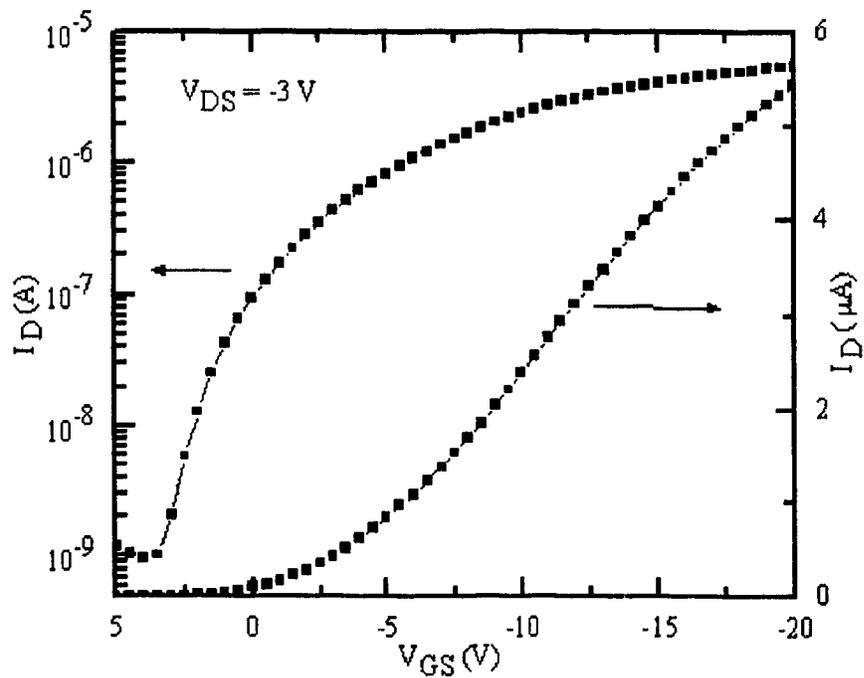
Figure 5-24 Gate characteristics of pentacene FET with oxygen plasma treatment
