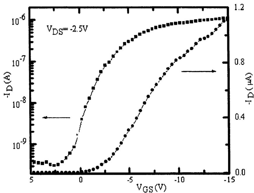
Figure 5-27 Gate characteristics of dual-gate Pentacene FET
