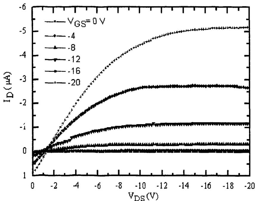
Figure 5-21 Drain characteristics of pentacene FET without  $O_2$  plasma treatment
