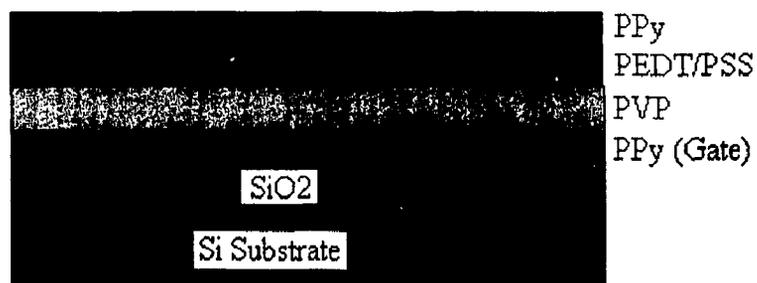
e. Spin-coat a layer of PPy as the Source/Drain electrode;
