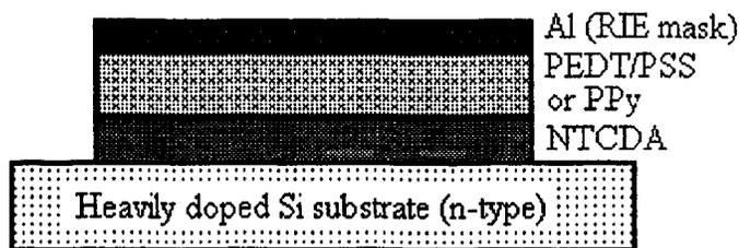
Figure 3-5 Schematic structure of organic diodes with Al as RIE pattern mask
