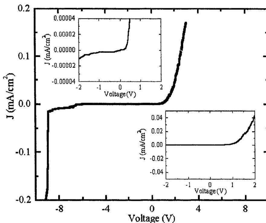
Figure 3-7 Current-voltage characteristics of NTCDA/PPy diode
