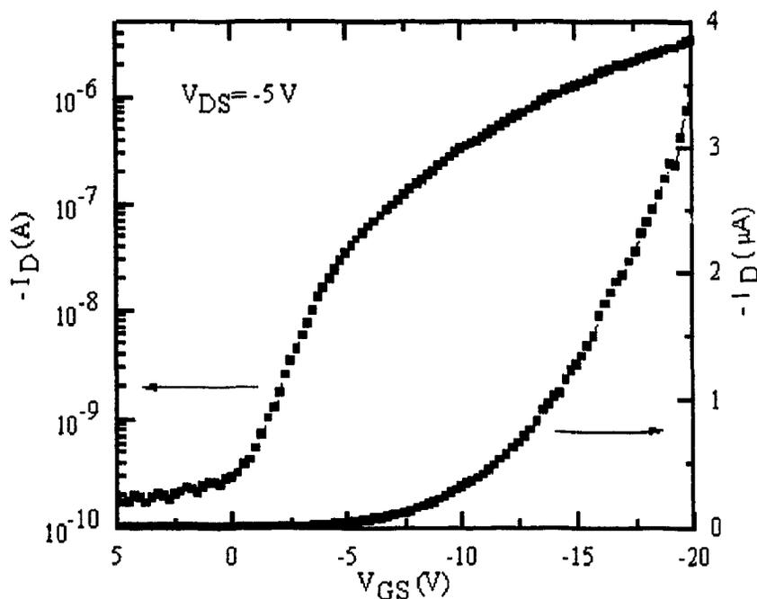
Figure 5-22 Gate characteristics of pentacene FET without  $O_2$  plasma treatment
