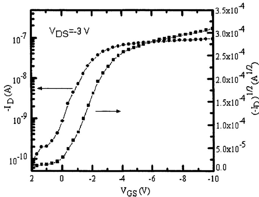
Figure 5-20 Gate characteristics of pentacene FET with SA-SiO<sub>2</sub> as insulator
