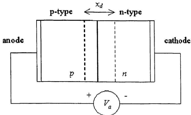
Figure 3-1 Cross-section of a p-n junction
