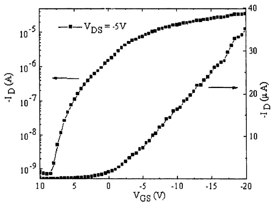
Figure 5-4 Gate characteristics of pentacene FET with thermal oxide as insulator
