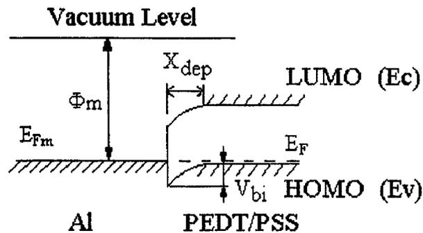
Figure 2-1 Schematic band diagram of metal/polymer contact under zero bias
