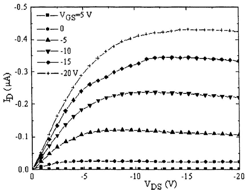
Figure 5-7 Drain characteristics of pentacene FET after one week
