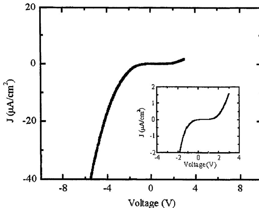
Figure 3-9 I-V characteristics of NTCDA/PPy after the acetone treatment
