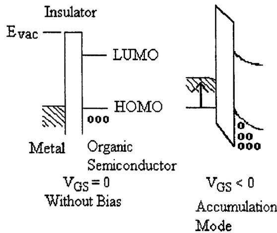
Figure 4-2 Schematic Band diagram of p-type OFET
