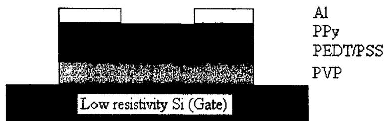
h. Pattern Al to form Source/Drain mask by wet-etching;
