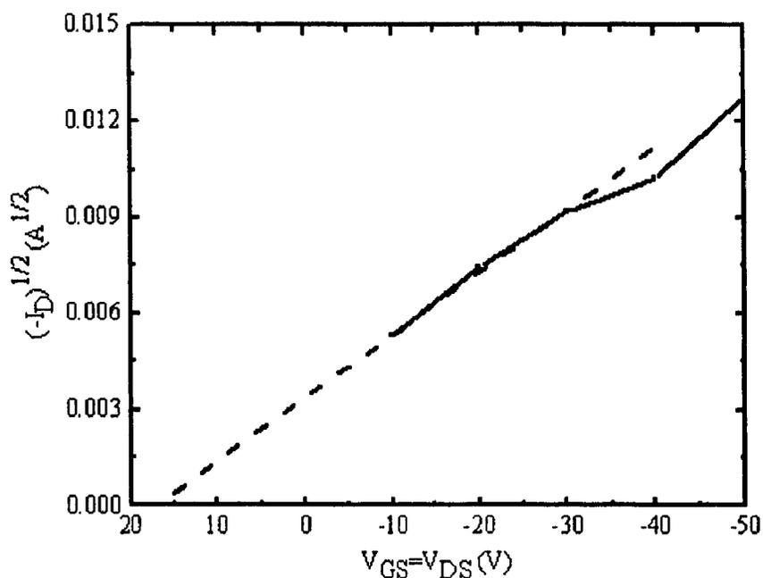
Figure 4-14  $I_D^{1/2}$  vs.  $V_{GS}$  of PEDT/PSS OFET with  $n^+$  Si as gate
