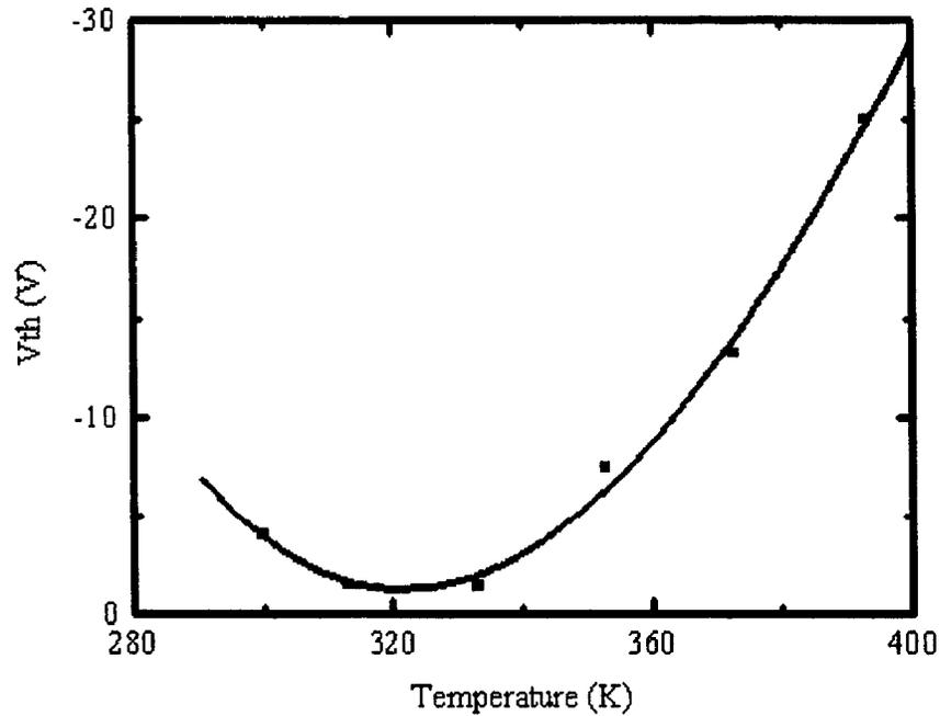
Figure 5-15 Temperature dependence of threshold voltage for pentacene FET
