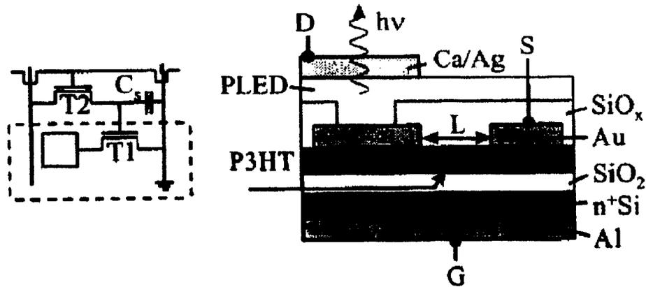
Figure 1-4 Schematic diagram of integrated polymer FET-LED <sup>[9]</sup>
