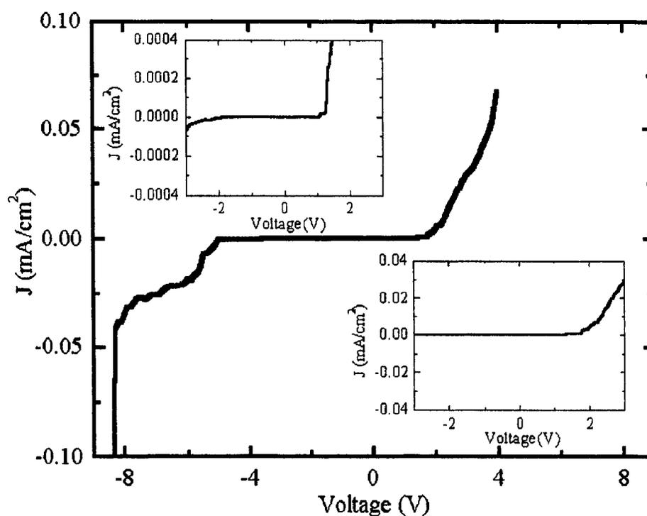
Figure 3-8 Current-voltage characteristics of NTCDA/(PEDT/PSS) diode
