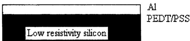
(c) Thermally evaporate a layer of Al: 200nm.
