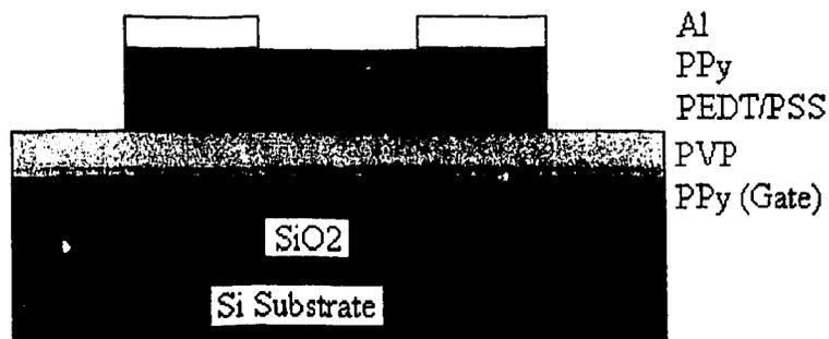
i. Pattern Al to form Source/Drain mask by wet-etching;
