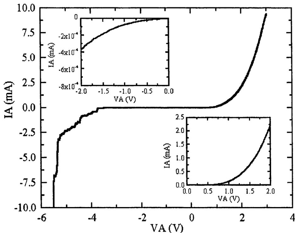
Figure 2-8 I-V characteristics of Al/(PEDT/PSS) contact
