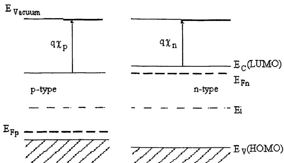
Figure 3-2 Band diagram of a p-n junction before contact
