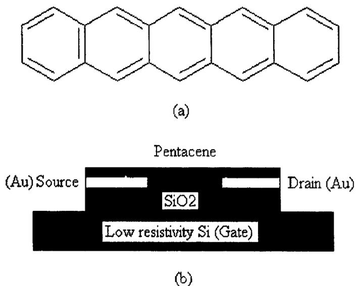
Figure 5-1 (a) Pentacene molecular; (b) Schematic structure of pentacene OFETs
