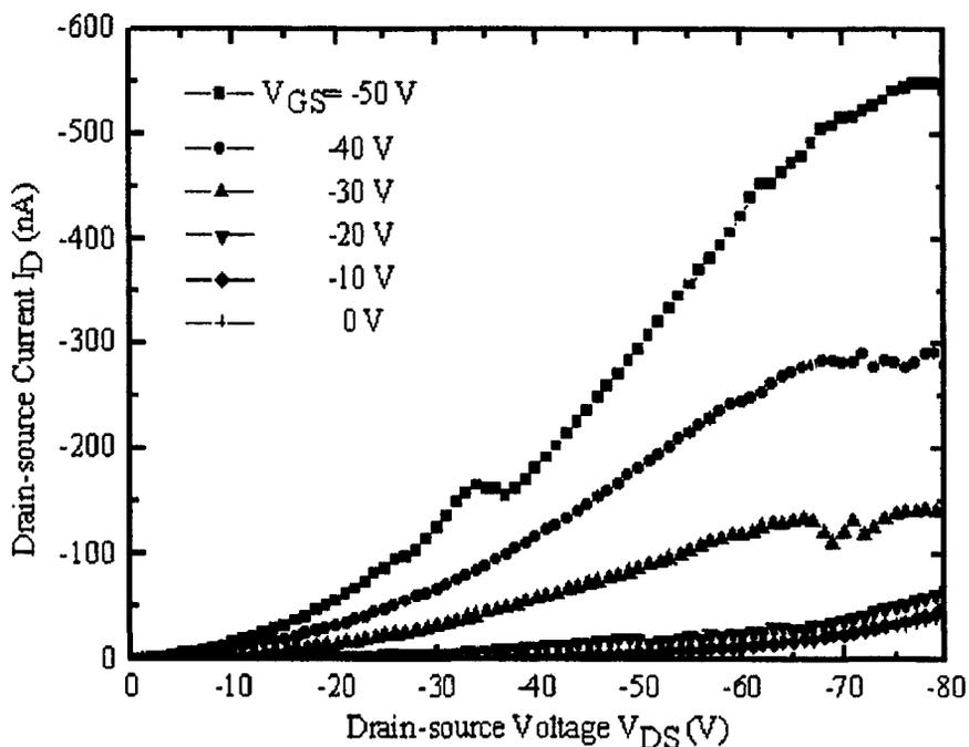
Figure 4-19 Drain characteristics of improved all-organic PEDT/PSS FET
