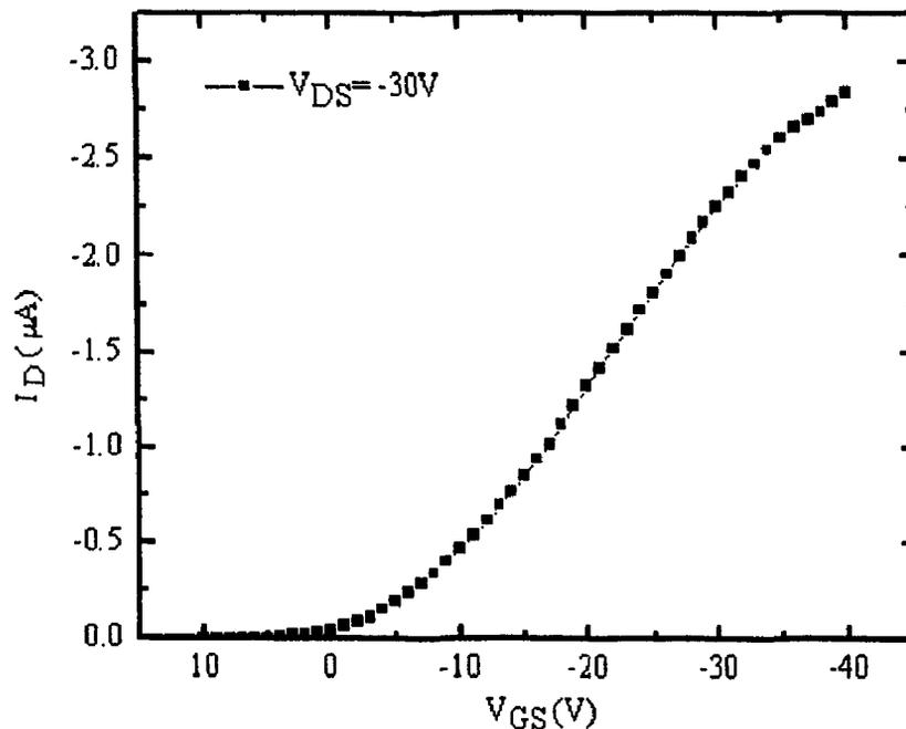
Figure 5-12 Gate characteristics of pentacene FET with thermal oxide as insulator
