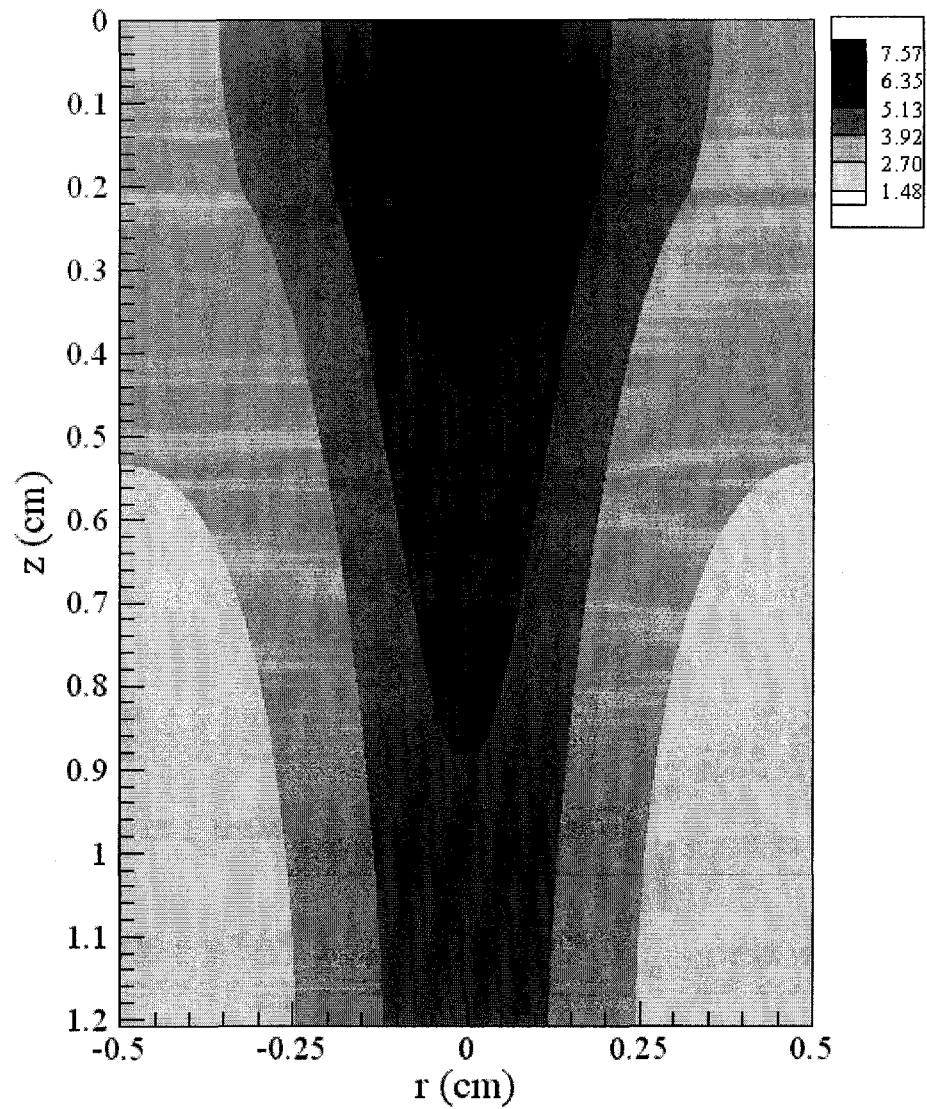
Figure 4.19 The contours of the elevated temperature distributions in the cross section with \varphi = 0 and \varphi = \pi , at t = 1536 seconds without any blood vessels
