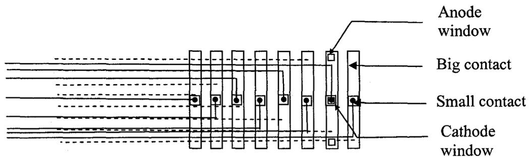
Figure 29. Making windows on the contacts.
