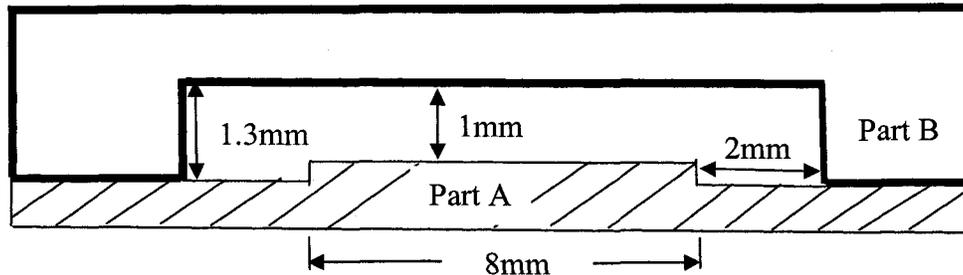
Figure 26. The mold for making FINE.
