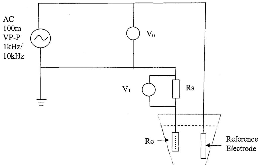
Figure 37. Setup for impedance measurement.
