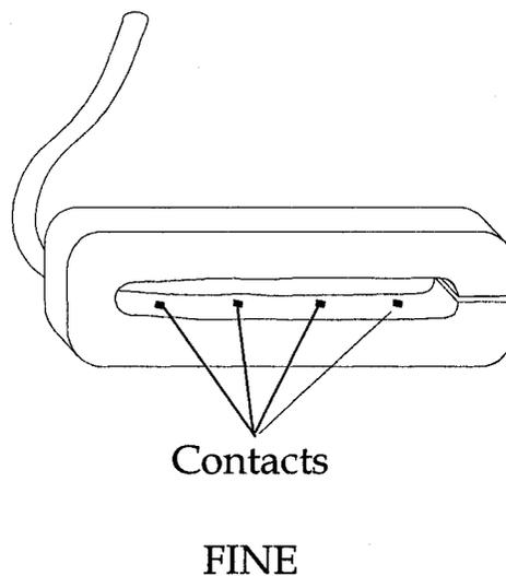
Figure 7. The Flat Interface Nerve Electrode (FINE).
