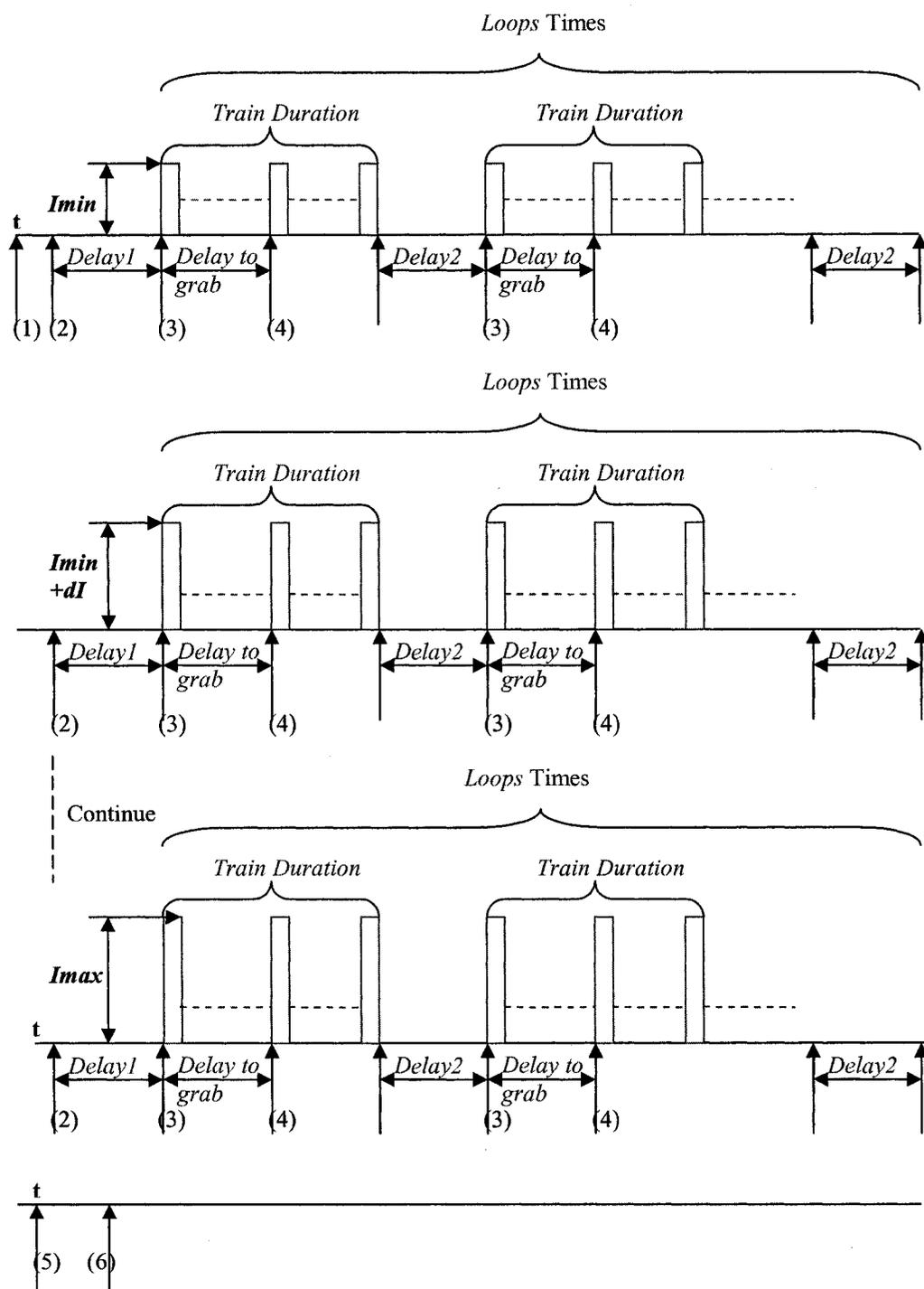
Figure 13. The figure shows the delays and incensement of stimulus pulses in the LabView program.
