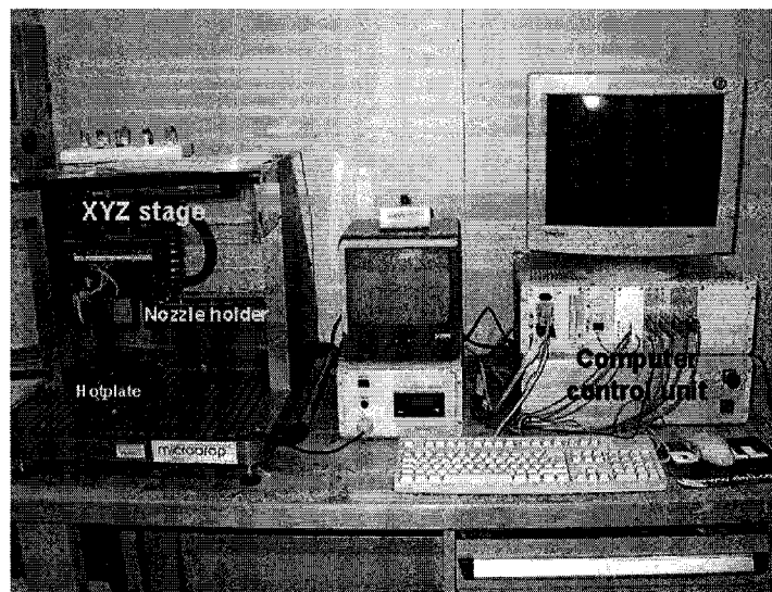
Figure 3-2 The Microdrop Dispensing System.
