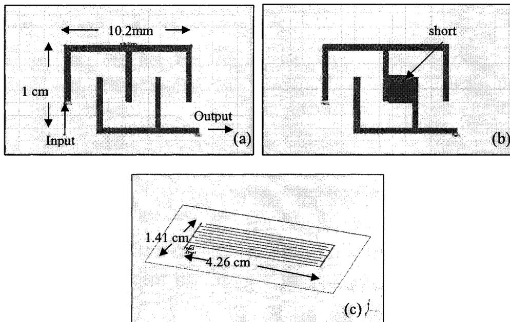
**Figure 4.15** Sensor switch layout for QTC and freshness sensors (a) interdigitated simulated structure (1.02 cm x 1 cm) (b) with short circuited electrodes (c) structure with large form factor (1.41 cm x 4.26 cm).
