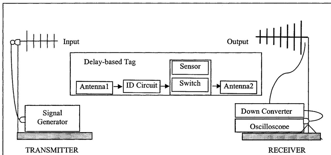
**Figure 2.3 Schematic diagram of delay-based RFID system.**
