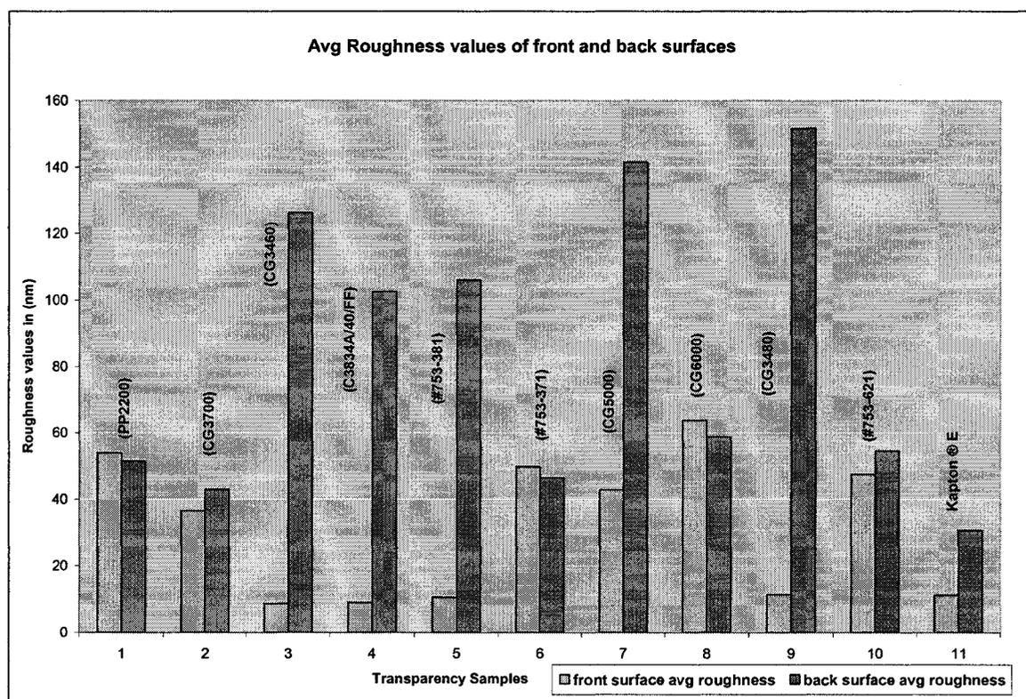
**Figure 3.1 Average roughness values of the flexible substrates under consideration.**
