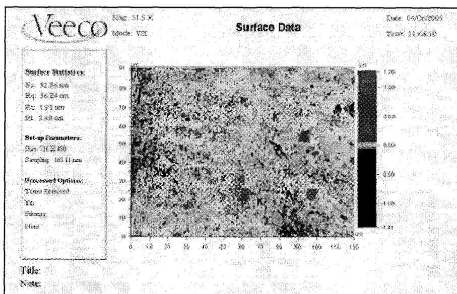
**Figure 3.14 R.S.T diagram showing roughness of the electroless deposited copper.**
