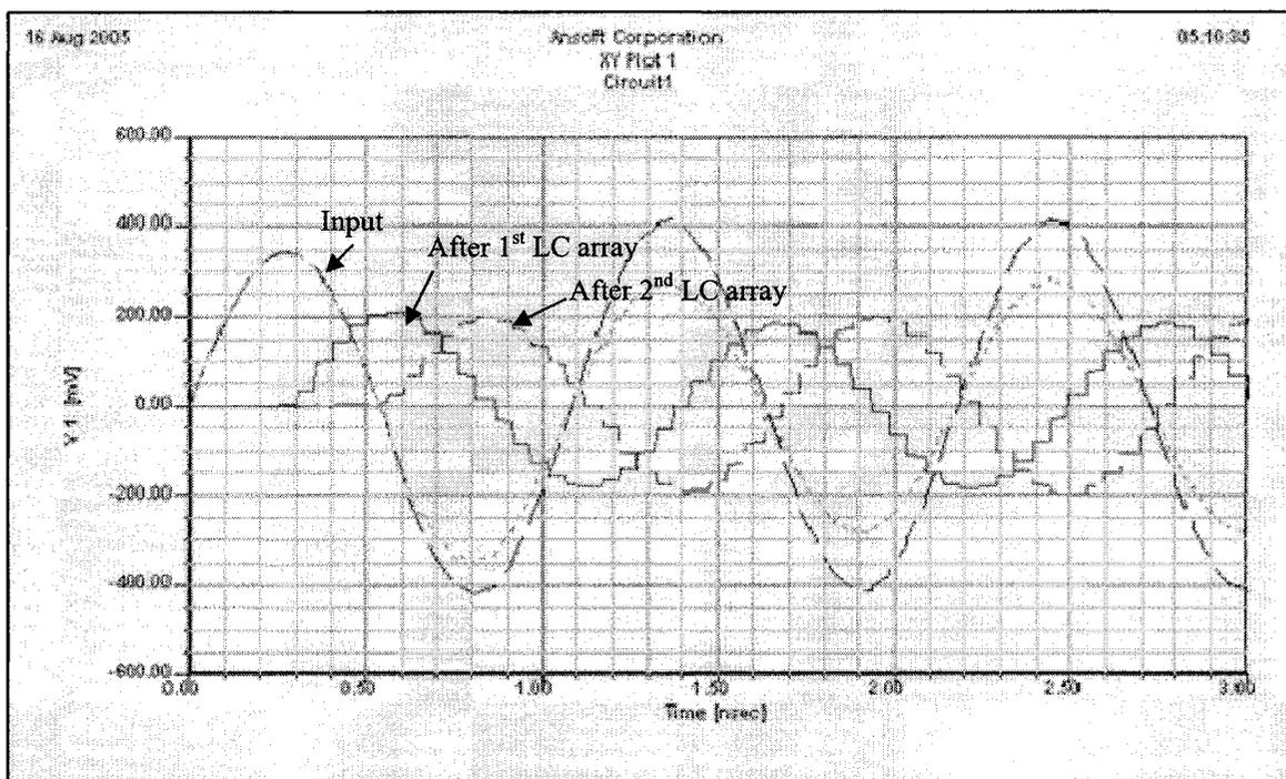
**Figure 5.2** Input and output signals after 1<sup>st</sup> and 2<sup>nd</sup> delay lines of the ID circuit.
