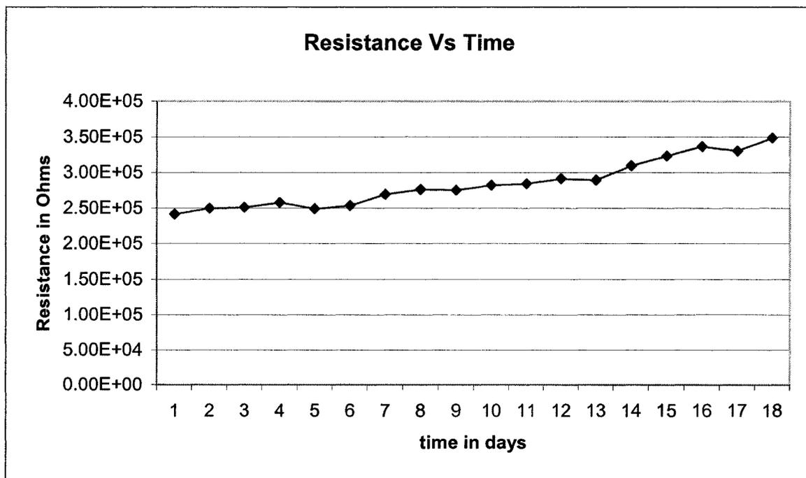
**Figure 3.17 Resistance vs time graph of PEDOT/PSS resistor patterns protected by polyimide.**
