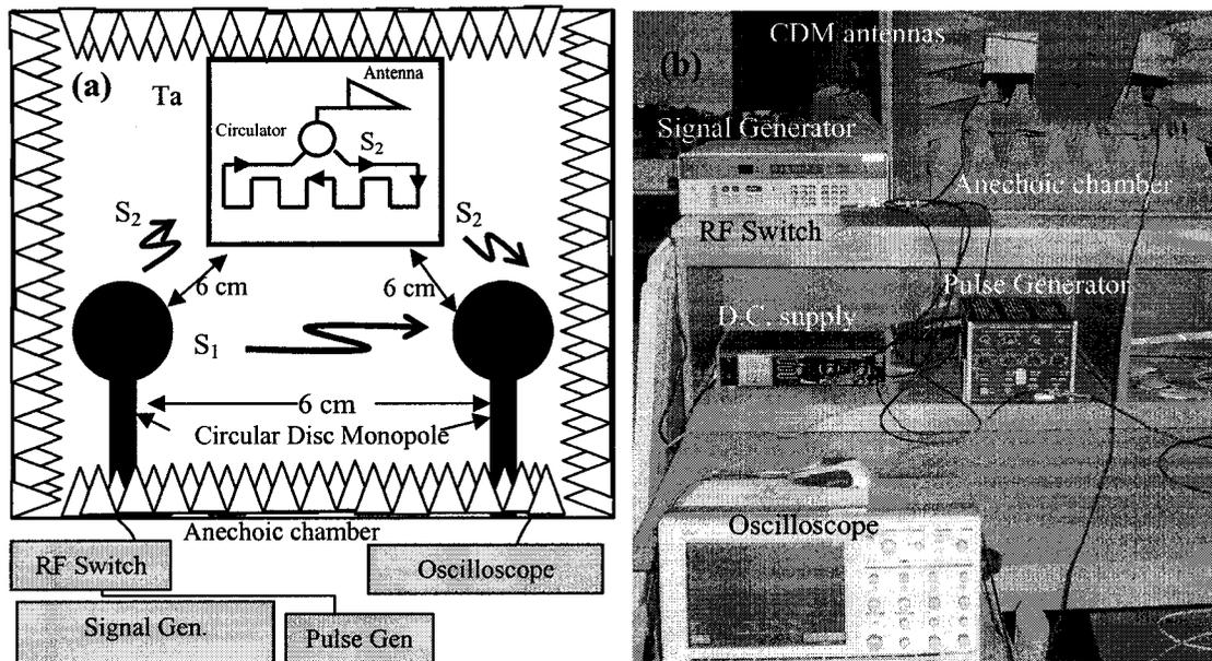
**Figure 6.19 (a) Schematic diagram of experimental setup with Circular Disc Monopole antennas and the tag inside the anechoic chamber
