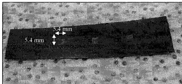
**Figure 4.8 Capacitors patterned with laser printer and electroless plated on a polyimide substrate.**
