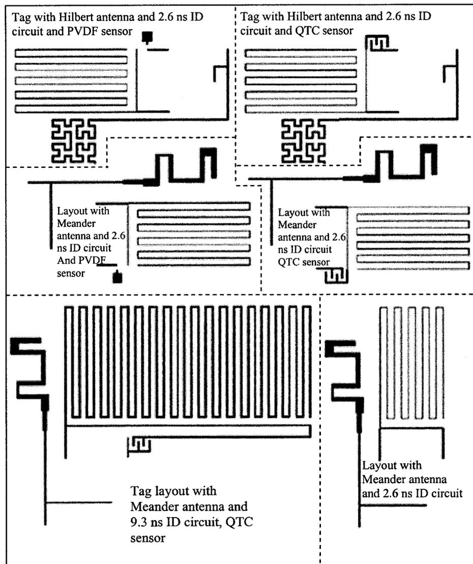
**Figure 6.8 Mask layout with different RFID and RFID-based sensor configurations.**
