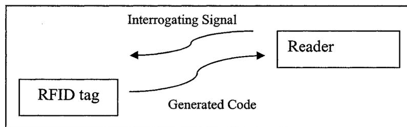
**Figure 1.1 Schematic diagram showing a typical RFID system.**
