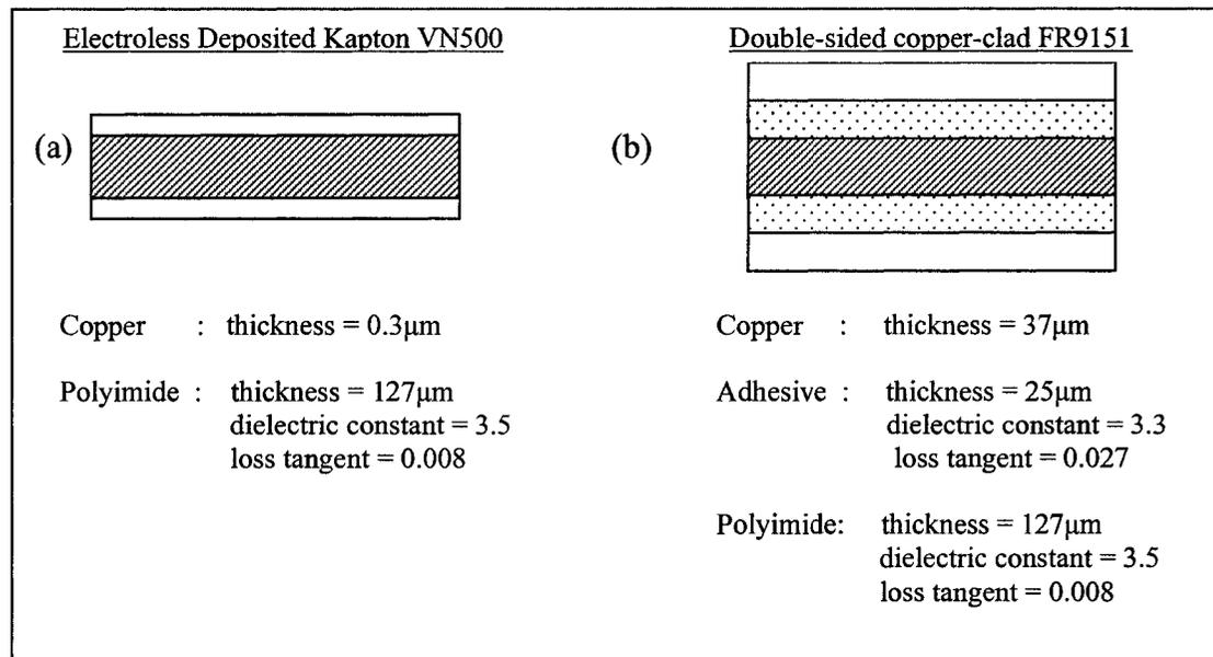
**Figure 4.1 Layout architecture for modeling and simulations (a) substrate stack up for proposed low-cost fabrication on Kapton VN500 (b) substrate stack up for silicon-based processes on FR9151.**
