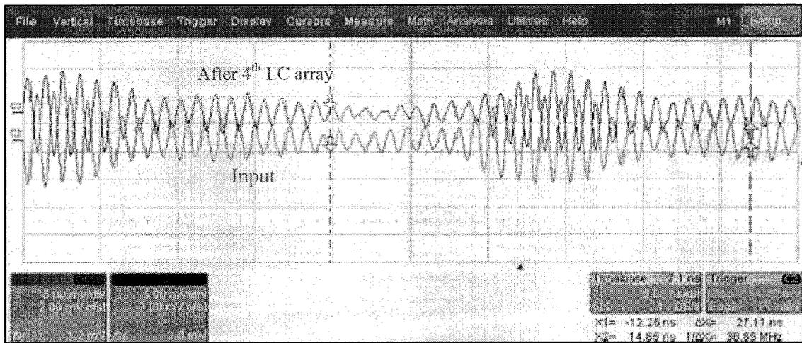
**Figure 5.16 Signal at the input and output of four LC array series of the ID generation circuit showing the time delay in the oscilloscope (x axis = 5 ns/div; y axis = 5 mV/div).**
