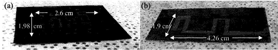
**Figure 4.14 (a) Hilbert antenna and (b) Meander antenna, fabricated using low-cost processes on Kapton 500VN.**
