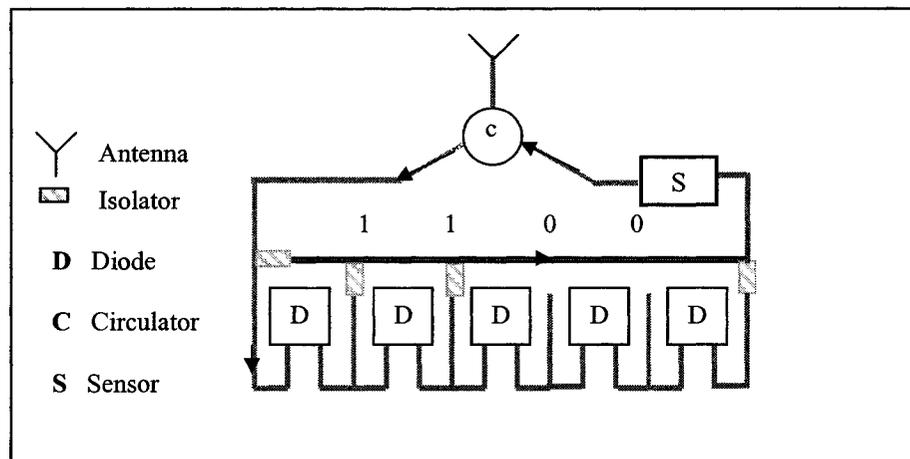
**Figure 2.9 Circuit diagram of transmission-delay-line-based RFID tag.**
