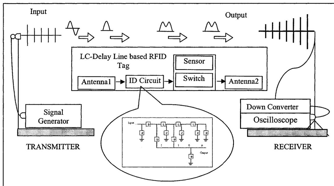
**Figure 2.6 Schematic diagram of a typical LC-delay-line-based RFID system.**
