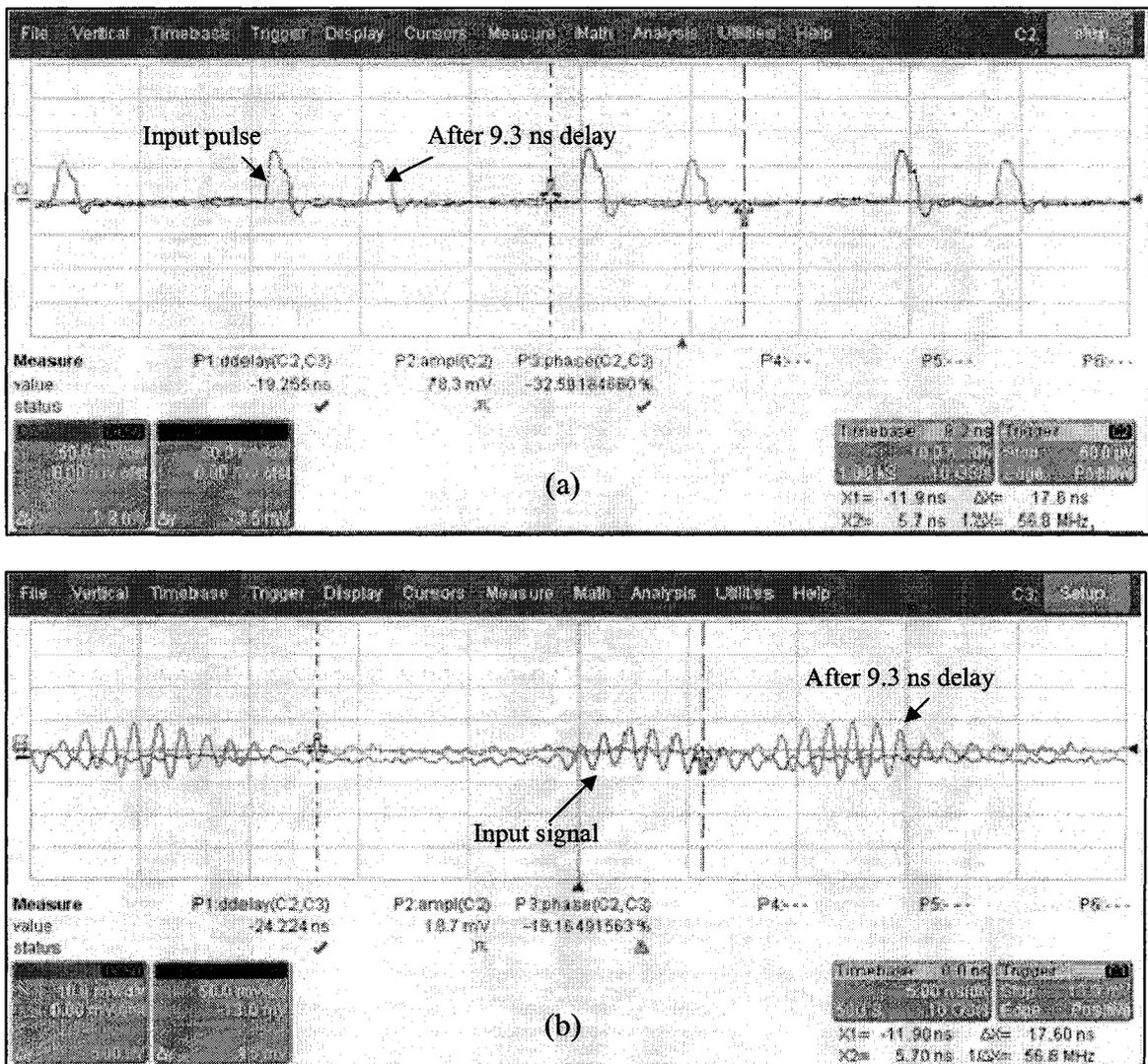
**Figure 6.6 Delay observed in the 1GHz digital oscilloscope for (a) pulse input (b) OOK modulated signal of 915 MHz center frequency using 5 ns pulse, 31.3 MHz PRF.**
