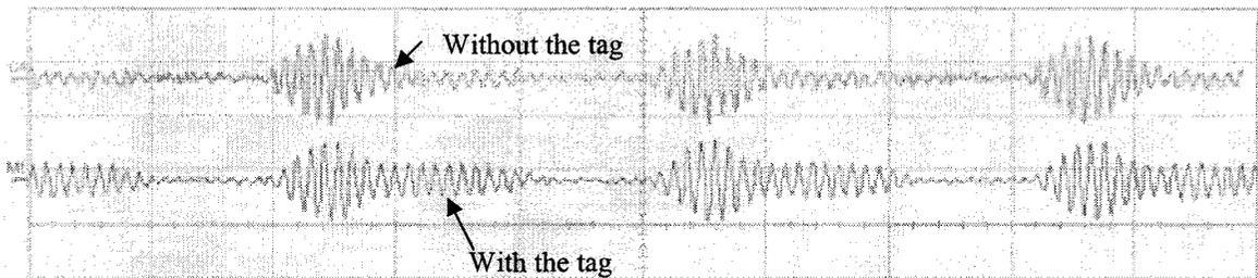
**Figure 6.20 Signal received by the oscilloscope from the transmitter in the absence and presence of the tag (x-axis, 10 ns/div; y-axis, 100 mV/div).**
