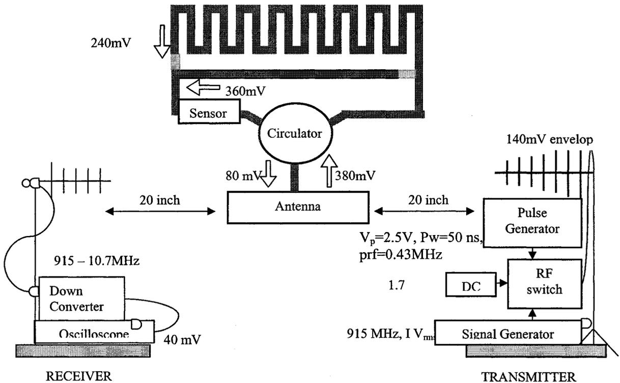
**Figure 6.12 Schematic diagram showing the test set up with different signal levels observed.**
