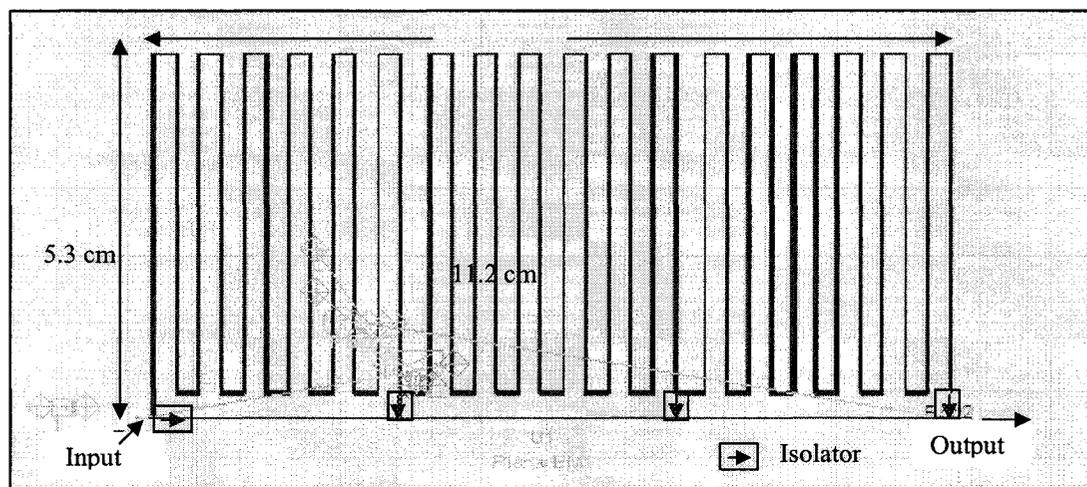
**Figure 6.2 Schematic showing simulated 9.3 ns delay ID generation circuit.**
