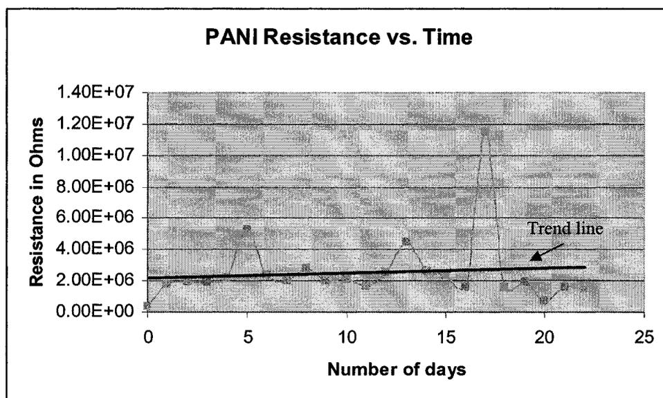
**Figure 3.16 Resistance vs time graph of polyimide coated PANI resistor patterns.**
