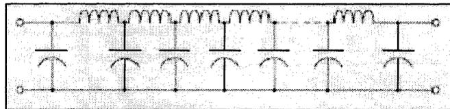
**Figure 2.4 Equivalent circuit diagram of a transmission line.**
