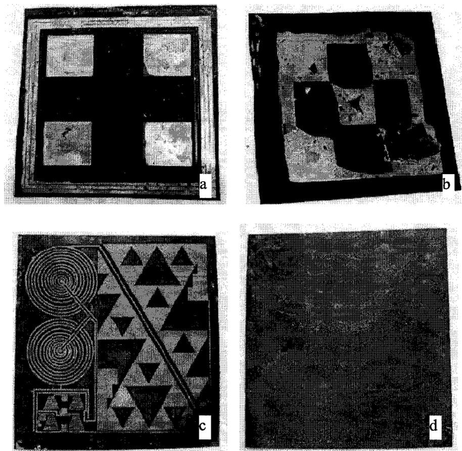
**Figure 3.12 Effect of activation and acceleration preconditioning method-1 on copper deposition of 13.56MHz layout (a) front side (b) bottom side. Preconditioning method-2 on 915 MHz layout (c) front side (d) bottom side (note: dimensions are not to the scale).**
