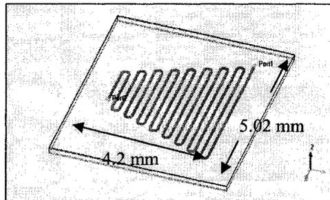
**Figure 4.5 Modified inductor layout for photolithography on FR9151.**
