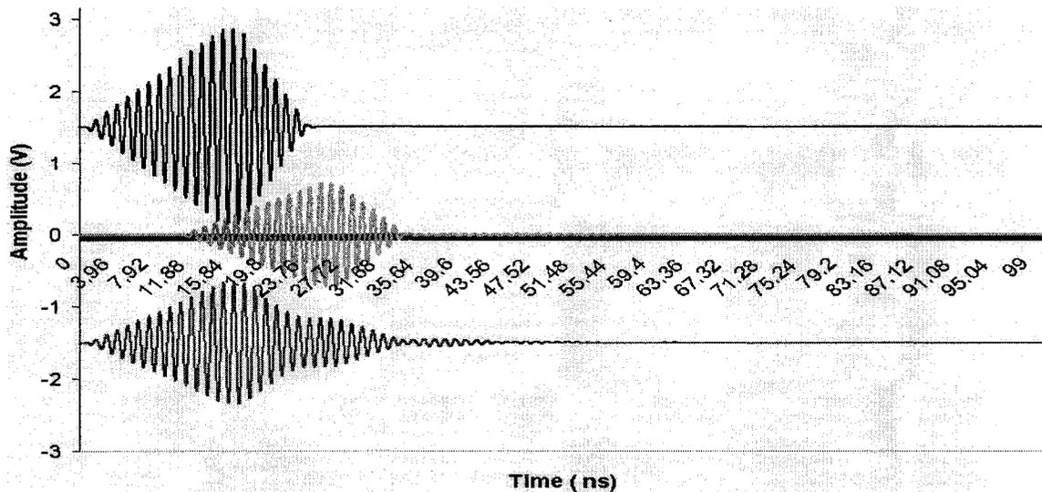
**Figure 6.13 Simulated input signal, delayed signal and the output signal of the tag in receiving mode.**
