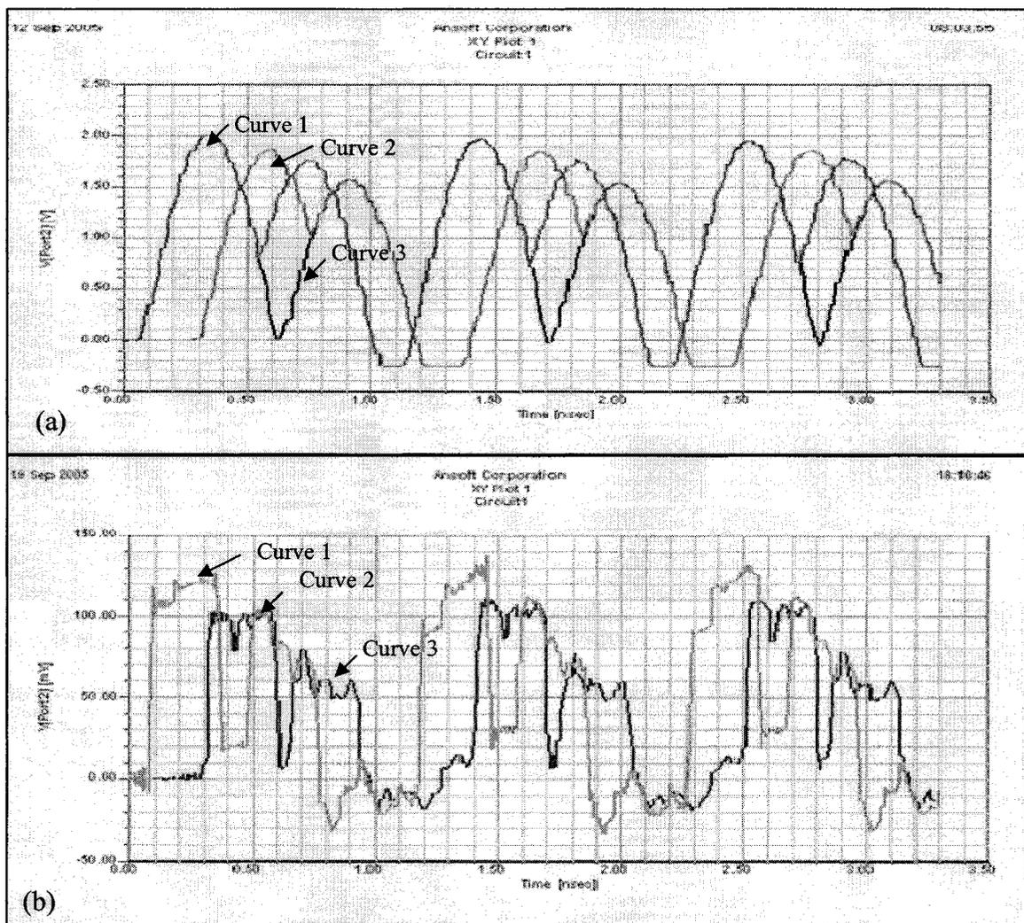
**Figure 6.3 Different bit code generation by ID generation circuit response to (a) half wave rectified sinusoidal input (b) pulse input.**
