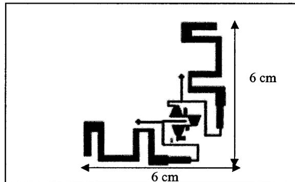
**Figure 5.4 RFID tag with impedance matched ID circuit and tuned antennas.**
