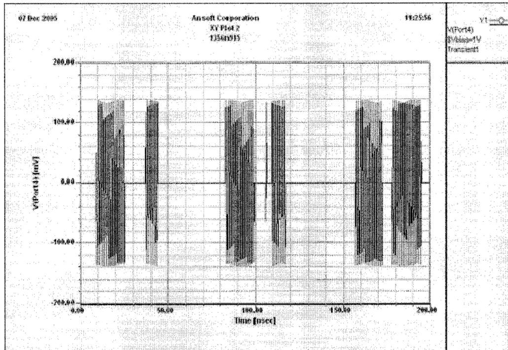
**Figure 7.3 Output obtained from the simulated circuit representing the tag and back-scatter modulation circuit.**
