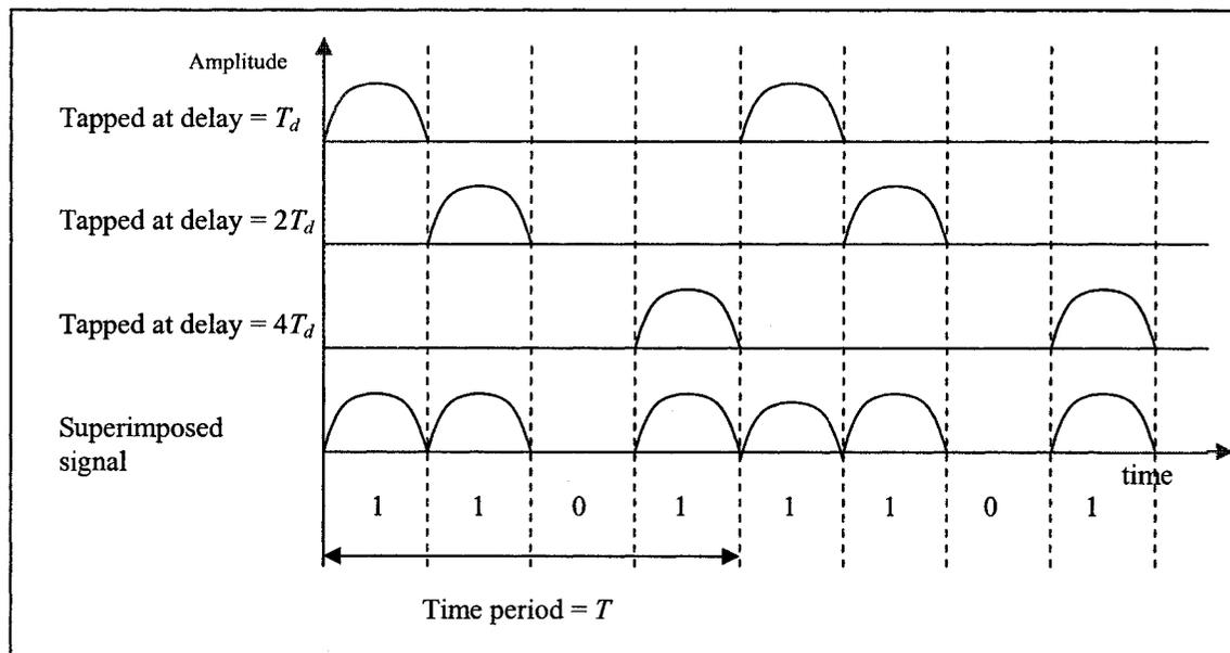
**Figure 2.5 Delay-based ID generation by superposing tapped signals at different delay.**
