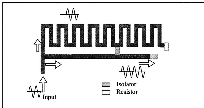
**Figure 6.1 Schematic diagram of ID generation circuit.**
