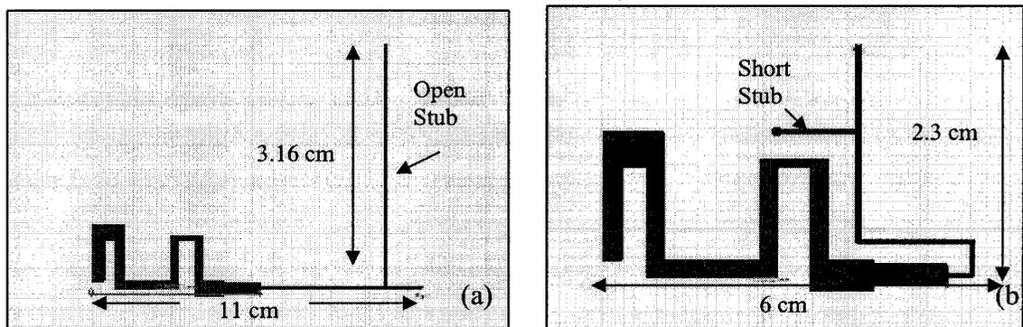
**Figure 5.3 (a) An open stub connected to a Meander antenna (b) Impedance matched antenna after adjusting the form factor and with a shorted stub.**
