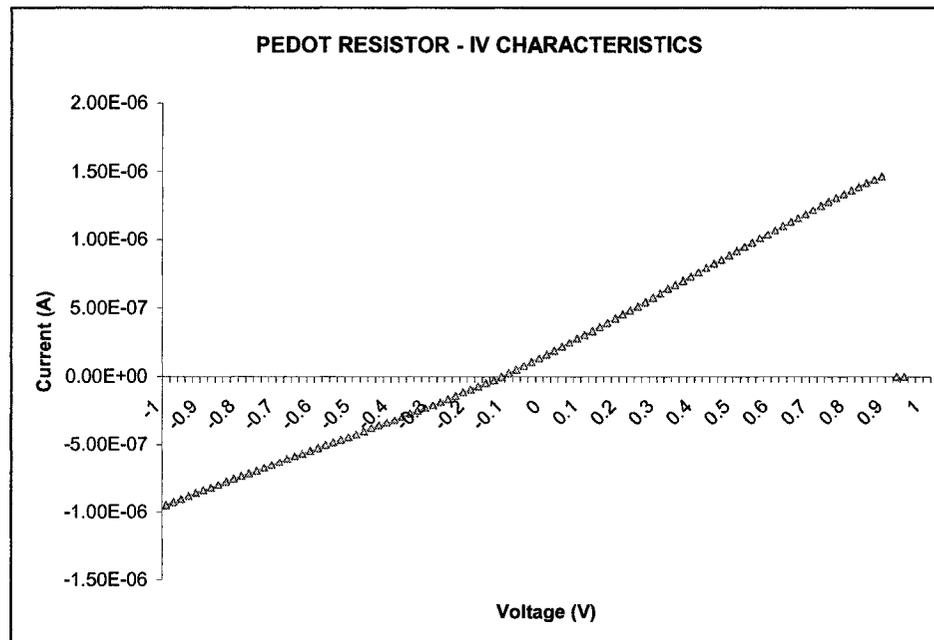
**Figure 4.10 DC characteristics of PEDOT/PSS resistor.**
