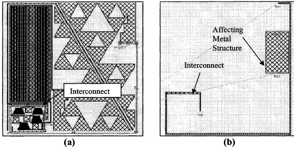
**Figure 5.5 Schematic showing (a) interconnect under consideration (b) set up to measure the proximity effects of a capacitor near by an inductor.**
