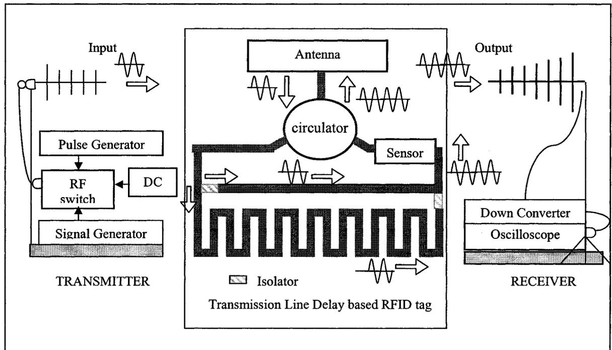
**Figure 2.8 Schematic of a transmission-delay-line-based RFID system.**
