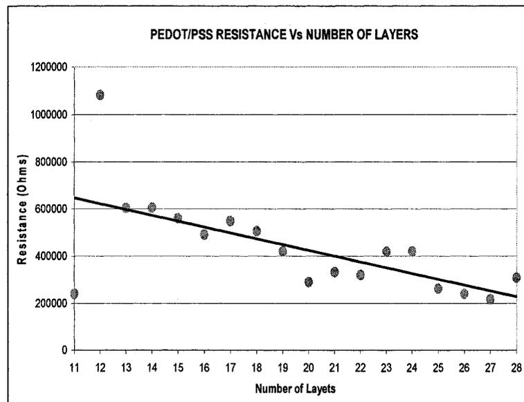
**Figure 3.9 Resistance changes of PEDOT/PSS patterns with the number of printed layers.**
