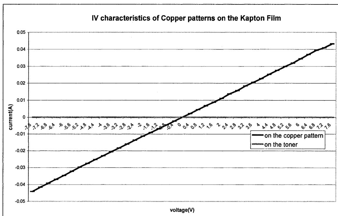
**Figure 3.5 I-V characteristic curves of copper pattern and toner.**
