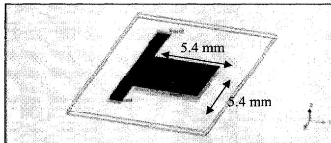
**Figure 4.7 Modified capacitor layout for photolithography on FR9151.**
