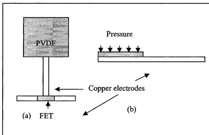
Figure 4.16 Layout for PVDF pressure sensor switch (a) top view (b) side view.
