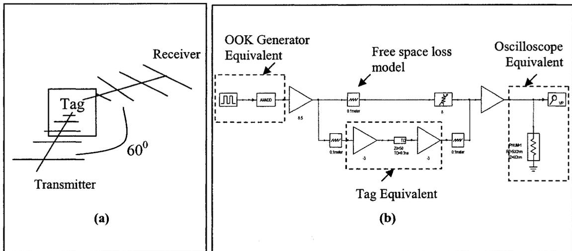
**Figure 6.16 (a) Schematic diagram of the experimental setup for complete tag testing (b) circuit equivalent of the experimental setup.**
