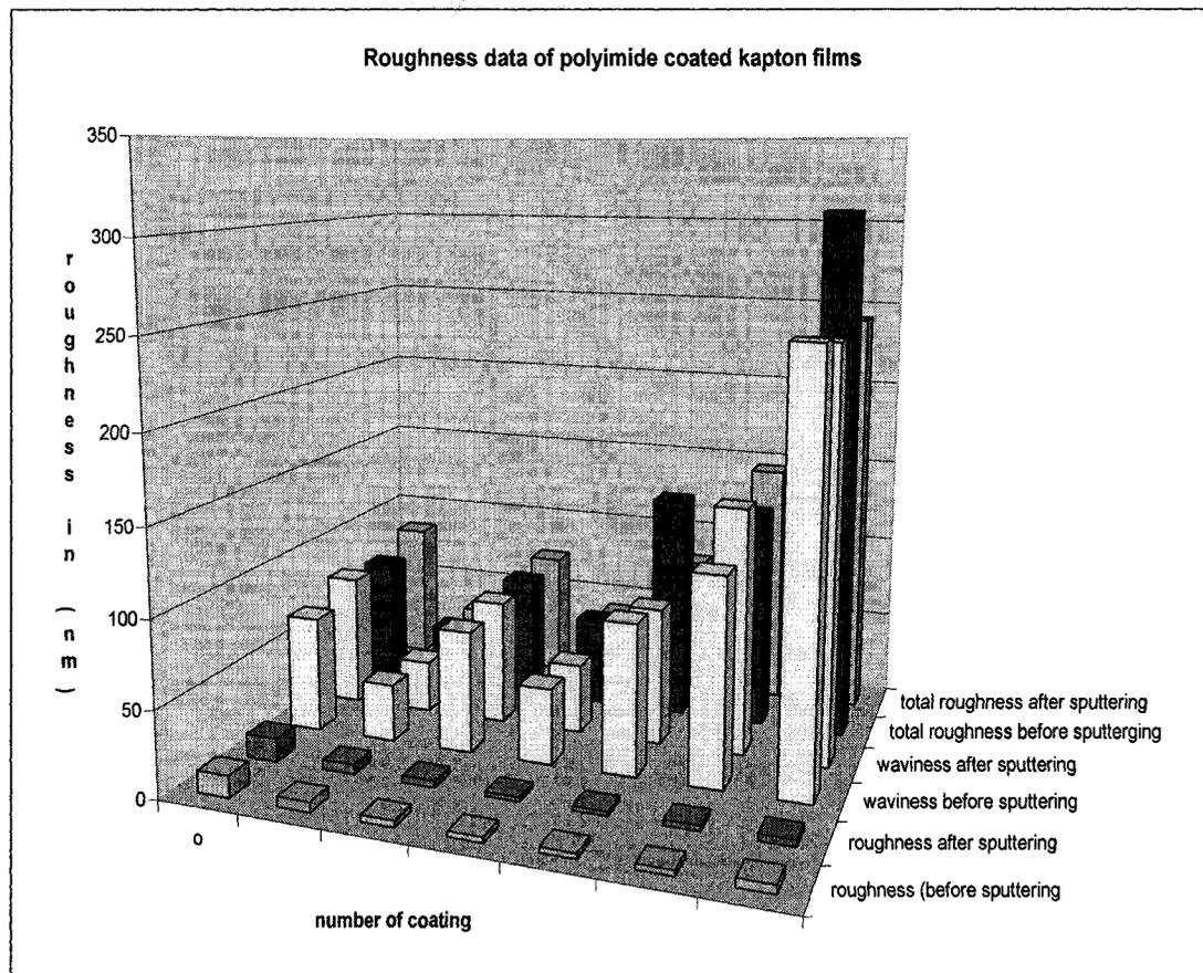
**Figure 3.4 Roughness parameters of polyimide coated Kapton 500VN films.**
