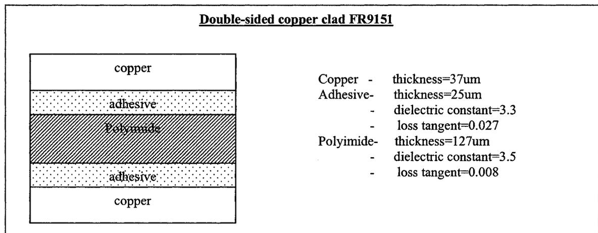
**Figure 3.20 Substrate stack up of FR9151 for simulations.**
