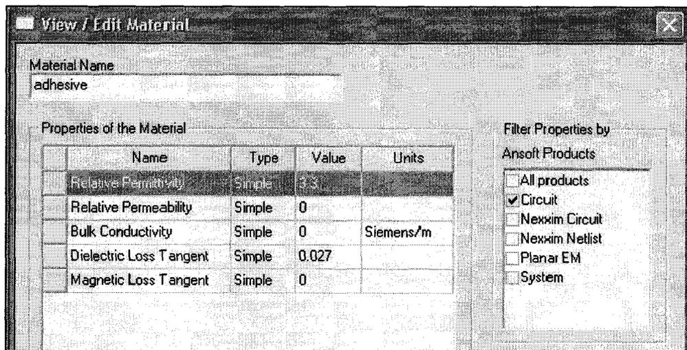
**Figure 4.2 Ansoft View/Edit Material window showing parameters of the adhesive material for FR9151.**
