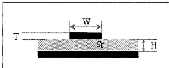
**Figure 4.3 Schematic diagram of a microstrip.**
