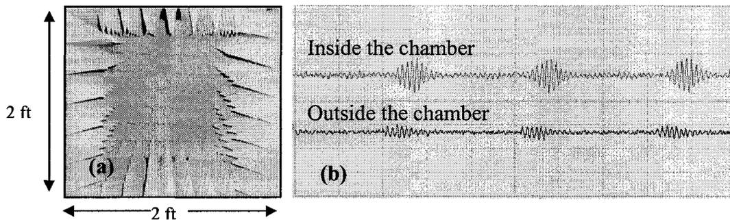
**Figure 6.18 (a) Custom built anechoic housing for tag testing (b) Effect of anechoic housing on the signal strength (x-axis = time, y-axis= voltage).**
