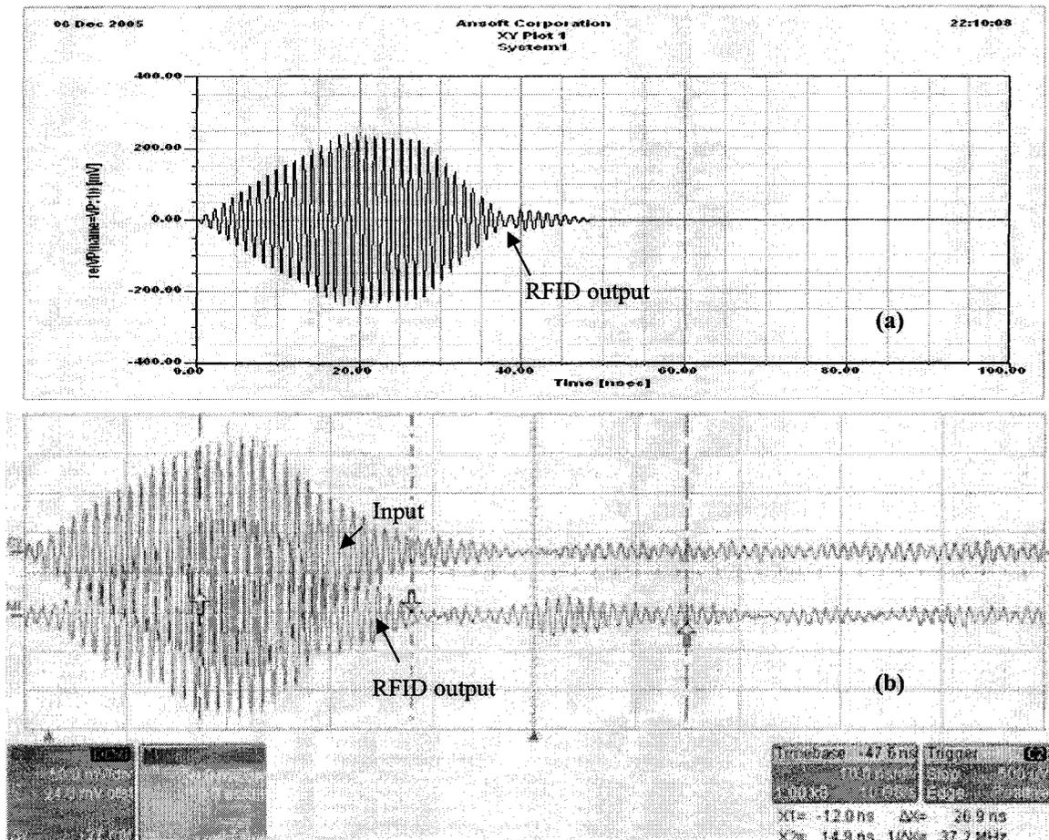
**Figure 6.17 (a) Simulated tag output at the oscilloscope (b) Input signal received by the oscilloscope when the tag is communicating with the external antennas (x-axis, 10 ns/div; y-axis, 50 mV/div).**
