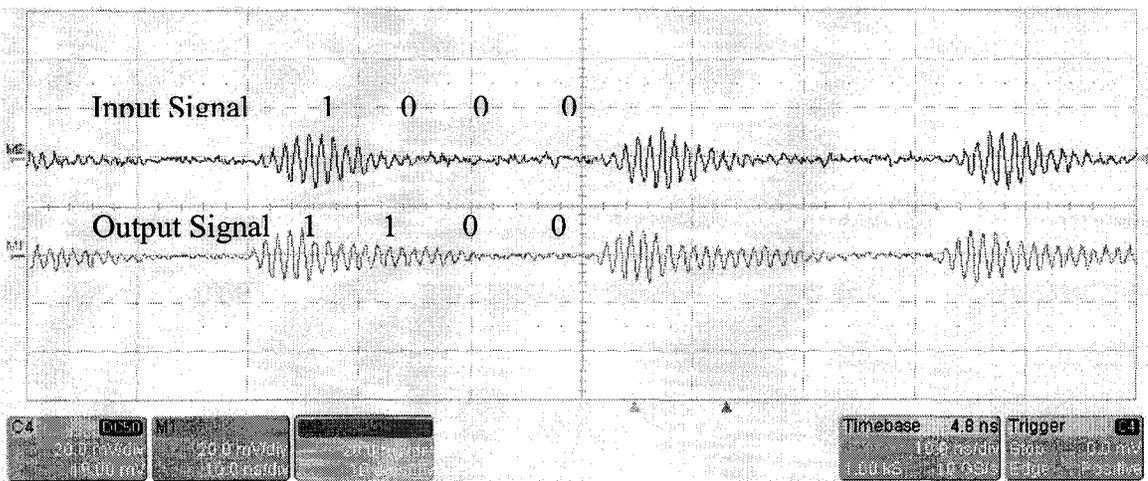
**Figure 6.15 Practical input and output from the tag in transmitting mode (for maximum coupled signal).**
