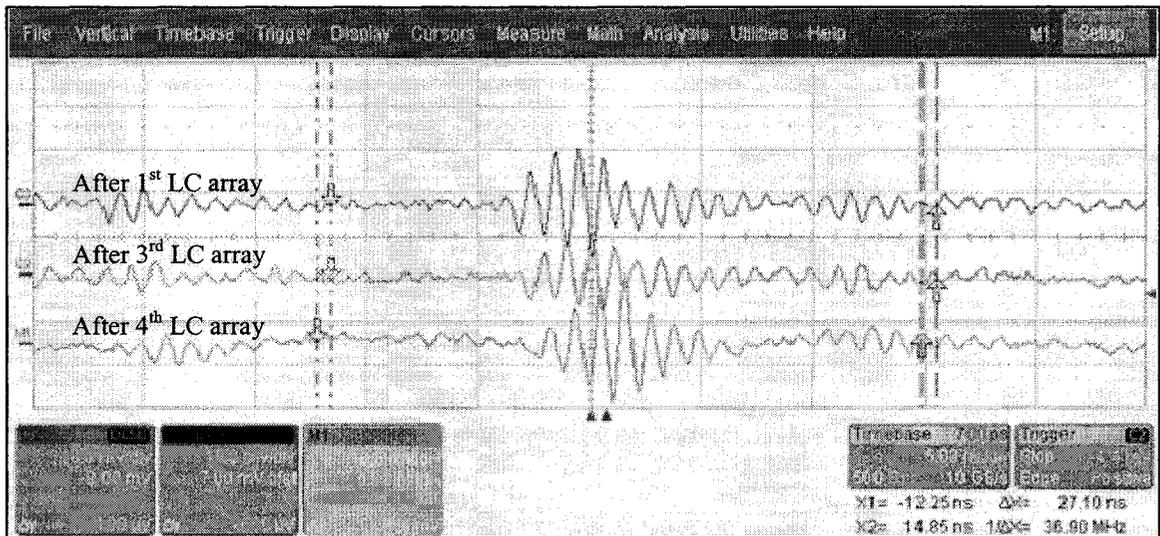
**Figure 5.10 Oscilloscope display showing OOK modulated signal after first, third and fourth LC array of the ID generation circuit (x axis = time (5 ns/div); y axis = voltage (10 mV/div)).**
