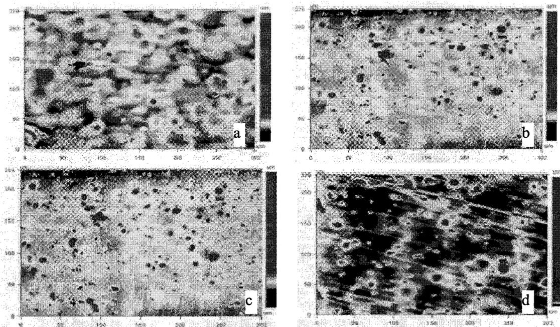
**Figure 3.10 (a) Untreated Kapton VN500 (65  $\mu\text{m}$ ) (b) mechanically roughened (37  $\mu\text{m}$ ) (c) Sensitized with Isopropyl alcohol under sonication (37  $\mu\text{m}$ ) (d) KOH etching for 1 min (15  $\mu\text{m}$ ).**
