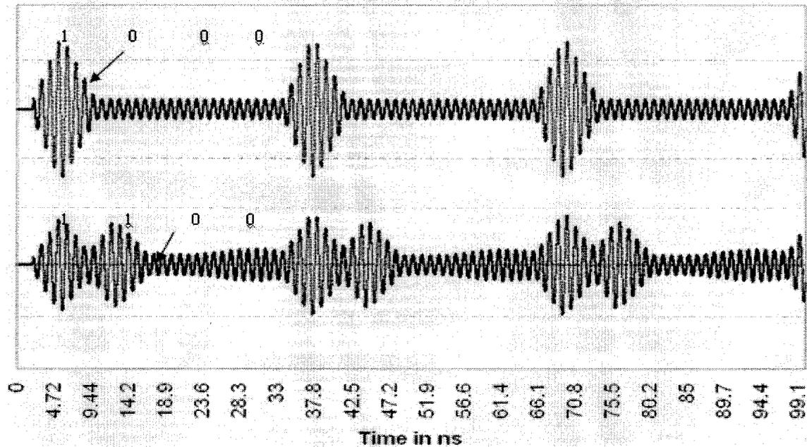
**Figure 6.4 Different bit code generation by ID generation circuits for modulated digital input (x-axis = 4.72 ns/div; y-axis = 0.3V/div voltage).**
