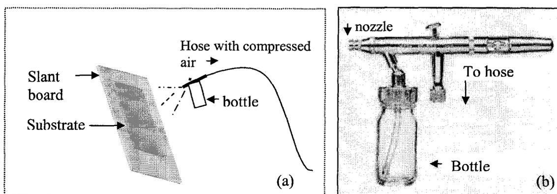
**Figure 3.15 (a) Spray coating experimental set up (b) air brush used for spray coating technique.**
