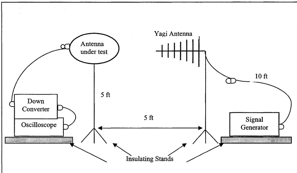
**Figure 5.12 Dimensions and instrumentation of measurement and test setup.**
