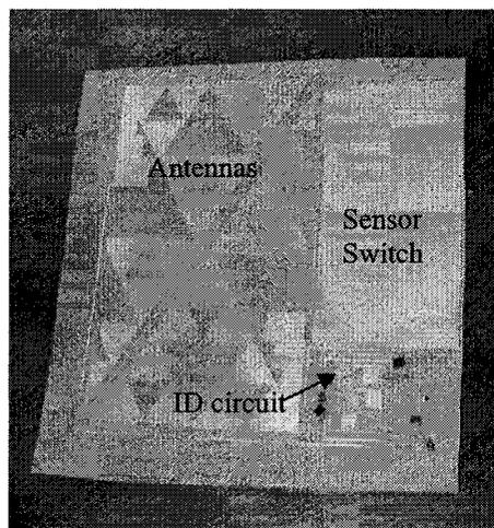
**Figure 5.8 Tag fabricated silicon-based fabrication processes and assembling.**
