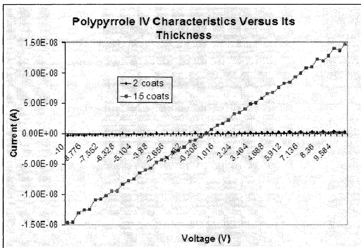
**Figure 3.2 Measured current-voltage characteristics, indicating change in resistance with respect to the number of layers of printed polypyrrole.**
