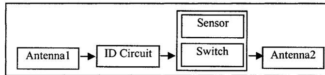
**Figure 2.1 Schematic diagram of wireless sensor tag showing receiving antenna (Antenna1), sensor-switch, ID generating circuit and transmitting antenna (Antenna2).**
