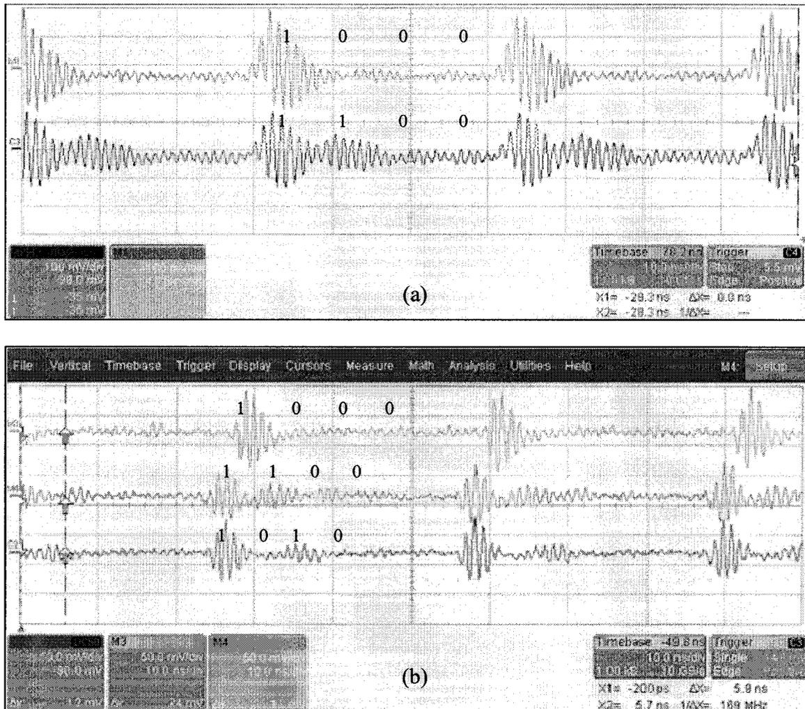
**Figure 6.7** Output waveforms from the ID generation circuit (a) 4 Code generation (x axis = 10 ns/div, y axis= 100mV/div) with 8 ns bit length (b) Codes generated with 4 ns bit length (x axis = 10 ns/div, y axis = 50 mV/div).
