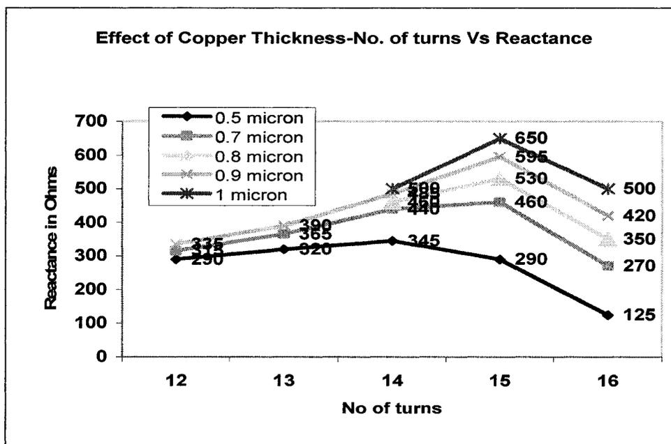
**Figure 4.4 Reactance change in simulated triangular planar inductors with respect to thickness and number of turns.**
