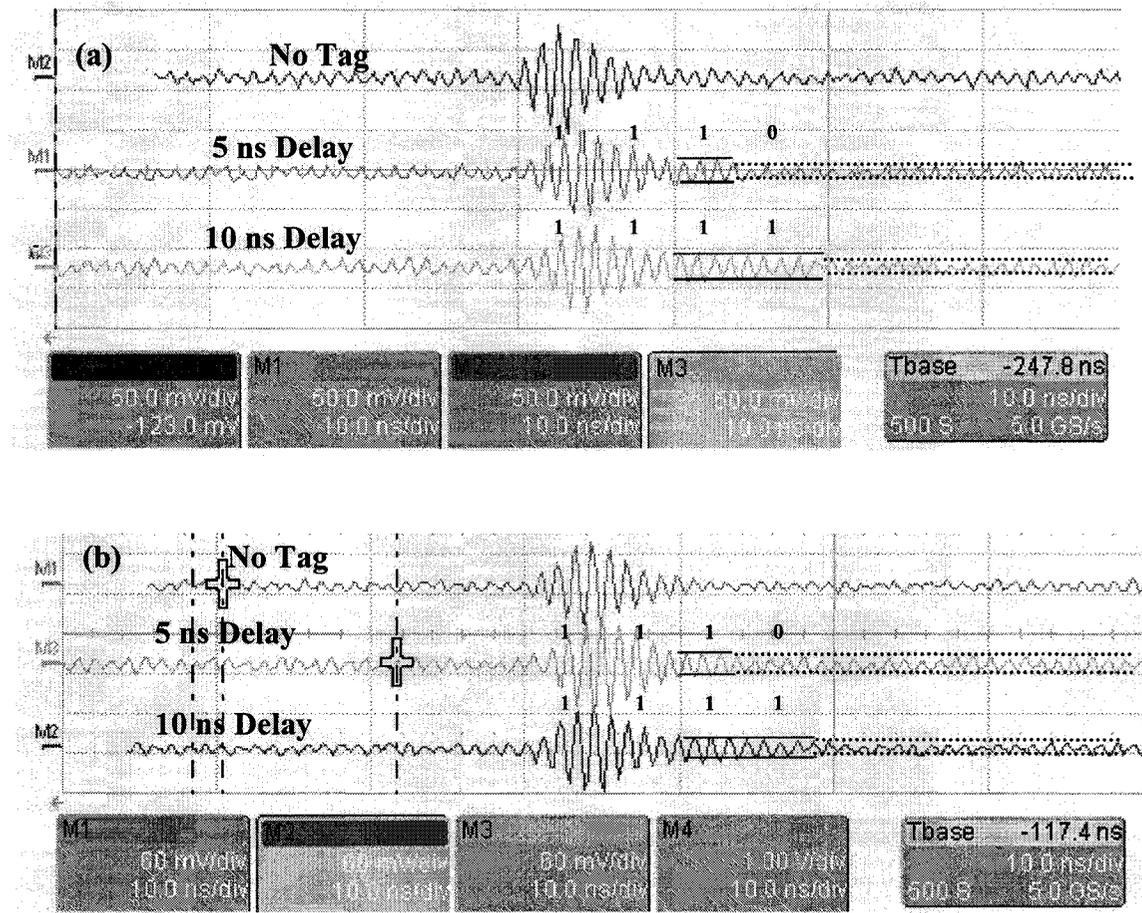
**Fig. 6.21 (a) 5 ns and 10 ns delay deliverable using RFID tag with triangular antenna (b) using RFID tag with spiral antenna.**
