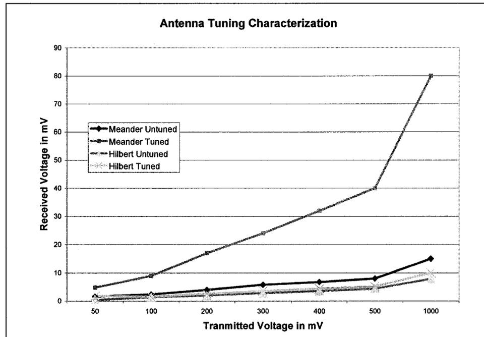
**Figure 5.14 Effect of tuning on Meander and Hilbert antennas.**
