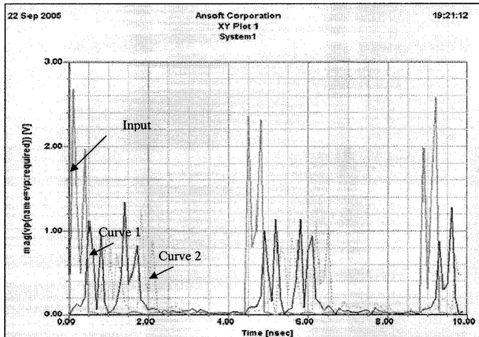
**Figure 6.10 Simulated input and output waveforms at the receiver.**
