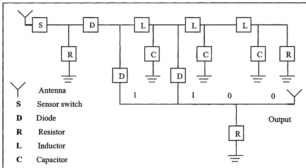
**Figure 2.7 Circuit diagram of LC-delay-line-based RFID/RFID-based sensor [35].**
