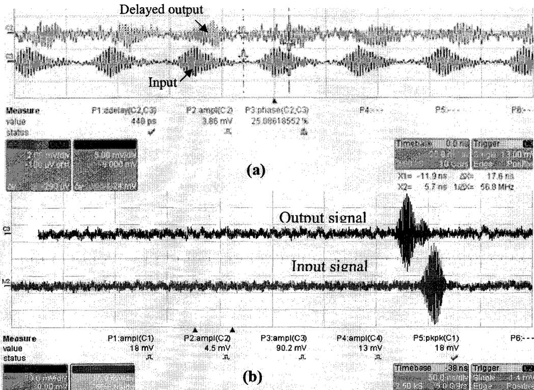
**Figure 6.14 (a) Observed delay in the Meandered and straight branches of the ID generation circuit with the input signal received (b). Measured input and output signals from the tag in receiving mode (for maximum coupled signal).**
