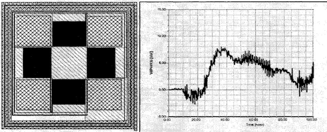
**Figure 7.2 (a) 13.56 MHz LC-delay line based circuit layout and (b) Obtained output from delay lines.**
