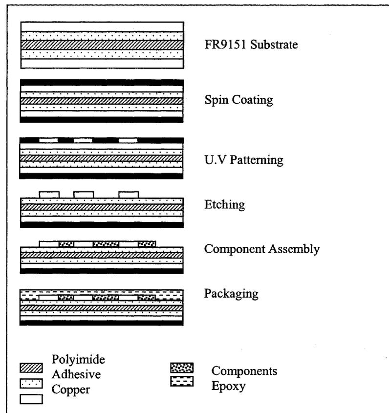
**Figure 3.21 Schematic diagram showing the process steps used in the fabrication of piezoelectric RFID tag.**
