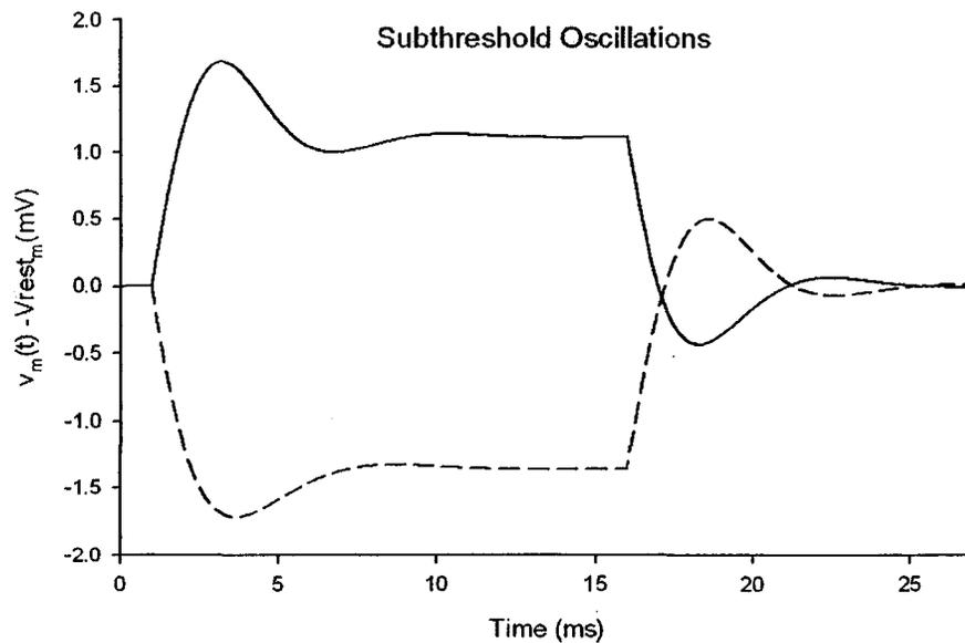
Figure 8.13. Subthreshold oscillations device model results—comparison with Weiss, page 233, figure 4.61.
