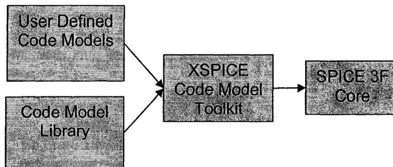
Figure 5.1. Graphical Representation of XSPICE Code Model toolkit implementation in SPICE.
