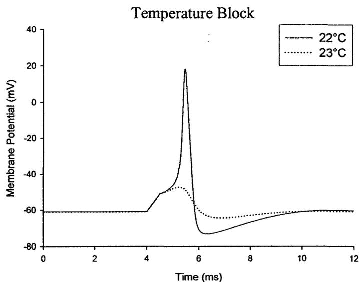
Figure 8.15. Device model results showing the thermal block between 22°C and 23°C.
