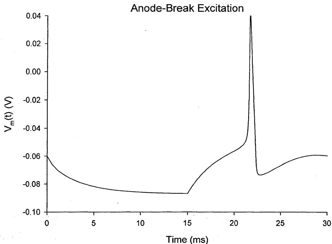
Figure 8.9. Anode-break device model results—comparison with Weiss, page 230, figure 4.59 (graph provided in appendix C).
