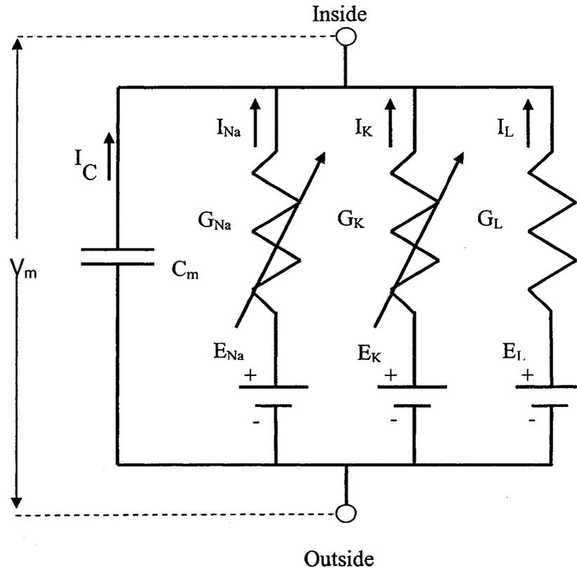
Figure 4.1. The Hodgkin-Huxley equivalent circuit diagram depicting a patch of a neuronal cell membrane in terms of ionic conductances ( $G$ ), current densities ( $I$ ), ionic potentials ( $E$ ) and membrane capacitance ( $C_m$ ).
