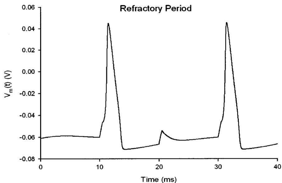
Figure 8.7. Device model results for the Basic refractory period simulation completed using the netlist in figure 8.5.
