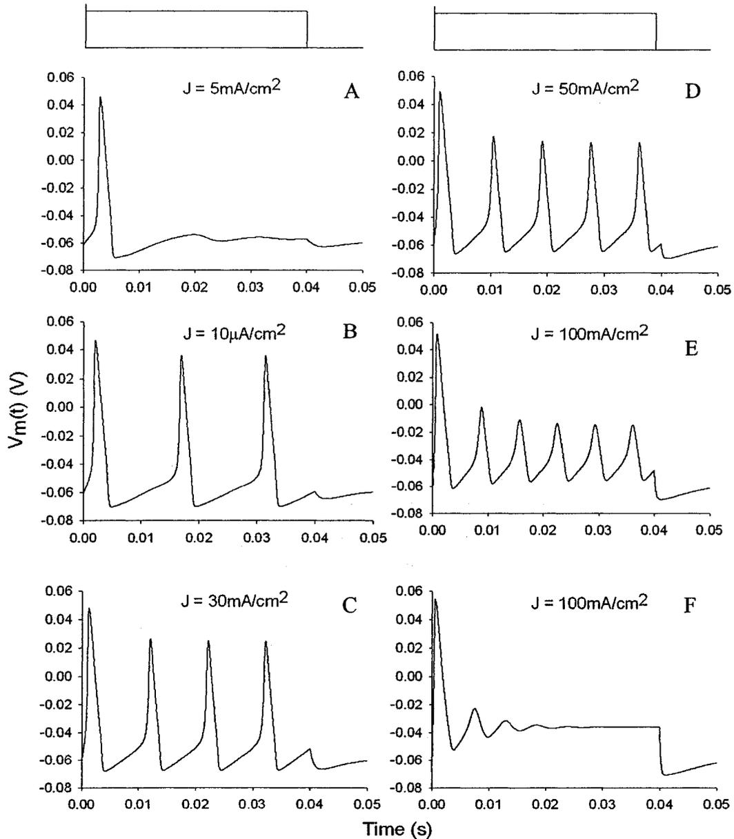
Figure 8.3. Actual device model results showing action potential repetitive activity using different current injections over a 40 ms time period—comparison with Weiss, page 232, figure 4.60 (graph provided in appendix C).
