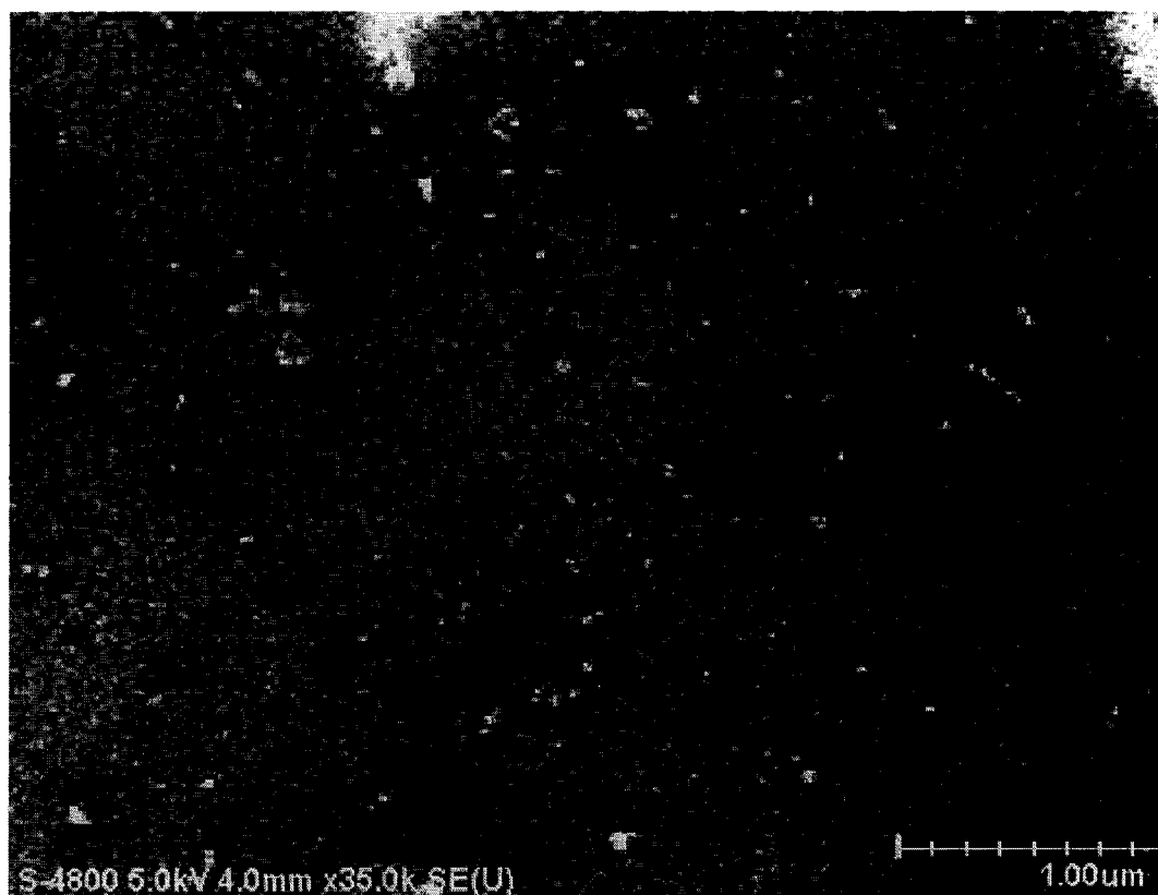
Figure 3.5 SEM micrograph for indium nanoparticles from reduction of \{[\text{HB}(3\text{-phpz})_3]\text{In}\}
