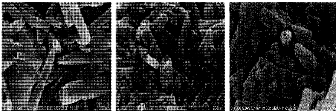
Figure 7.1: SEM images of unloaded empty halloysite. Images were taken after sputter coating the dried sample with 2 nm thickness of Iridium.
