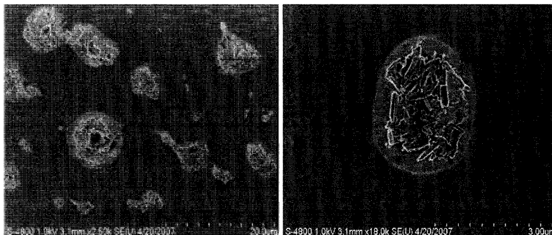
Figure 3.10 SEM images of Curcumin loaded chitosan-alginate particles. Images were taken after sputter coating the dried sample with 2 nm thickness of Iridium.
