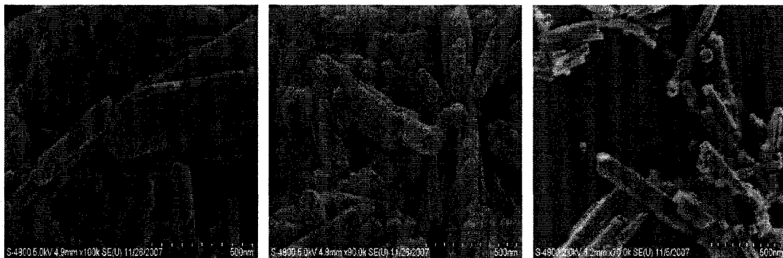
Figure 7.4: SEM images of silver nanoparticles prepared by reducing silver acetate by normal light in the presence of lysozyme. Images were taken after sputter coating the dried sample with 2 nm thickness of Iridium.
