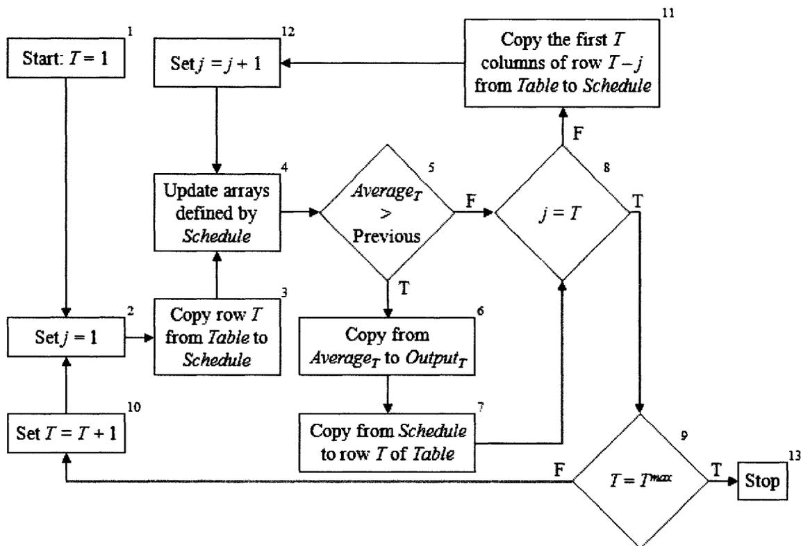
Figure 2 Flowchart of software logic.
