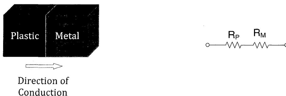
Figure 2.9: Series Connected Plastic and Metal with Equivalent Circuit Model
