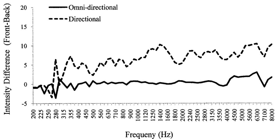
Figure 4 SPL difference between the front and back response for the omnidirectional and directional microphone conditions for all left ears.
