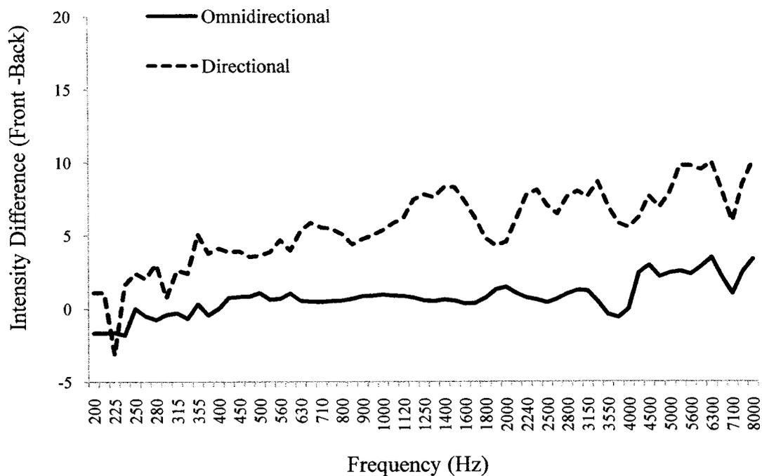
Figure 3 SPL difference between the front and back response for the omnidirectional and directional microphone conditions for all right ears. Note: Difference was calculated by subtracting front response from the back response.
