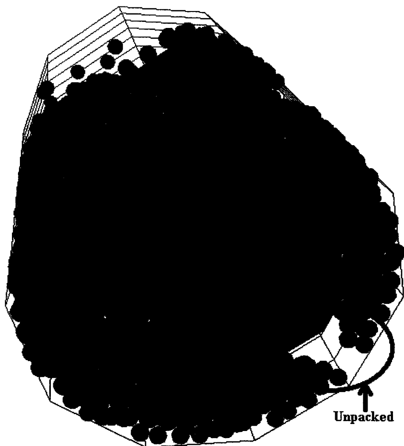
Figure 4 5 Graphical representation of a packed pore obtained from the implementation of the sectoring method
