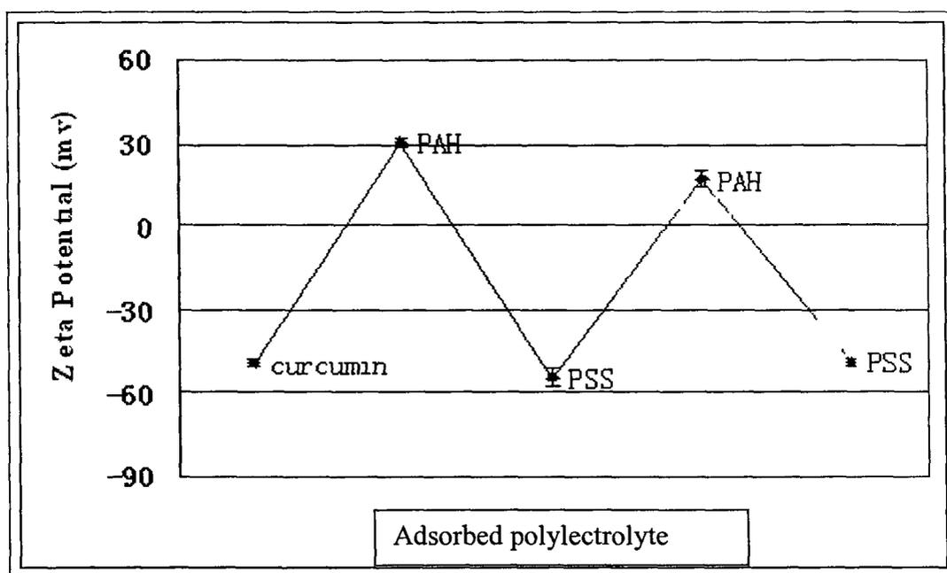
Figure 4-3  $\xi$ -potential alternation during LbL-shell formation of cationic PAH and anionic PSS on curcumin nanoparticles. Standard deviation shows the same sample run 10 times on zeta potential analyzer.
