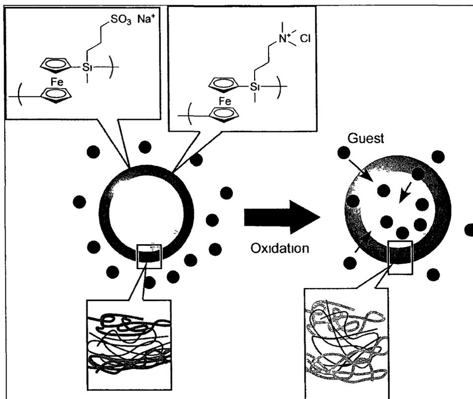
Figure 2-4 Organometallic polyelectrolyte multilayer microshells, composed of polyanions and polycations of poly(ferrocenylsilane)
