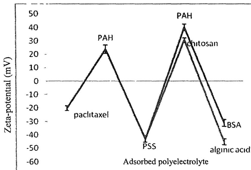
Figure 4-6  $\xi$ -potential of paclitaxel coated with two different bilayers of PAH-PSS-PAH-BSA and PAH-PSS-chitosan-alginate acid (using top-down approach). Standard deviation shows the same sample run 10 times on zeta potential analyzer.
