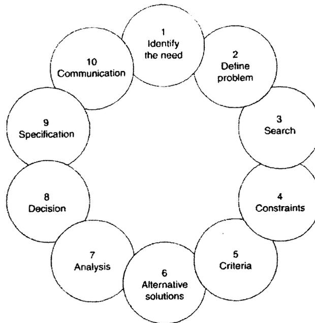
Figure 2-2: Illustration depicting the engineering design process as seen in the textbook *Engineering Fundamentals and Problem Solving* [24].
