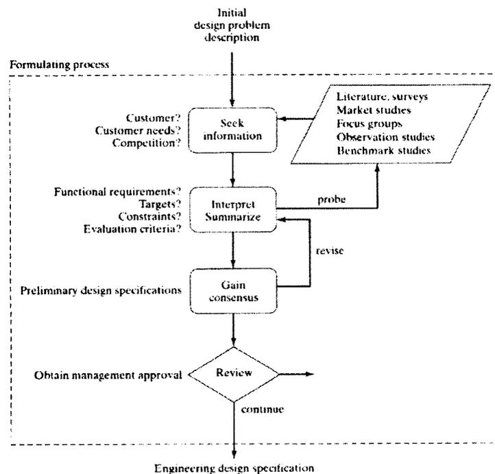
Figure 2-5: A flowchart identifying the formulation phase of the engineering design process [23].
