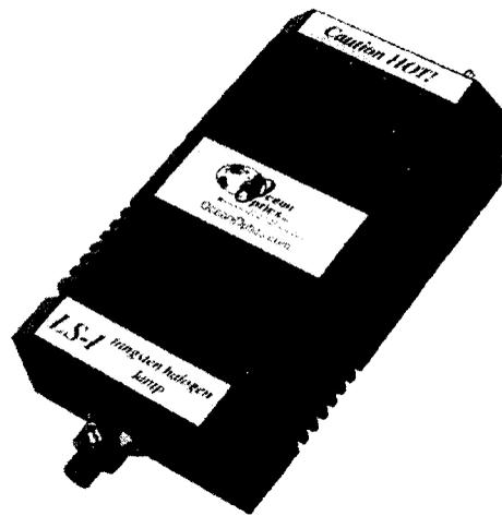
Figure 2.7 Photograph of a white-light source.
