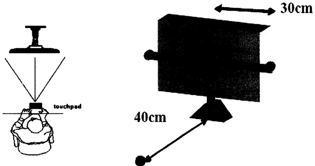
Figure 19: The experimental setup is illustrated. Touch pads (circles) are placed at the base (resting) position and at the targets of the reaching tasks (left, right, and forward) to track whether the subject has performed the tasks correctly.
