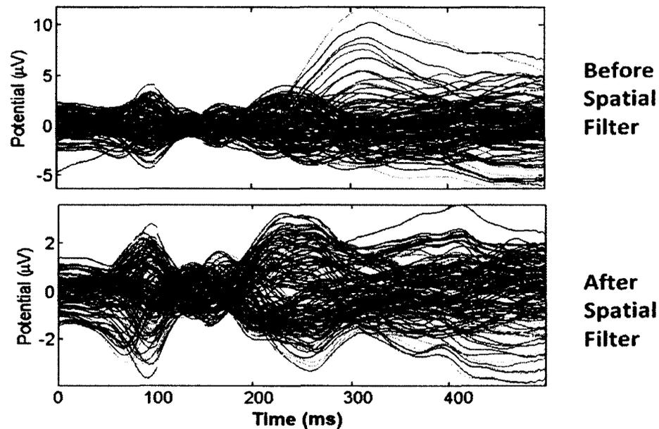
Figure 24: EEG signals before and after spatial filtering is shown. The signal for each channel is averaged across all trials prior to ICA spatial filtering. An example of eye artifact is seen in the EEG spatial map around 305ms. After eye artifact is removed, the averaged signal for each channel after ICA spatial filtering is shown at the bottom subplot.
