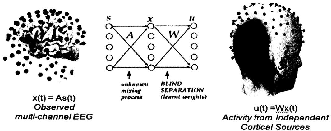
Figure 8: A Spatiotemporal Filter for extracting activity from multiple cortical sources.
