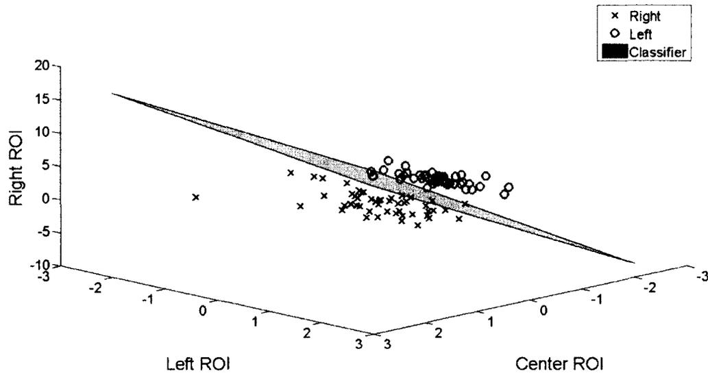
Figure 31: Scatter plot of EEMD-based features for left and right intended movement separated by FLD classifier.
