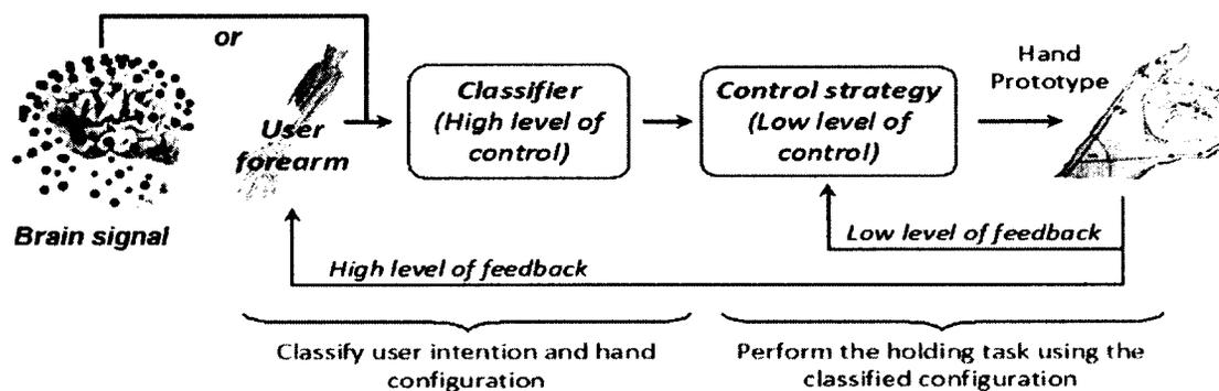
Figure 2: The classical (EMG based) and the new (brain wave) control of prosthesis.
