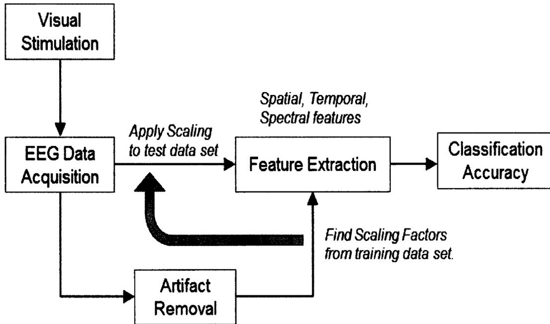
Figure 18: A flow chart describing overall experimental procedure for decoding the reaching tasks during the planning stage. The visual stimulation was provided to subjects for recording EEG signals. Artifact in the data was removed before finding the suitable scaling factors. Once the scaling factors were obtained, they were applied to the signal amplitude features in the test set. To determine the overall accuracy, a 5x5-fold cross validation procedure was performed for a binary classifier.
