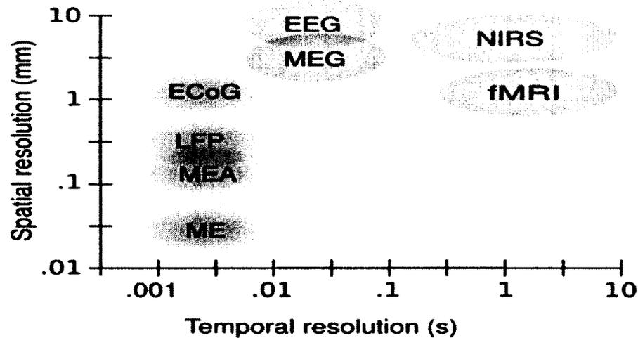
Figure 7: Overview of the scale of spatial and temporal resolution of measurement methods used for BCI. Non-invasive methods are shown in blue and invasive methods are shown in red [11].
