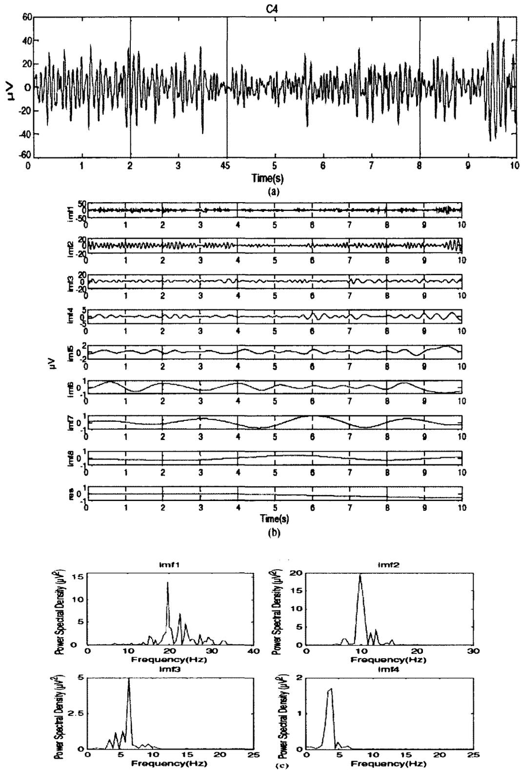
Figure 15: Illustration of the characteristic IMF extraction. (a) The single-trial EEG data at C4 during the imagination of the combined left-foot with left-hand movement. (b) The EMD results of (a). (c) The PSD distribution of the first four IMFs in (b) [25].
