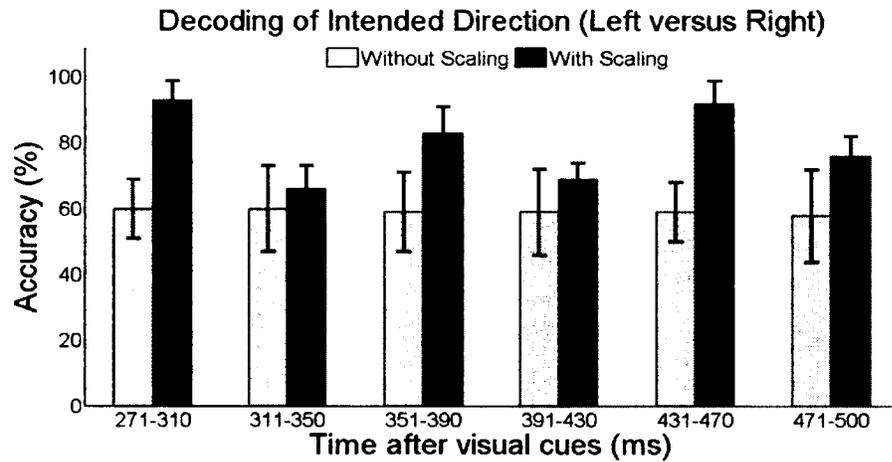
Figure 30: EEG amplitude features obtained in the PPC regions can be used to classify the intended direction of reaching motion. Classification accuracy is at the highest using amplitude features 271-310 ms after the presentation of the visual cues.
