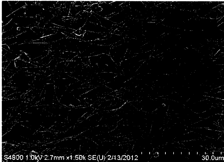
Figure 48: SEM image of nanowire GMR thin film on PET substrate
