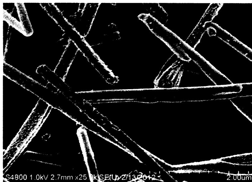
Figure 49: Closer view of nanowire GMR thin film on PET substrate
