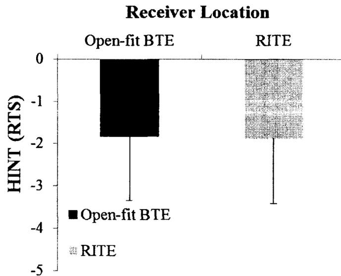
*Figure 4.* Mean HINT with noise generated from the front loudspeakers (in SNR) for the open-fit BTE and RITE devices.
