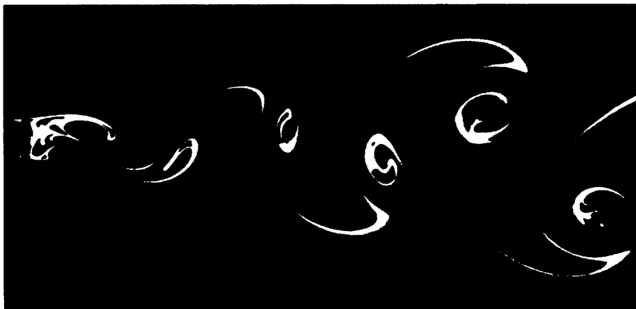
Figure 6-4: SPH simulation of Vortex Shedding: Von Kármán vortex street behind a circular cylinder at Reynolds number 140, photographed by Sadatoshi Taneda [89].
