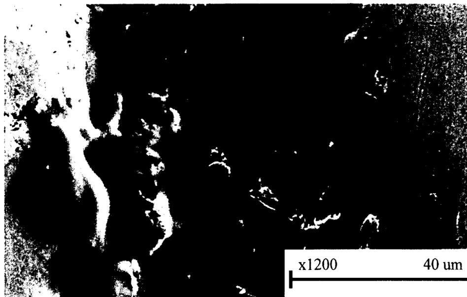
Figure 65. Scanning electron microscope image of an electrochemically treated fatigue crack within 5 mm of the crack tip.
