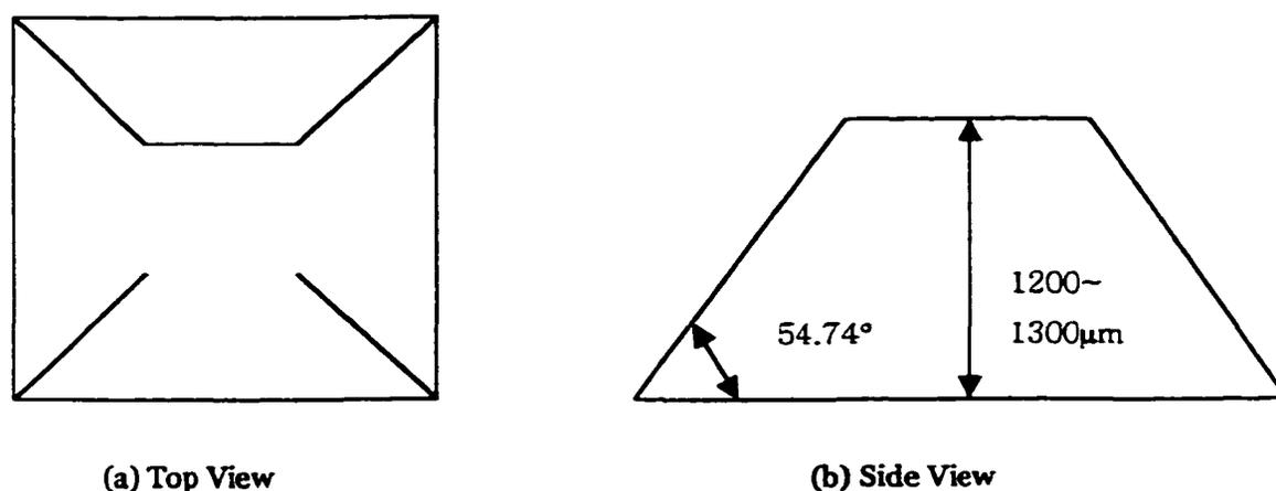
Figure 2-1. Diagrams for Mirrors
