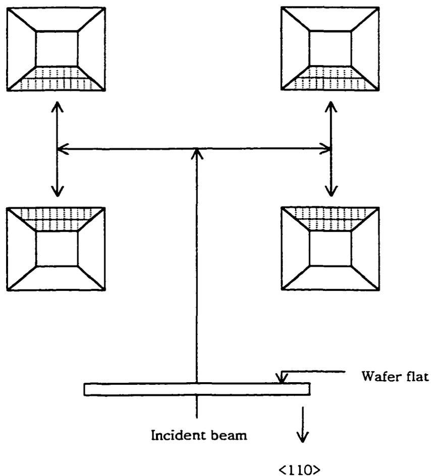
**Figure 2-13.** Direction of Incident Beam to  $45^\circ$  Mirrors
