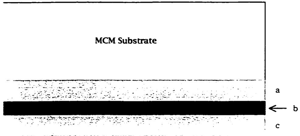
Figure 1-4. Silica Glass Waveguide Layers (a: Upper Buffer Layer, b: Core of The Waveguide, c: Under Buffer Layer).
