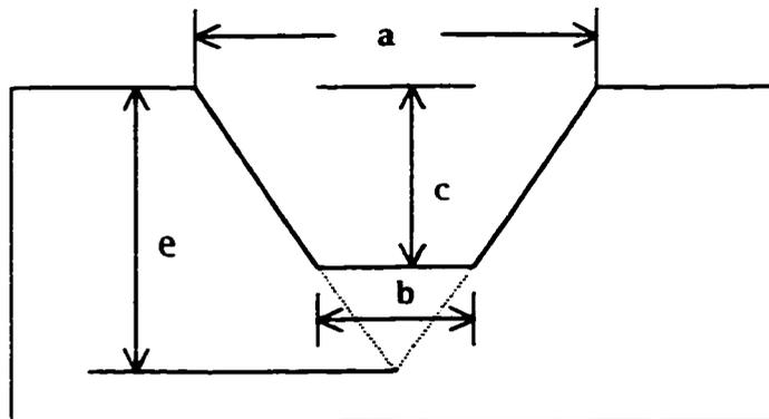
Figure 2-8. Geometry of an Etched Pit
