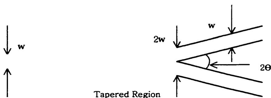
Figure 3-9. Y-Branching Waveguide Structure.
