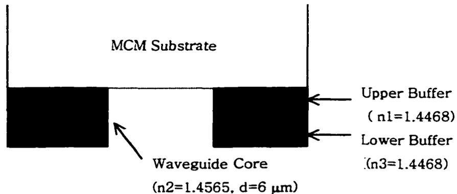
Figure 3-1. Silica Glass Waveguide Substrate
