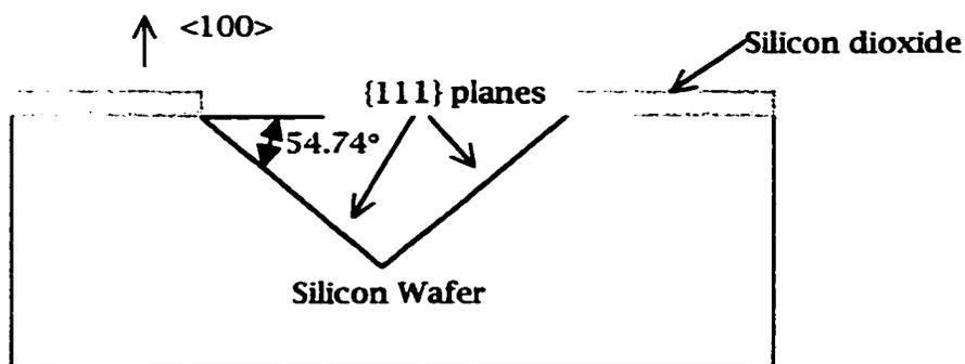
Figure 2-7. Micromachined Silicon Substrate
