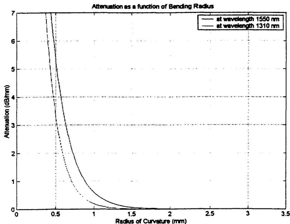
Figure 3-7. Attenuation as a Function of Bending Radius
