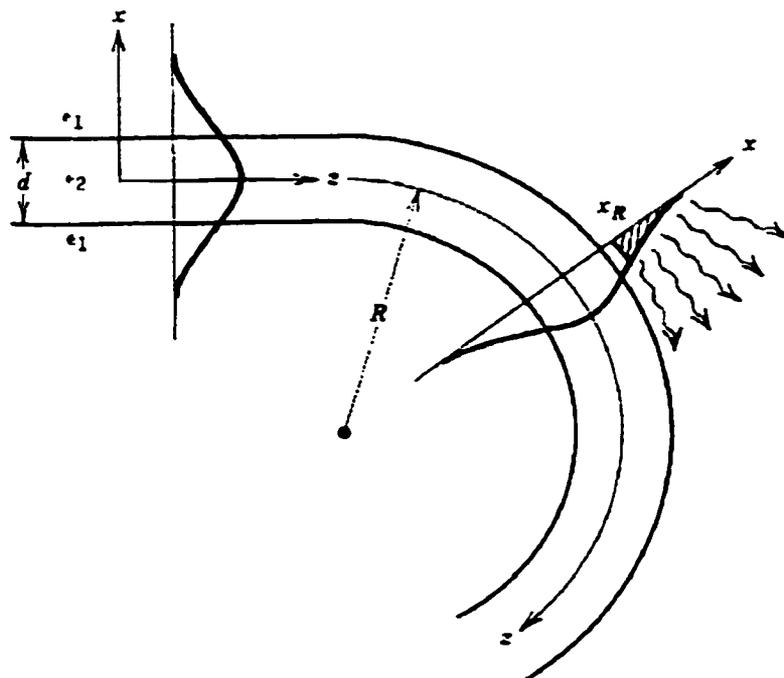
Figure 3-5. Bending Section of the Waveguide [58]
