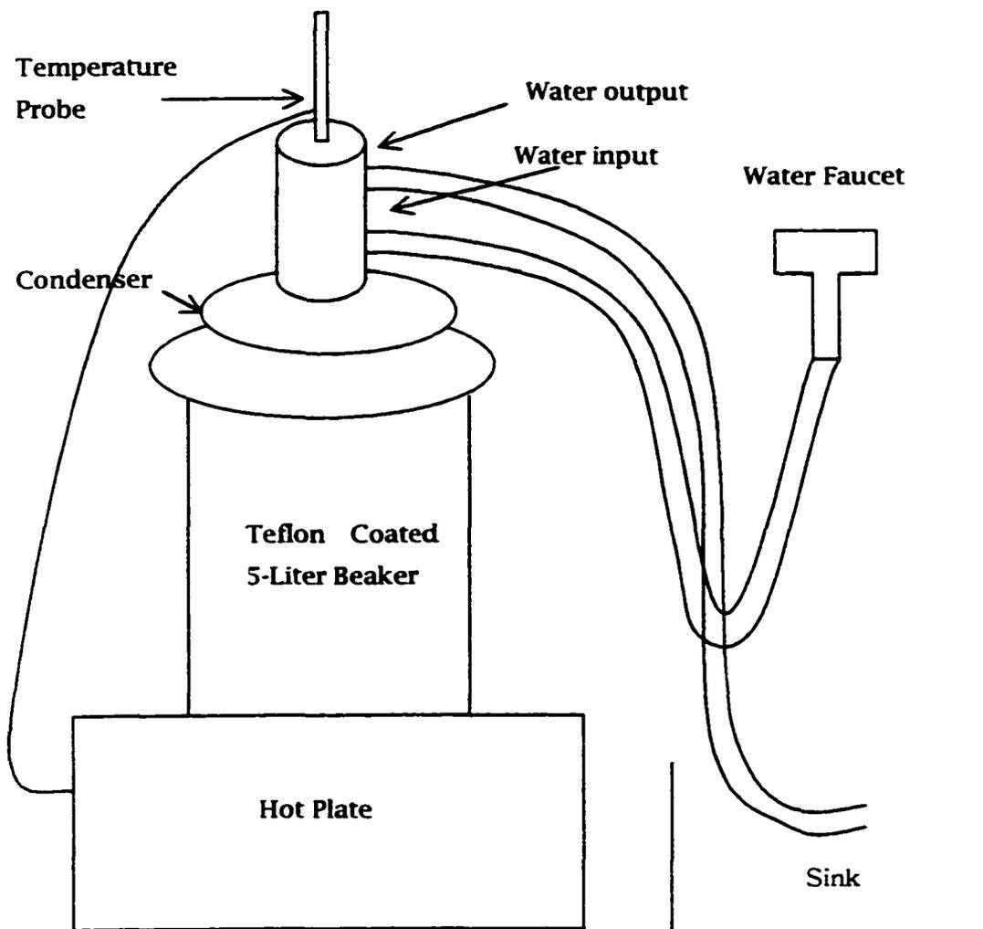
**Figure 4-4 Anisotropic Etching System**
