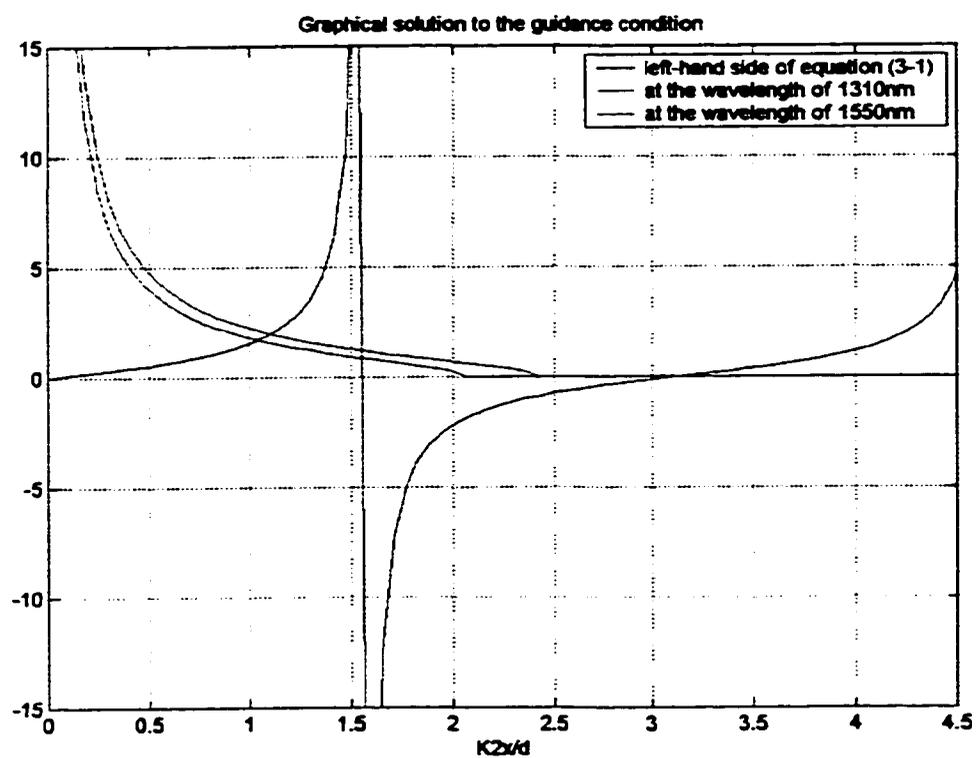
Figure 3-3. Graphical Solution of the Guidance Condition
