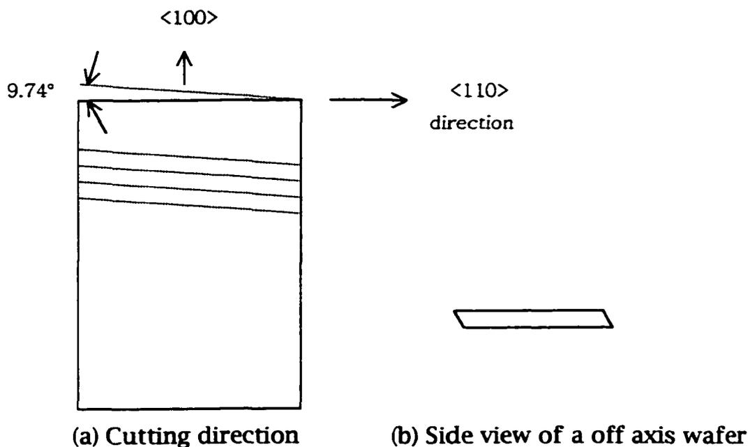
Figure 2-11. Geometry of Off Axis Silicon Wafer
