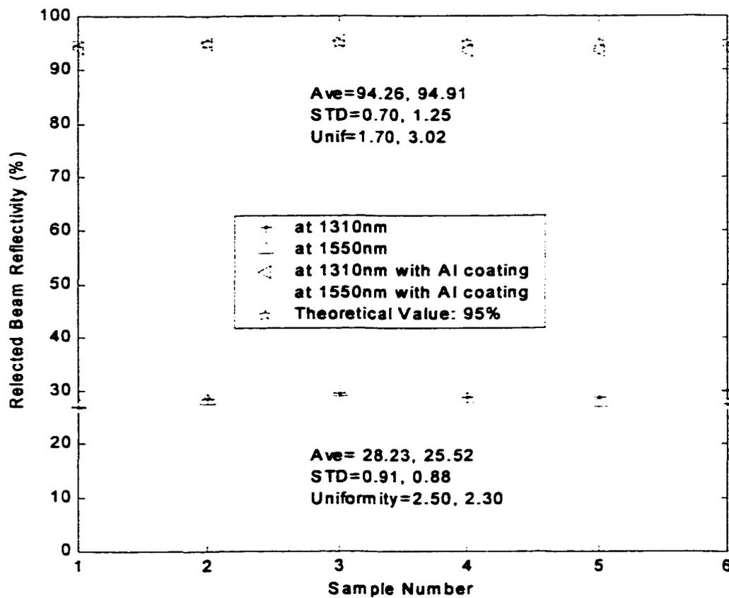
**Figure 4-6. Beam Reflectivity of Silicon Mirror**
