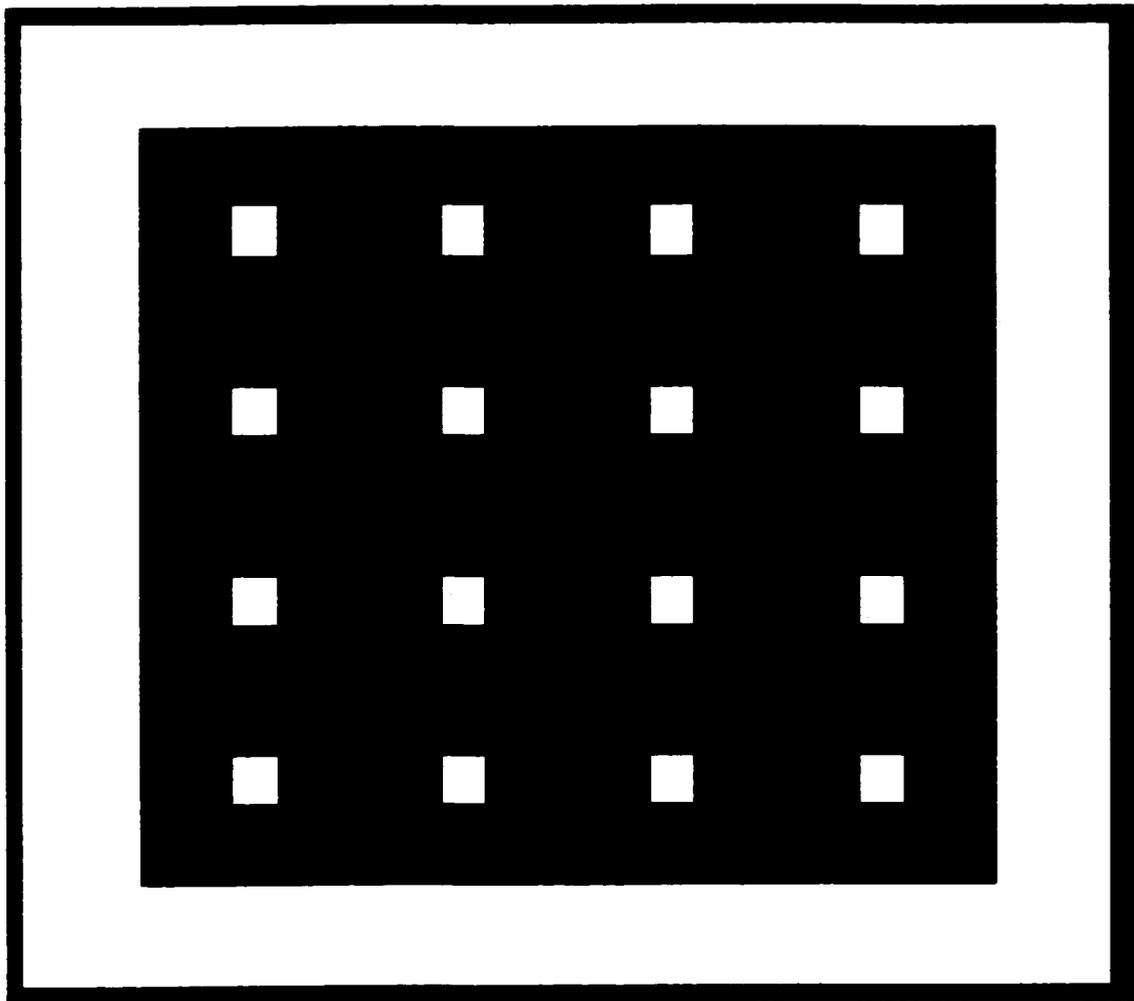
**Figure 2-10. Mask Layer for Sixteen Through-Holes**
