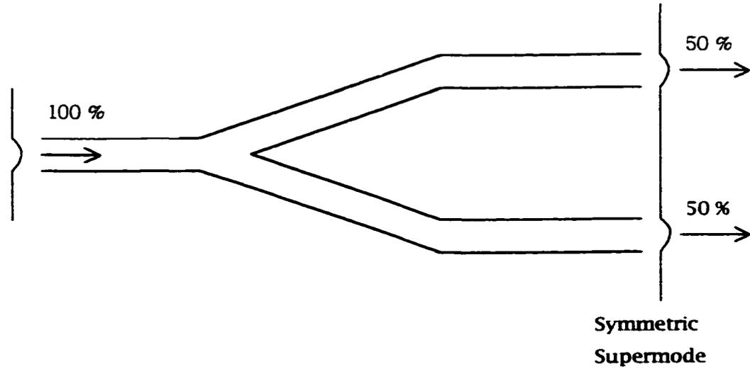
Figure 3-11. Excitation of a Y-Junction at the Left End [62]
