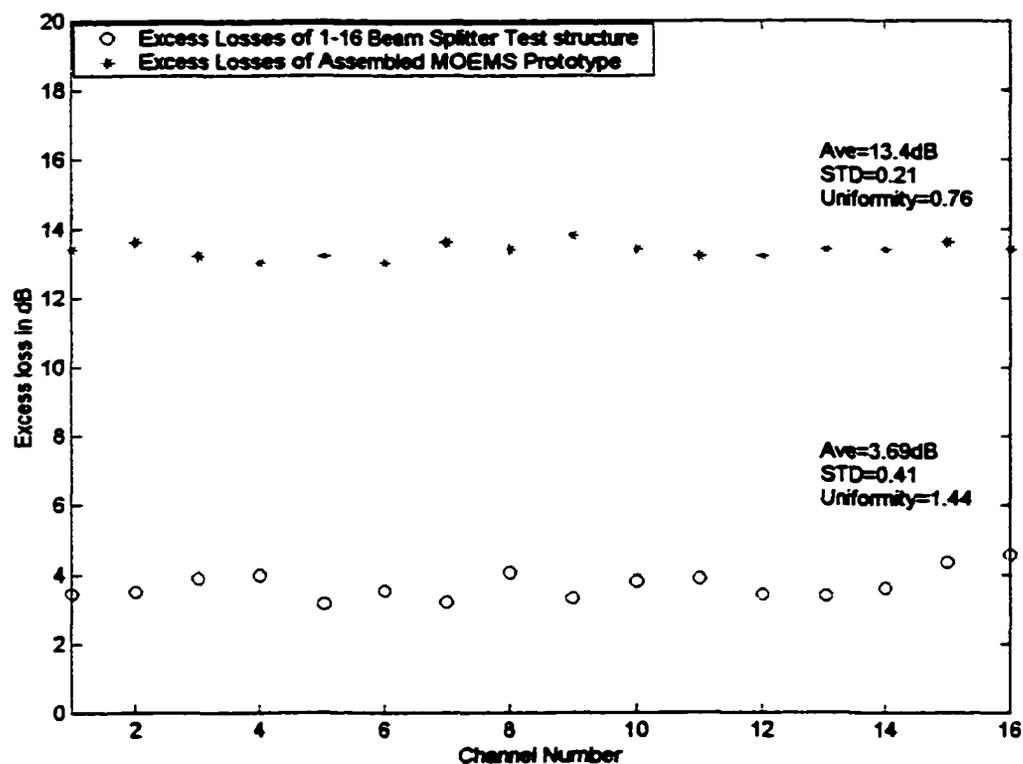
Figure 5-1. Excess Losses at Sixteen Fan-Out Nodes
