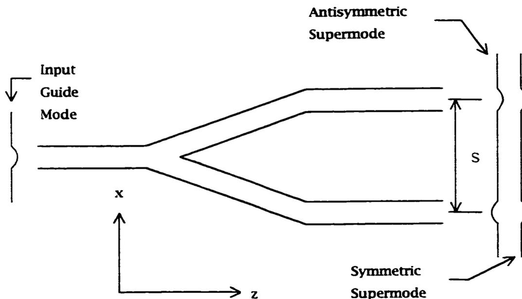
Figure 3-10. Characteristic Modes of a Symmetric Y-Junction [62]
