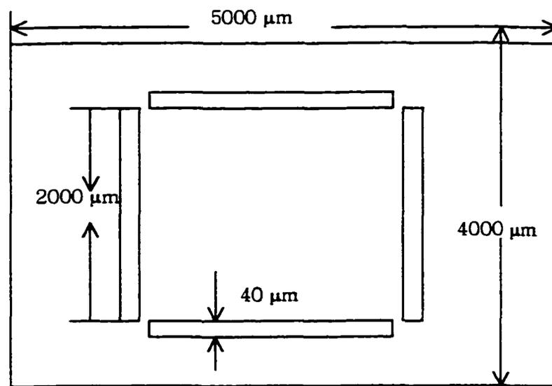
**Figure 2-9. Mask Layer for Through-Holes**
