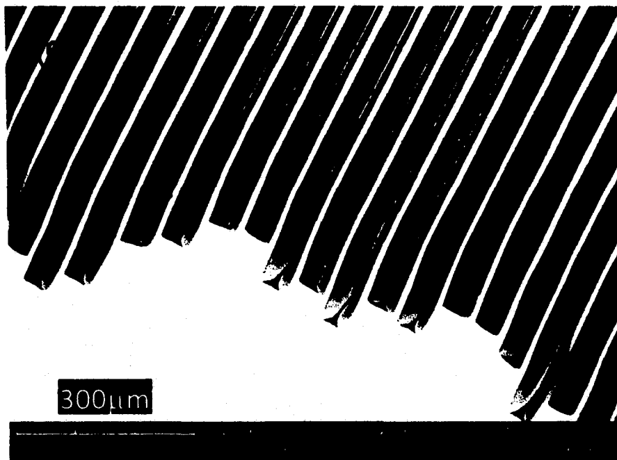
Figure 3-7d: The assembly quality of the nanowires with PAN solutions of various concentration: 10 %, The N 2 gas flow was fixed at ~1.0 ml/h.
