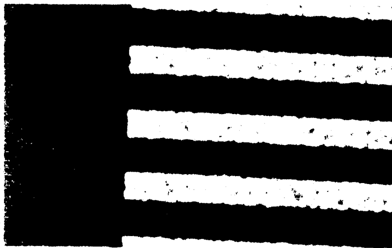
Figure 3-3: An optical microscopy image of the fabricated micropatterns on a silicon wafer.
