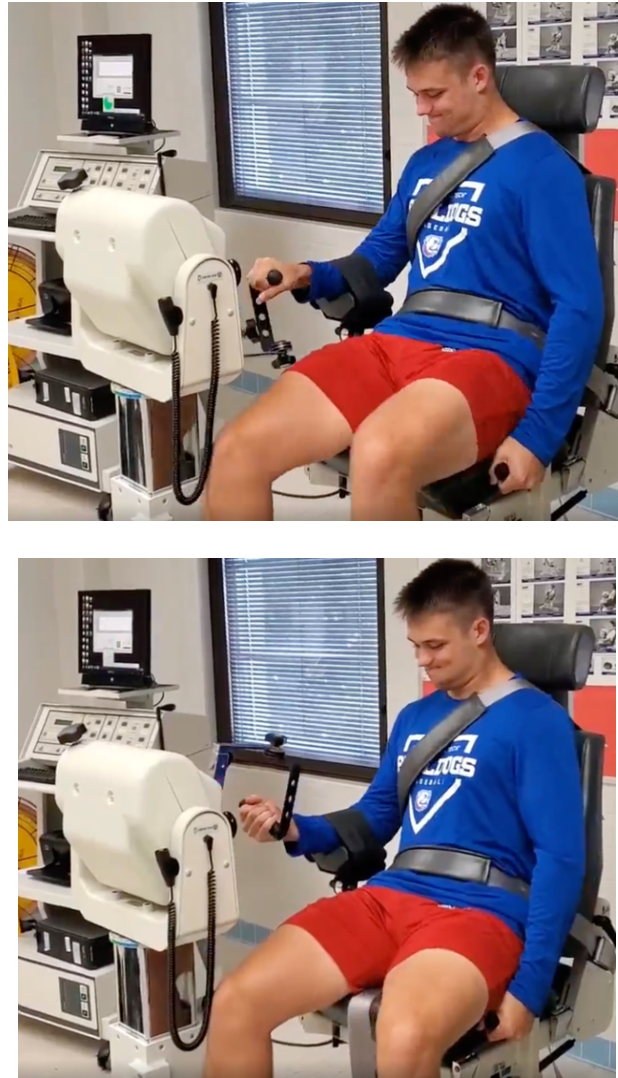
Figure 2. The seated Biodex isokinetic dynamometer forearm pronation (left) and supination (right) test.
