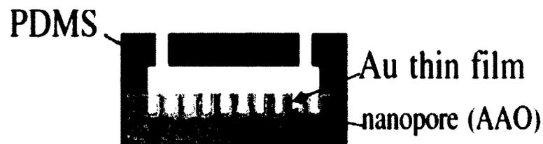
Figure 5-3. Cross sectional view of the PDMS microchannel attached to gold coated (Au) AAO nanopore thin film [38].
