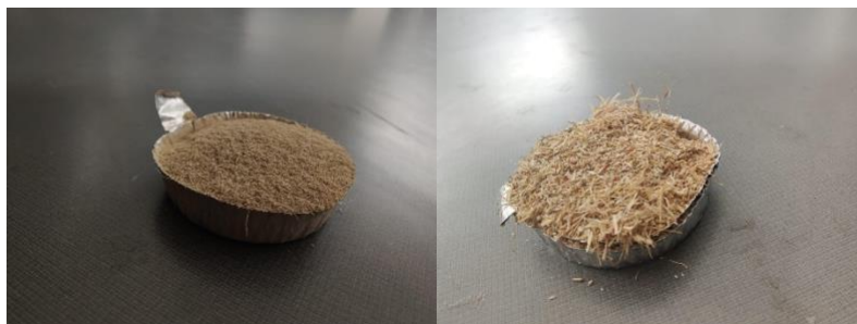
Figure 3-2: CS of particle size 180 \mu\text{m} (LEFT) and particle size 710 \mu\text{m} (RIGHT).
