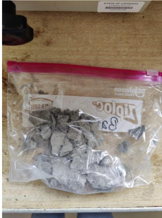
Figure 3-10: Samples after compression test.
