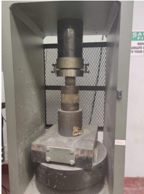
Figure 3-9: Hydraulic compression test machine used for testing compressive strength.
