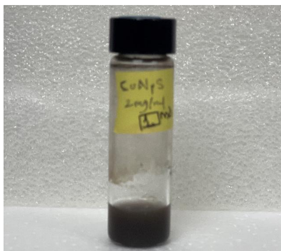
Figure 2-1-1: Vortexed CuNPs stock solution 2mg/ml.
