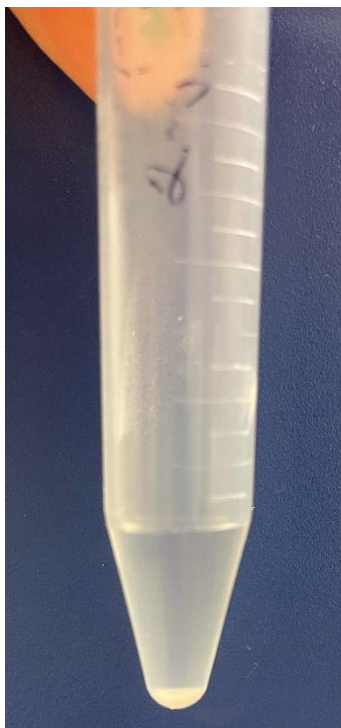
Figure 2-5-1: Silicon dioxide nanoparticles in suspension.
