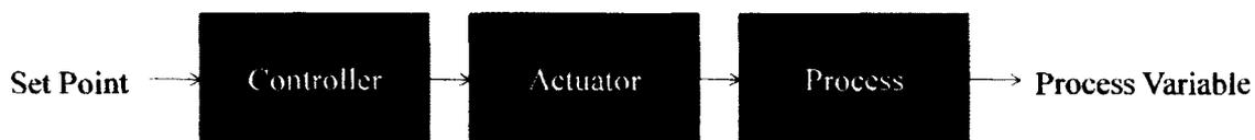
Figure 2.1 Open Loop Control System
