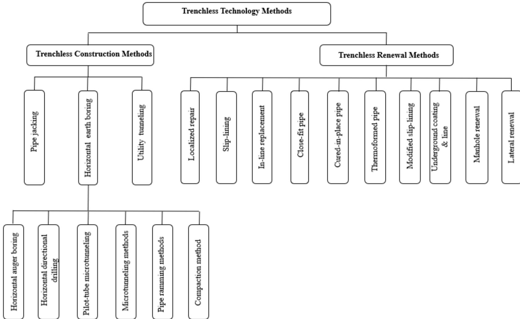
Figure 2-1 Pipeline Construction Methods (Trenchless Technology Methods)
