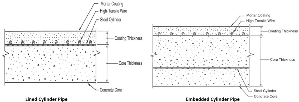
Figure 3-2 Schematic Shows the Different in Wall Cross Sections Between LCP and ECP Pipe (AWWA C304-14)
