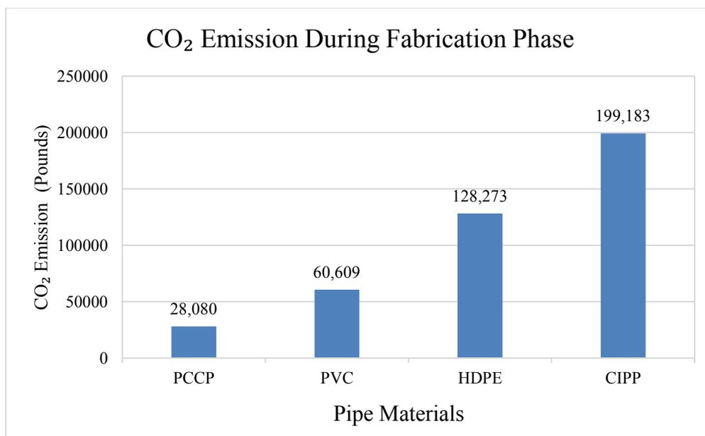
Figure 3-6 CO<sub>2</sub> Emission During the Fabrication Phase
