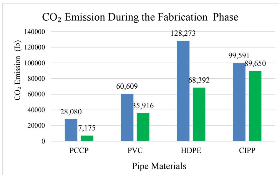
Figure 6-5 Shown the Difference Between the Pipeline Materials During the Fabrication Phase Before and After the Optimizing
