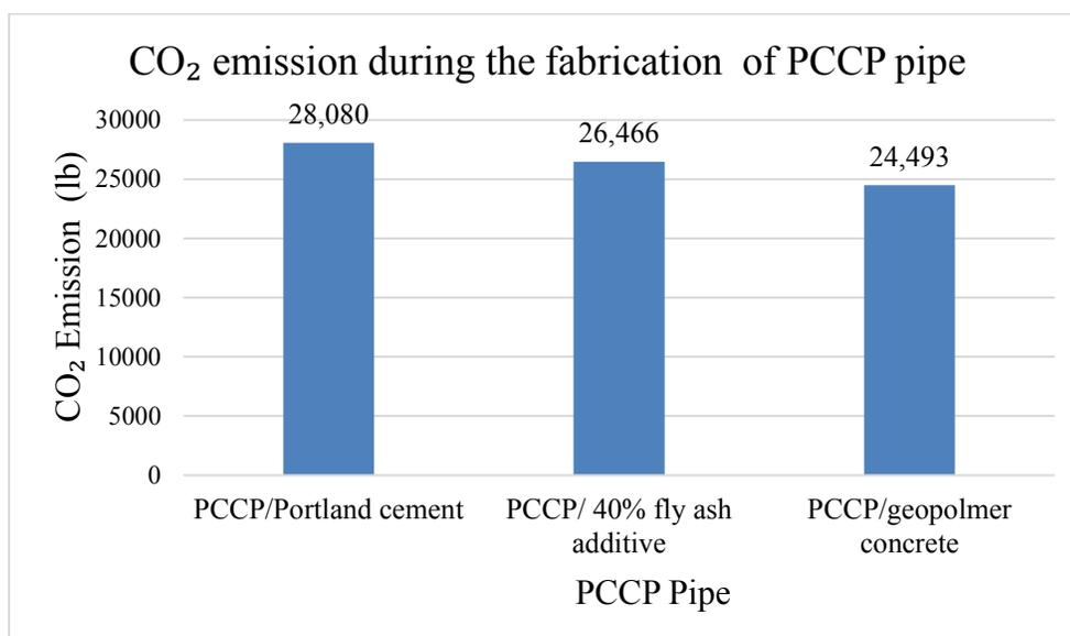
Figure 6-2 Comparing the CO<sub>2</sub> Emissions by Using Portland Cement, Fly Ash and Geopolymer Concrete During the Fabrication Phase of PCCP Pipe
