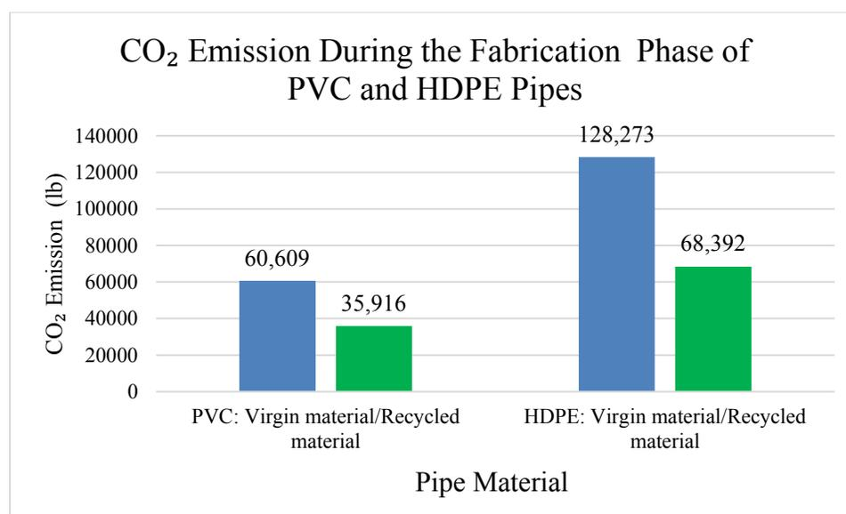
Figure 6-3 Comparing the CO<sub>2</sub> Emissions Between Virgin VS. Recycled Materials for PVC and HDPE Pipes
