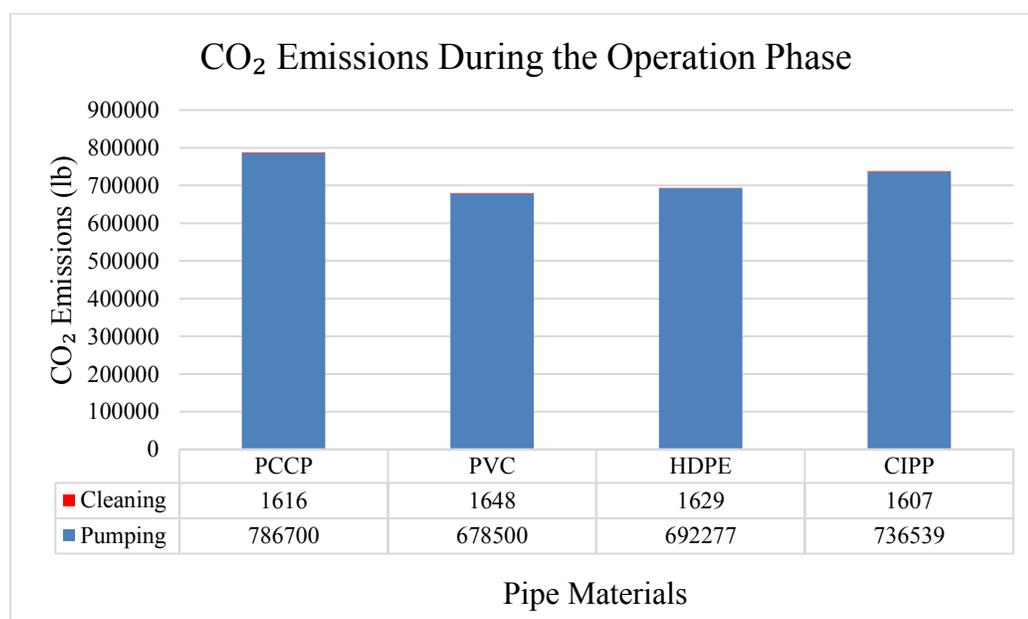
Figure 5-2 CO<sub>2</sub> Emissions During the Operation Phase
