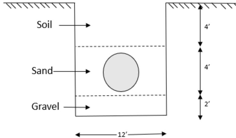
Figure 4-5 Pipeline Backfill Materials
