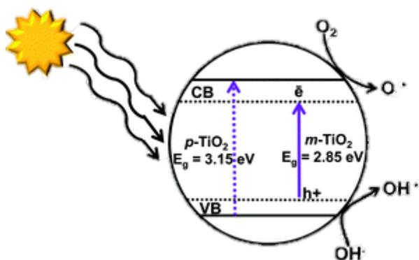
The semiconductor  $\text{TiO}_2$  works because of its energy bandgap and reaction of molecules.
