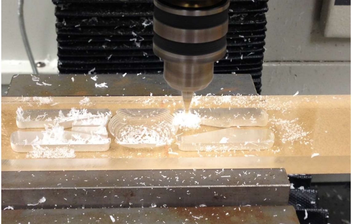
Figure 5-8: Milling the Basket from PC Stock. Smallest bit available 2mm diameter. Some features larger due to milling bit size.
