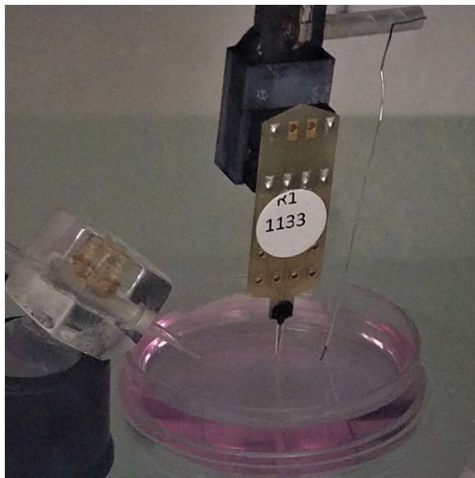
Figure 7-2: Environment and Sensor Arrangement. Sensor immersion into fluid, covering all four sites; centered in dish. Does not touch bottom of dish. Reference pictured to right. Dropper pictured left.
