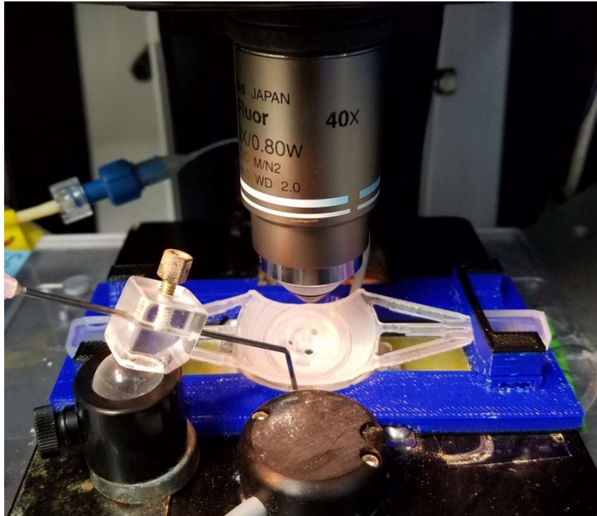
Figure 5-9: PICS Setup on Microscope Stage. Ample room for PICS underneath objective.
