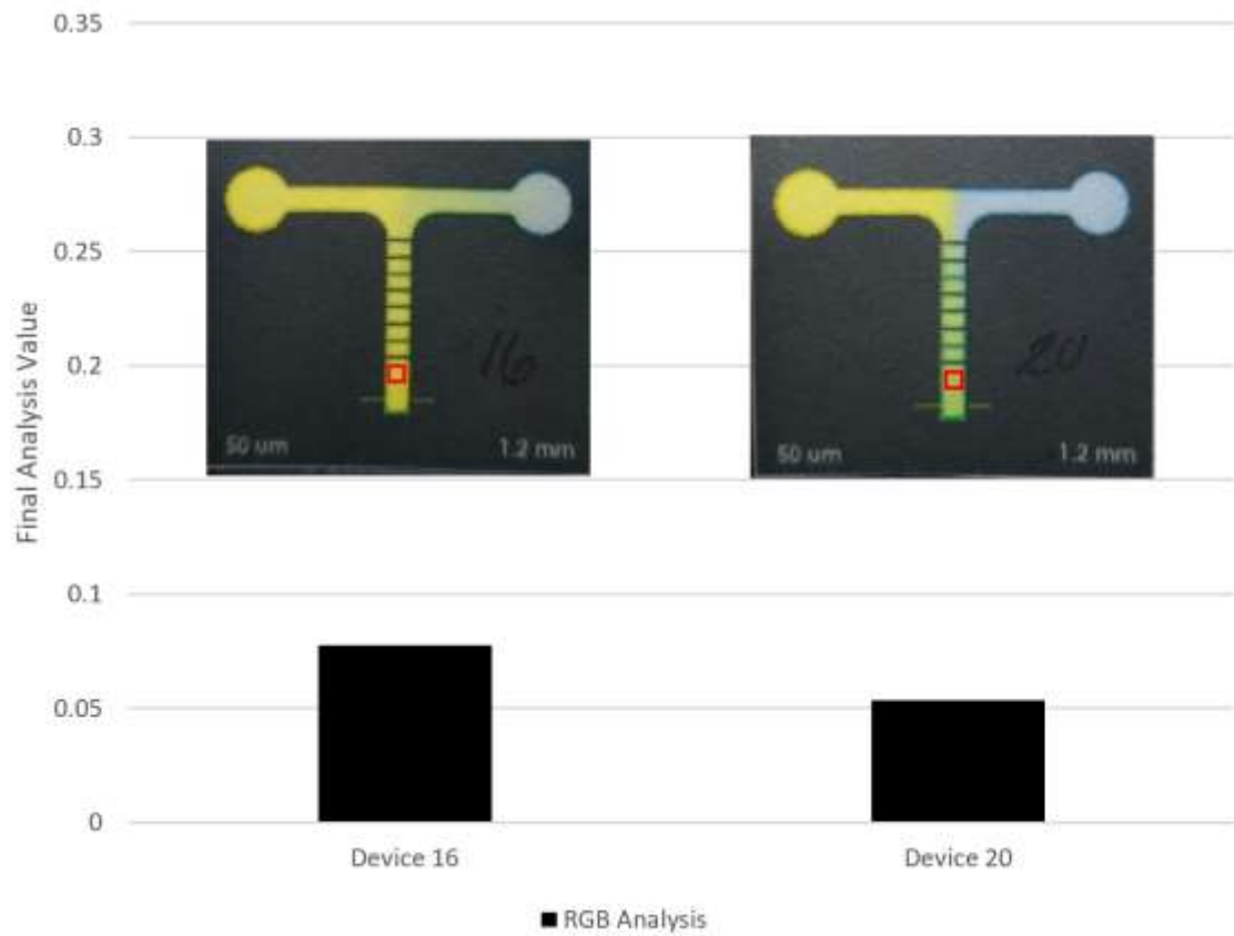
Figure 3-5: RGB analysis of a device with a test region that is qualitatively yellow and a device with a test region that is qualitatively green to show that the RGB analysis does not significantly distinguish the yellow regions from the green regions.
