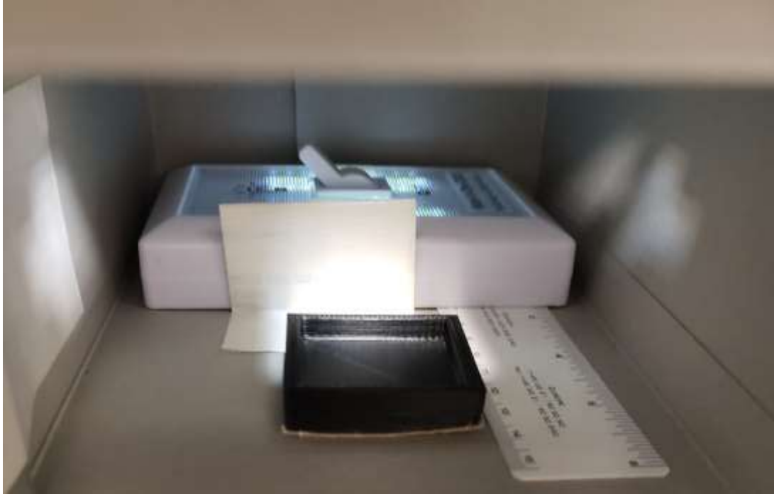
Figure 3-3: Image of the inside of the light controlled box with the 3D printed device holder and ruler for scale.
