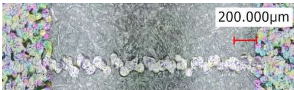
Figure 6-1: Laser Scanning confocal microscope image of a wax printed line in a paper-based microfluidic device.
