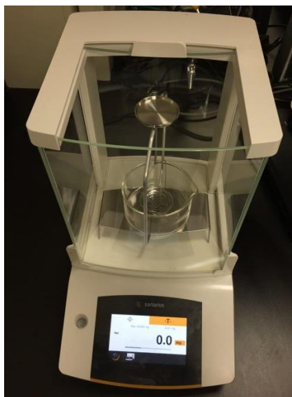
Figure 2-2: Sartorius Density Kit with a hanging basket apparatus used for precisely measuring weight and density.
