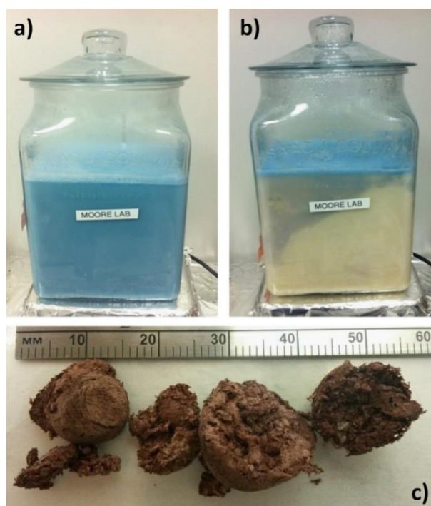
Figure 2-1: The precursor solution a) before and b) after heating on a hot plate at 50 °C with magnetic stirring for 12 hours. The final Cu NW product after freeze-drying is shown in c) with a millimeter scale for reference. Reproduced with permission from Ref. [72].
