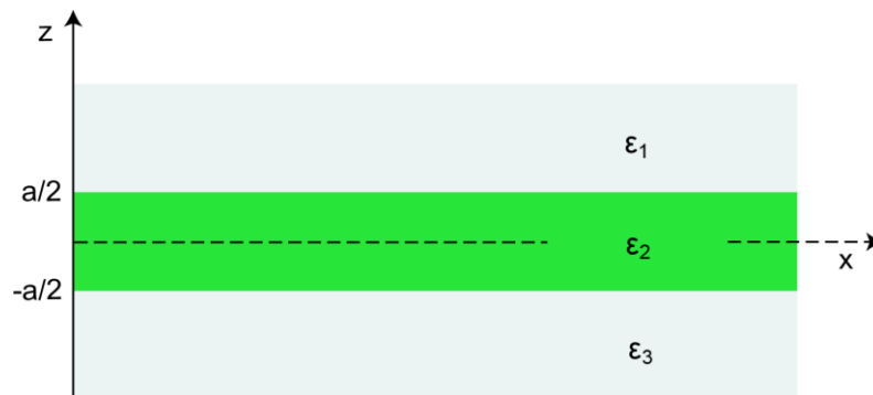
Figure 2-4: Geometry of a three-layer system consisting of a thin layer (2) with permittivity \epsilon_2 is sandwiched between two infinite half spaces (1) and (3).
