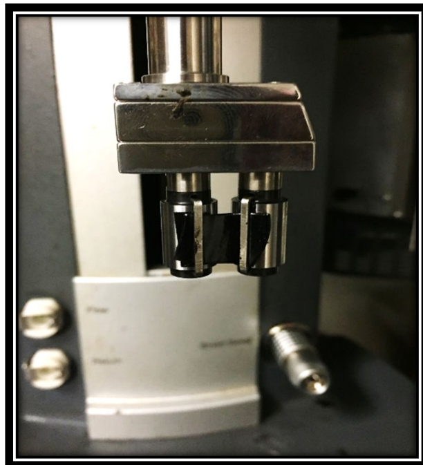
Figure 3-17. SER fixture after loading the sample
