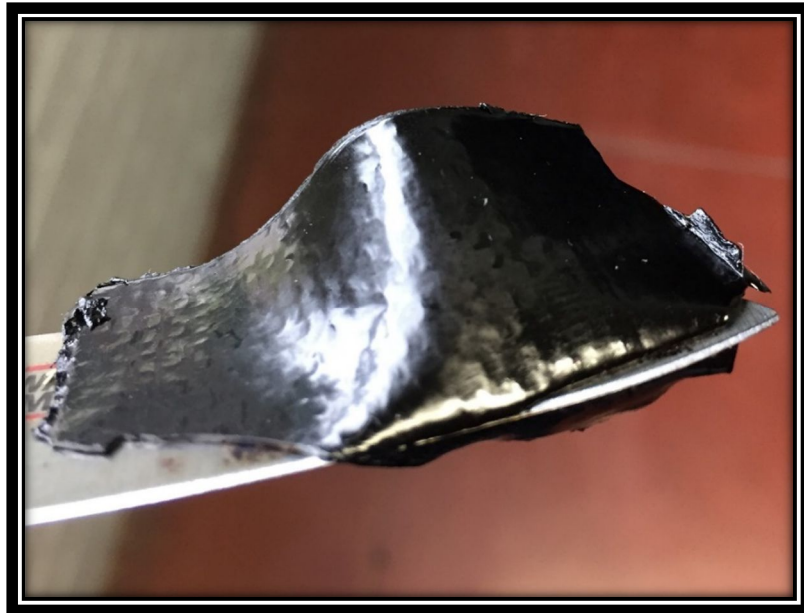
Figure 3-10. Sticking to the metal edge due to a short cooling period
