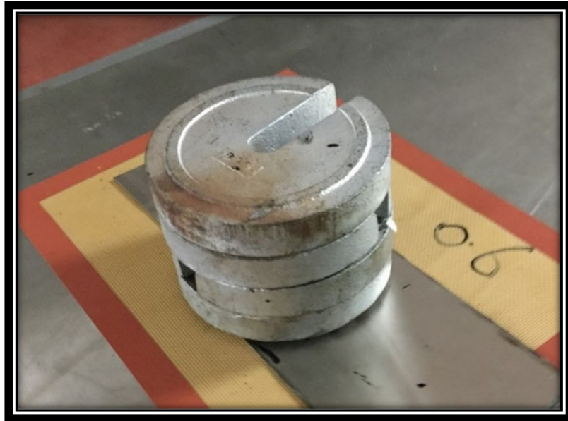
Figure 3-7. The loads placed over the thick glass
