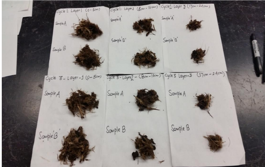
Figure 3.20: Air-drying the root samples (two from each soil layer) collected from wet sieving.
