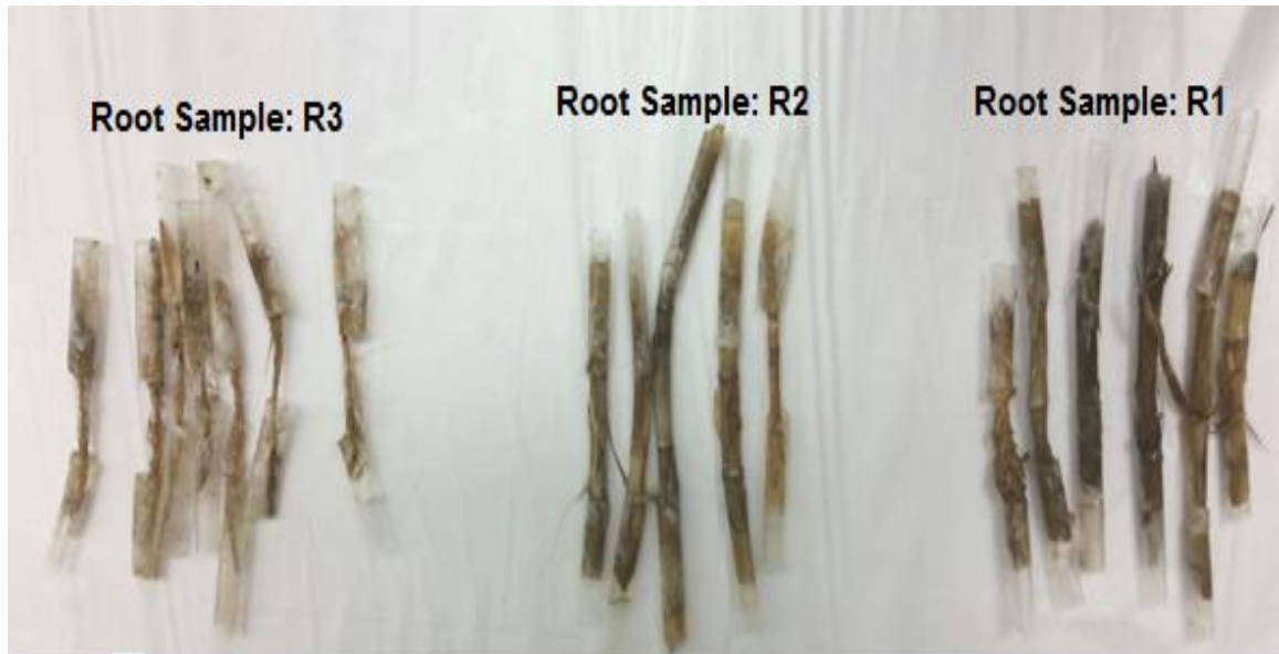
Figure 3.14: Three different root types of Spartina alterniflora showing their ends being prepared for the tensile test.
