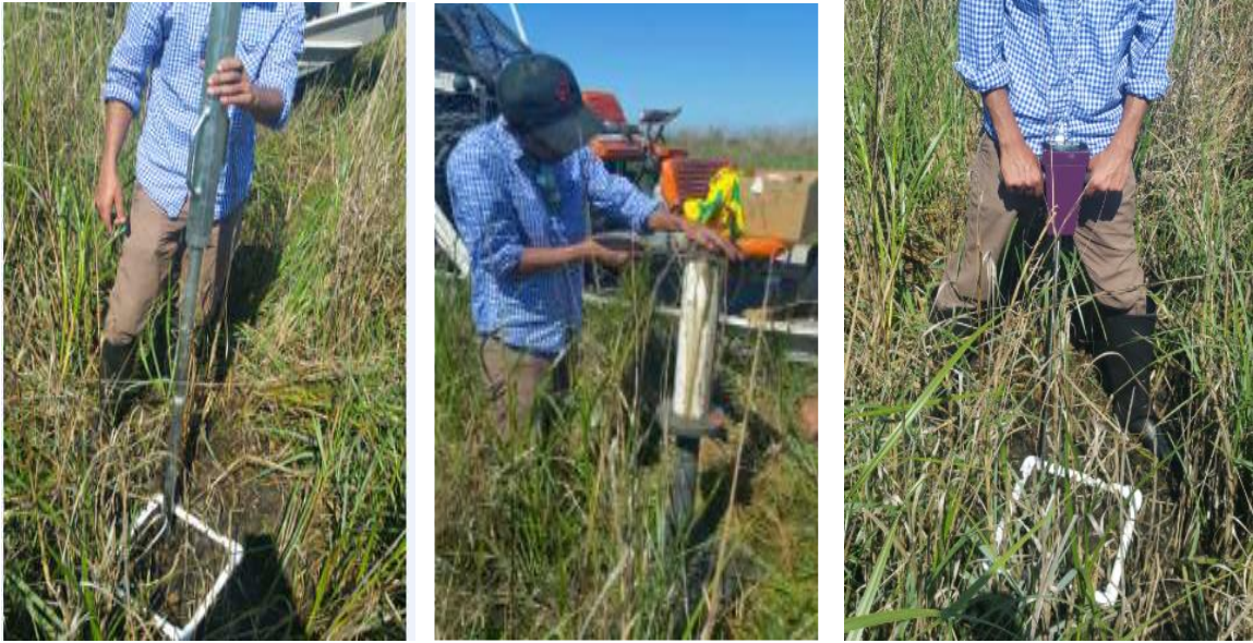
Figure 3.7: (left) Using extruding rod with hammer to get soil samples from Shelby tube from inside the quadrant as seen in picture; (mid) Trimming soil samples at different depths obtained from PVC core sampler; (right) Penetrometer test being conducted on the site.
