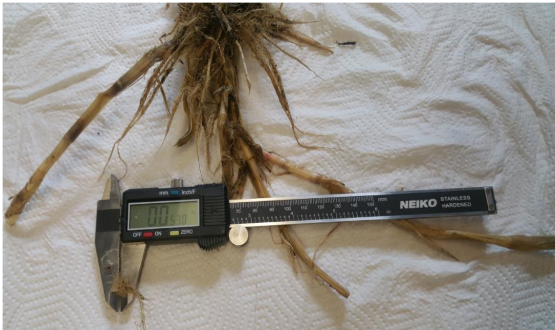
Figure 3.16: Electronic slide caliper used to measure the root diameters of Spartina alterniflora .
