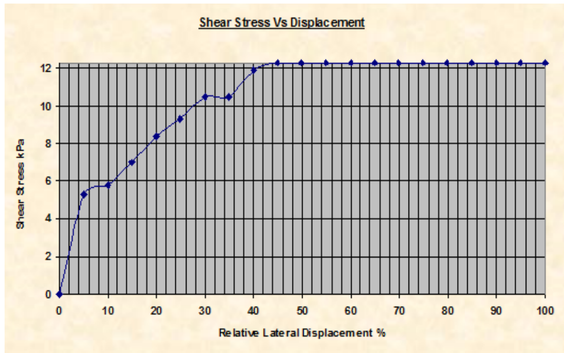
Figure 3.13: A typical shear vs. displacement curve obtained from DS-7 software during the shearing stage of direct shear test.
