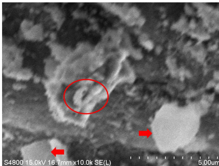
Figure 3-38: SEM imaging of NiFe 1:1 nanofiber catalyst after 15 hours of reaction showing nickel carbides (arrows) and nanofiber clumps (circle).
