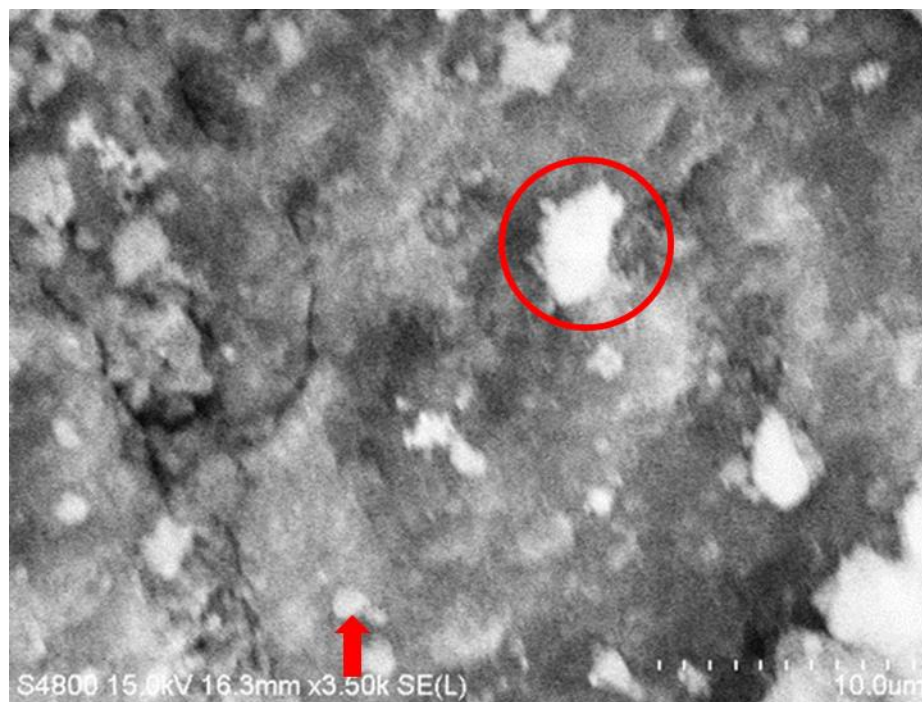
Figure 3-29: SEM image of NiFe nanofiber catalyst 2:1 after 9 hours on stream showing nickel carbides (arrows) and clusters of nanofibers (circle).
